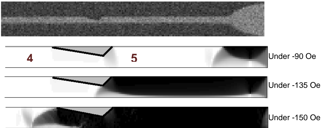
Figure 3.19: (a) Pad simulation showing the cell size and magnetisation direction. (b) The top image is the scanning electron microscopy (SEM) image of sample 14 and then the simulation results of sample 14 showing domain wall motion before the notch.
