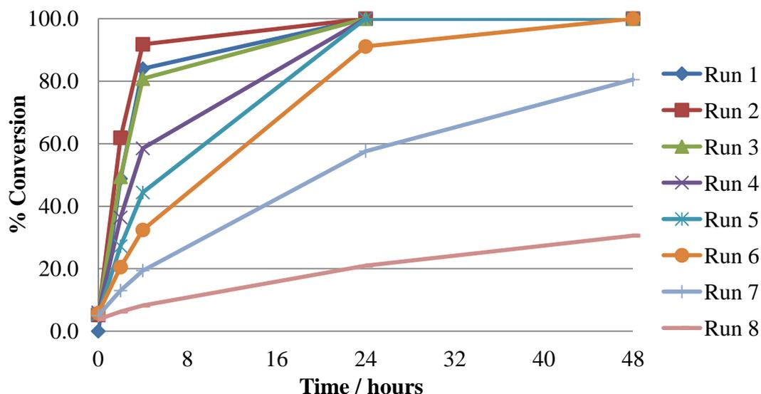
**Chart 7.9** Reuse data for the reduction of benzaldehyde by catalyst **7.12** via **Scheme 7.5**
