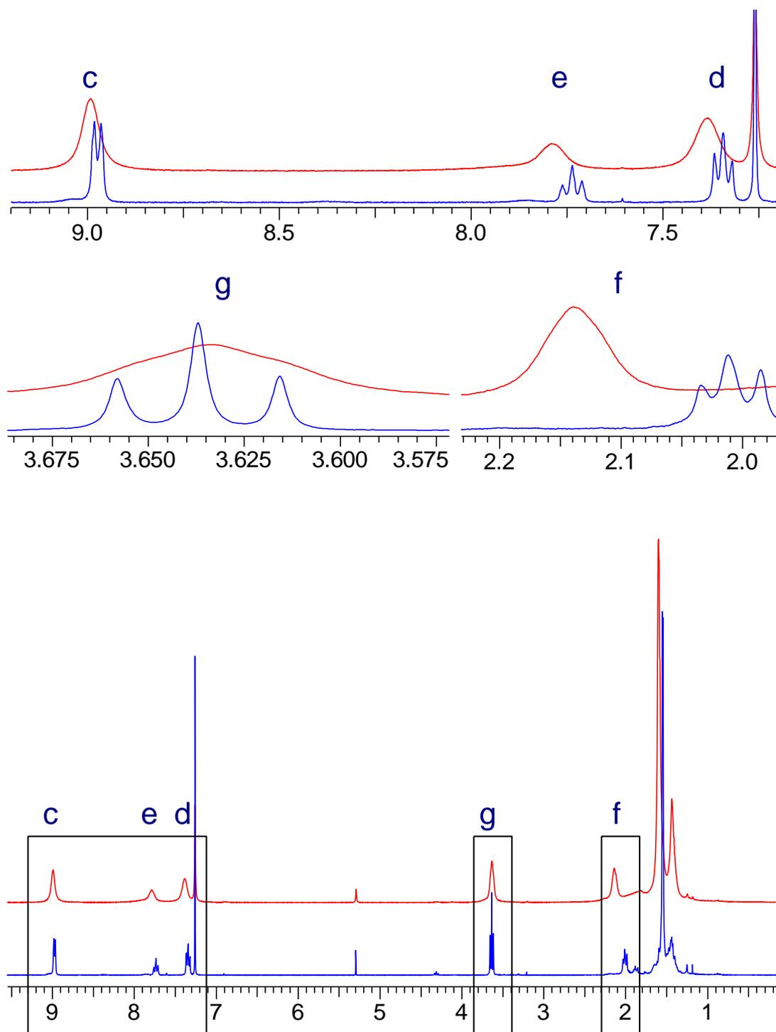
**Figure 3.17** Comparison of the  $^1\text{H}$  NMR spectra of iridium and rhodium tethered pyridine complexes **3.8** and **3.15**
