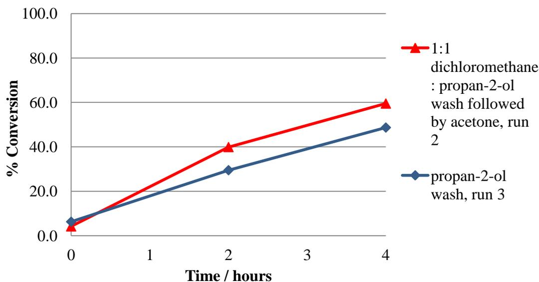
**Chart 7.5** A graph to highlight the improved catalytic activity of catalyst **7.10** for the reduction of benzaldehyde *via* **Scheme 7.5**, with a new washing regime
