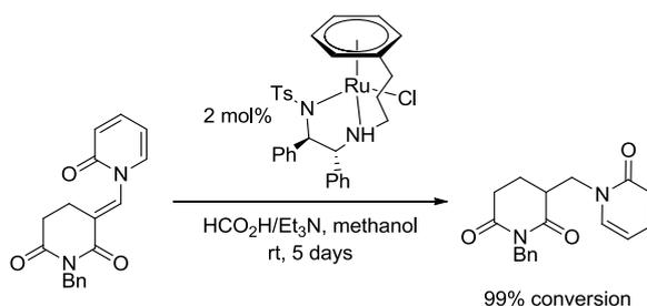
**Scheme 1.44** Reduction of an alkene bond, by a tethered ruthenium catalyst to form an N-benzyl-(3-aminomethylglutarimide) derivative
