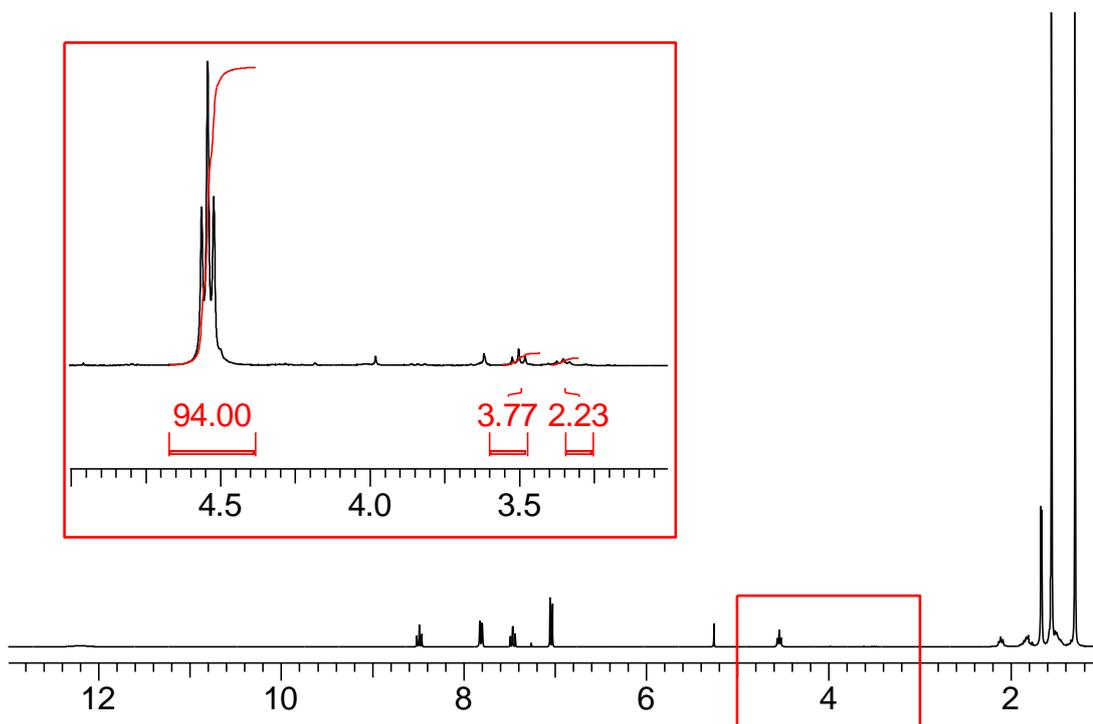
**Figure 7.3**  $^1\text{H}$  NMR spectrum of the *in situ* triflate intermediate **7.4**, showing 94% conversion to the triflate *cf.* secondary products
