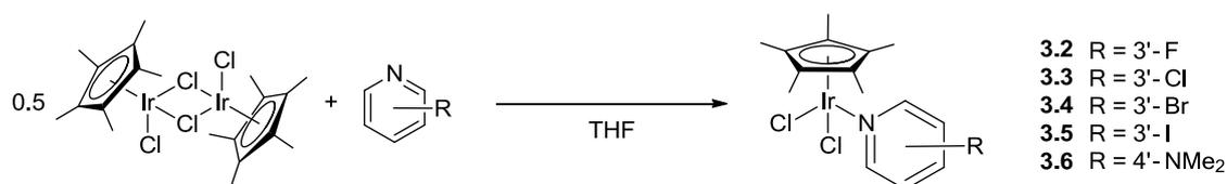
**Scheme 3.1** General synthesis of iridium Cp\* dichloride pyridine complexes
