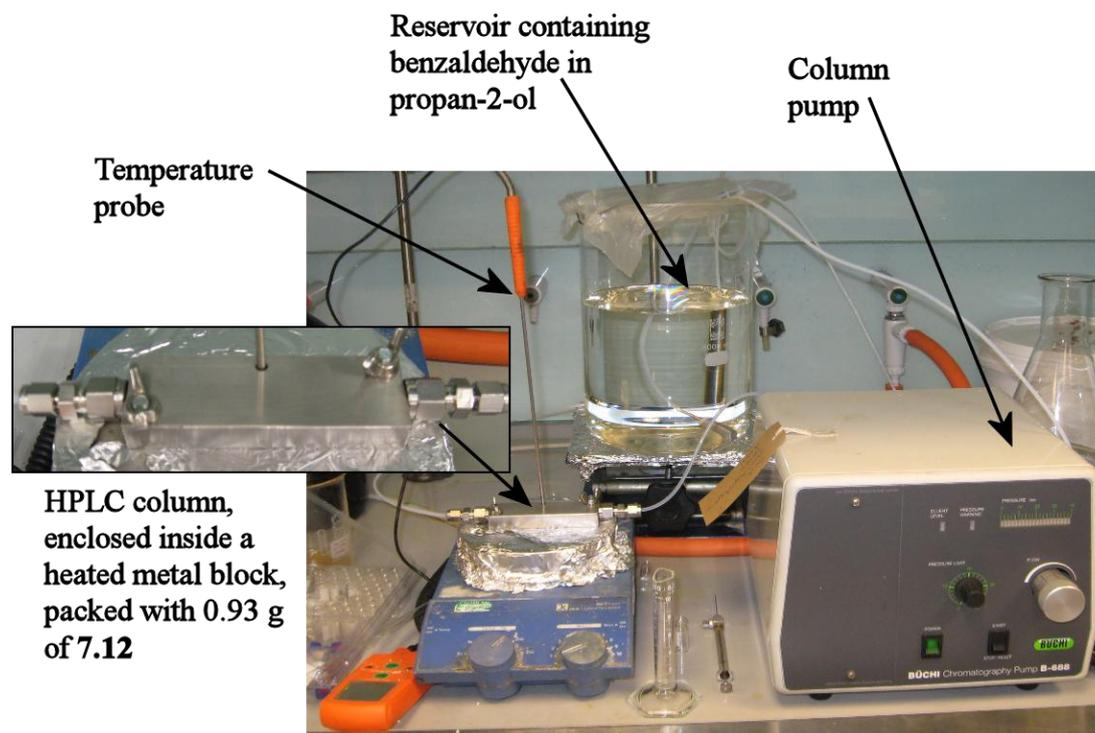
**Figure 7.8** Flow apparatus used for the reduction of benzaldehyde by catalyst 7.12
