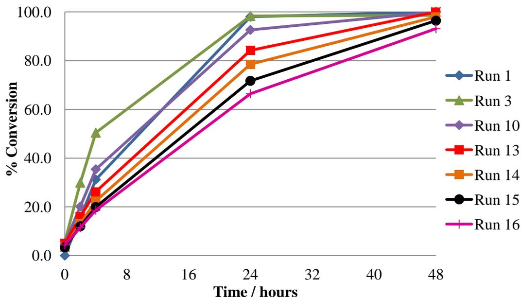
**Chart 7.6** Reuse data for the reduction of benzaldehyde by catalyst **7.10** via **Scheme 7.5**
