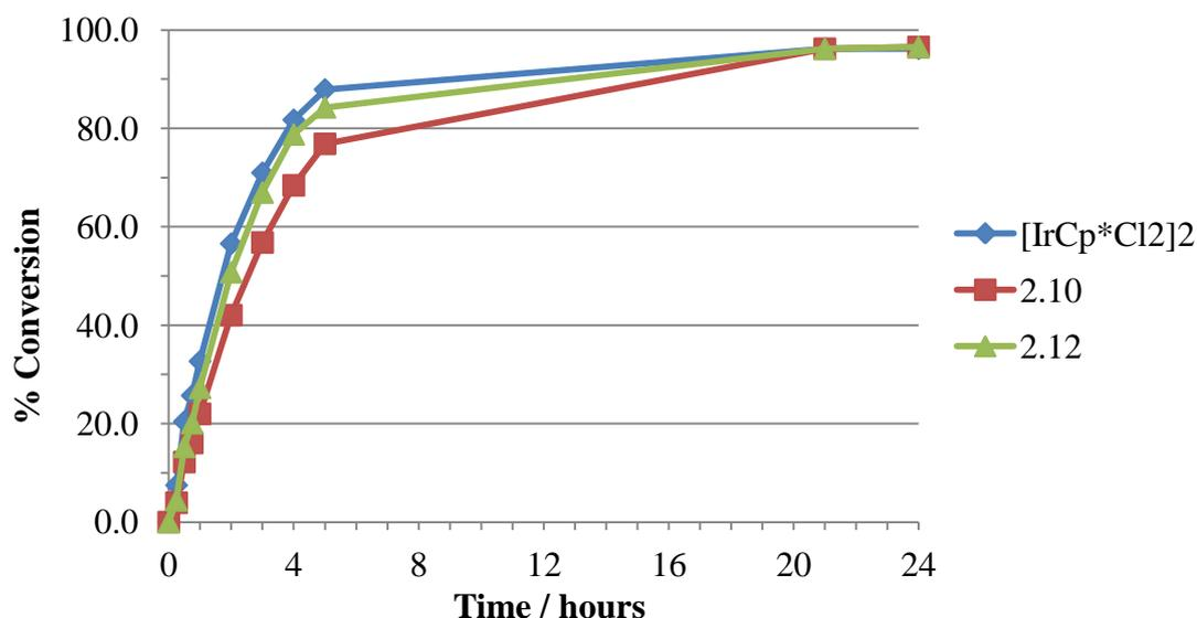
**Chart 6.3** Catalytic reduction of acetophenone using hydroxyl tethered Cp\* based iridium chloride dimers
