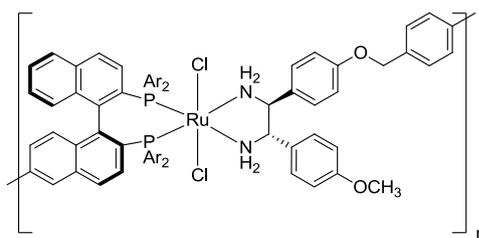
**Figure 1.26** A ruthenium MOF used for the enantioselective hydrogenation of ketones
