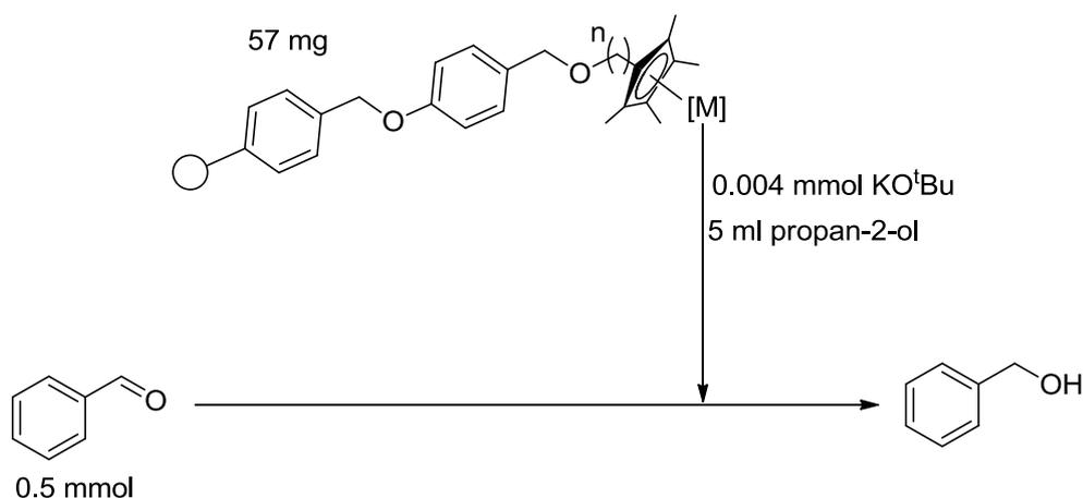
**Scheme 7.5** General scheme for catalytic reduction of benzaldehyde with immobilised complexes
