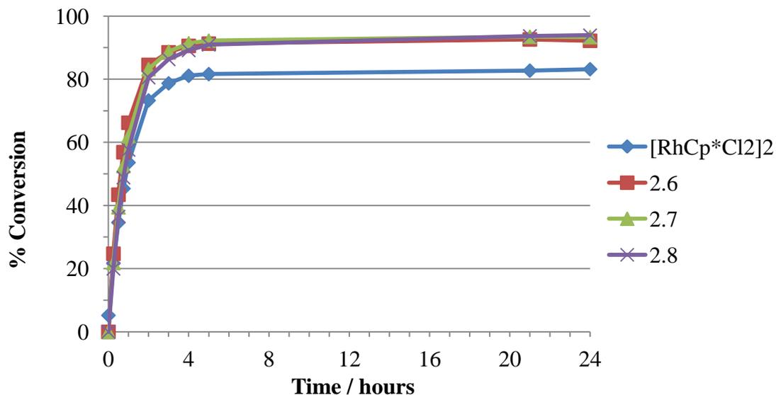
**Chart 6.4** Catalytic reduction of acetophenone using hydroxyl tethered Cp\* based rhodium chloride dimers
