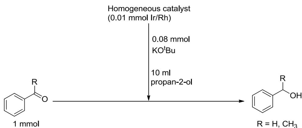
**Scheme 6.1** General scheme for catalytic reduction of benzaldehyde with homogeneous complexes
