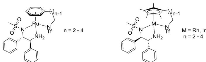
**Figure 1.14** Triflylamide tethered Noyori-type catalysts
