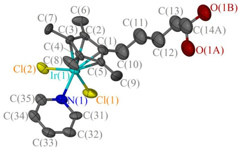
**Figure 3.13** A crystal structure of compound **3.8**, displacement ellipsoids are at the 50% probability level. Hydrogen atoms are omitted for clarity
