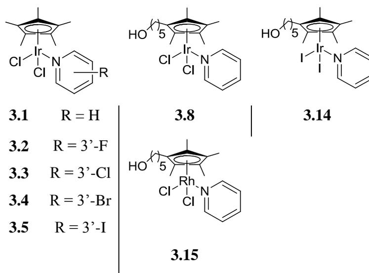
**Figure 6.2** List of hydroxyl tethered Cp\* based group 9 halide pyridine complexes used as homogeneous catalysts in this Chapter
