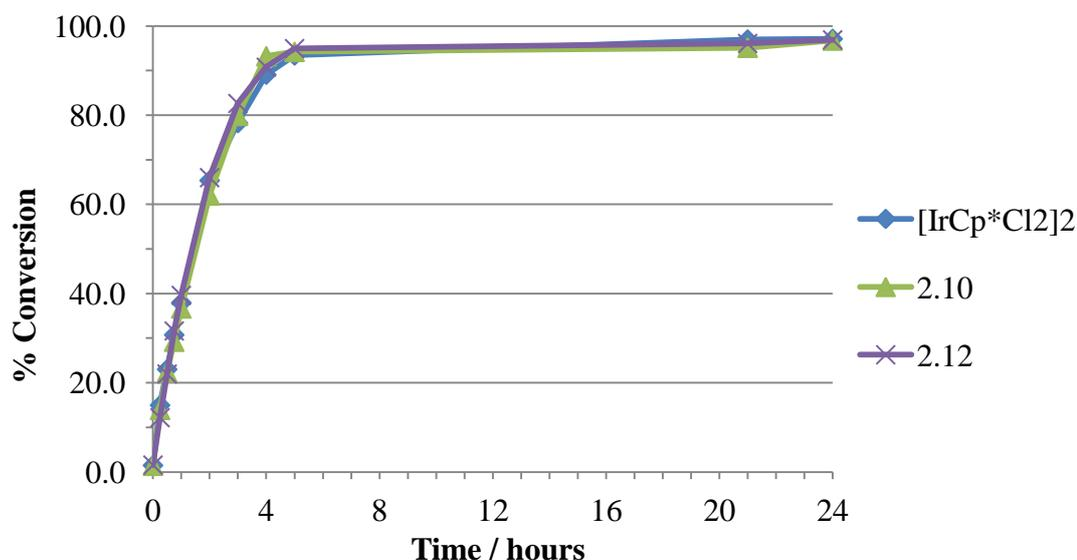
**Chart 6.1** Catalytic reduction of benzaldehyde using hydroxyl tethered Cp\* based iridium chloride dimers
