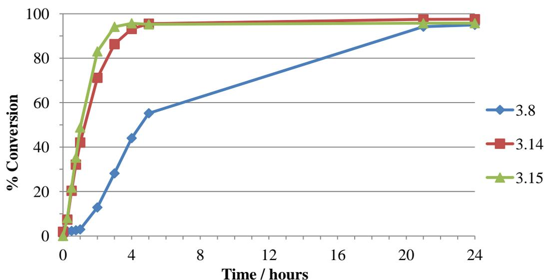
**Chart 6.6** Catalytic reduction of benzaldehyde using hydroxyl tethered Cp\* based pyridine complexes **3.8**, **3.14** and **3.15**
