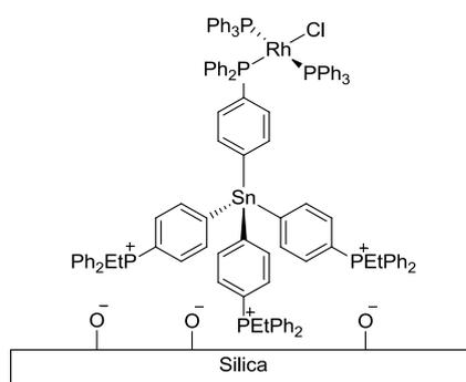
**Figure 1.25** Immobilised Wilkinson-type catalyst, through coordinative bonding and electrostatic interactions
