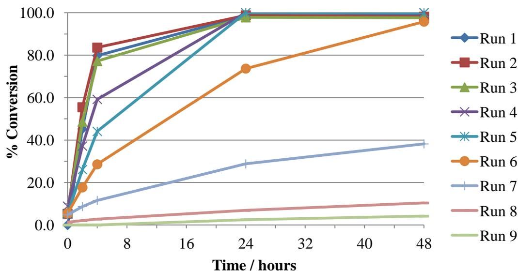
**Chart 7.8** Reuse data for the reduction of benzaldehyde by catalyst **7.11** via **Scheme 7.5**
