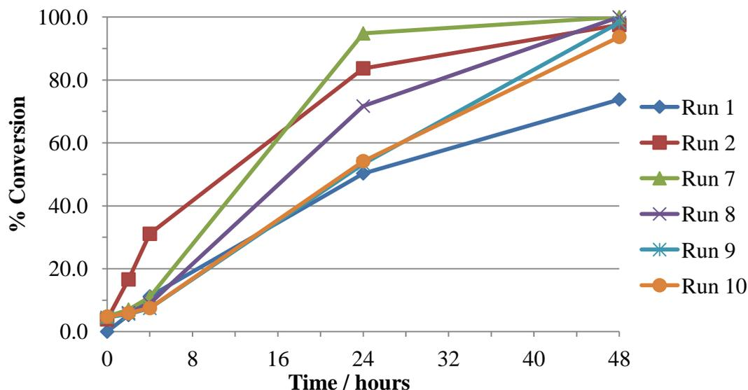
**Chart 7.11** Reuse data for the reduction of benzaldehyde by catalyst **7.8** via **Scheme 7.5**
