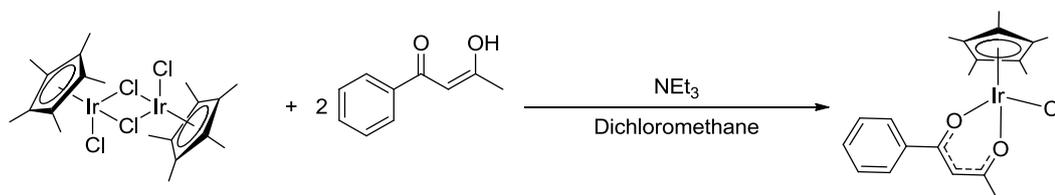
**Scheme 5.3** Synthesis of the iridium Cp\* chloride diketonate complex, **5.4**
