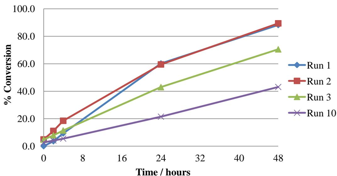
**Chart 7.10** Reuse data for the reduction of benzaldehyde by catalyst **7.7** via **Scheme 7.5**
