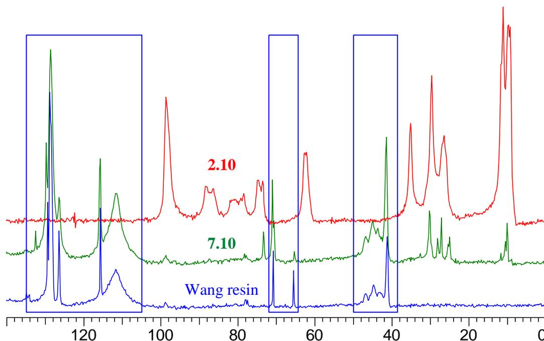
**Figure 7.7** Solid state  $^{13}\text{C}\{^1\text{H}\}$ NMR of the immobilised complex **7.10**, along with the functionalised dimer **2.10** and polystyrene supported Wang resin for reference. The blue boxes highlight the peaks due to the resin
