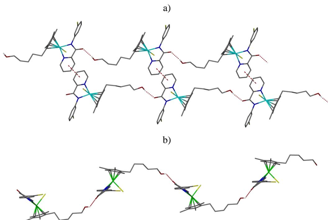
**Figure 1.8** Packing diagrams of compounds **a) 4.15**, and **b) 4.19** showing intermolecular hydrogen bonds and  $\pi$ - $\pi$  stacking. Hydrogen atoms (apart from the hydroxyl) are omitted for clarity
