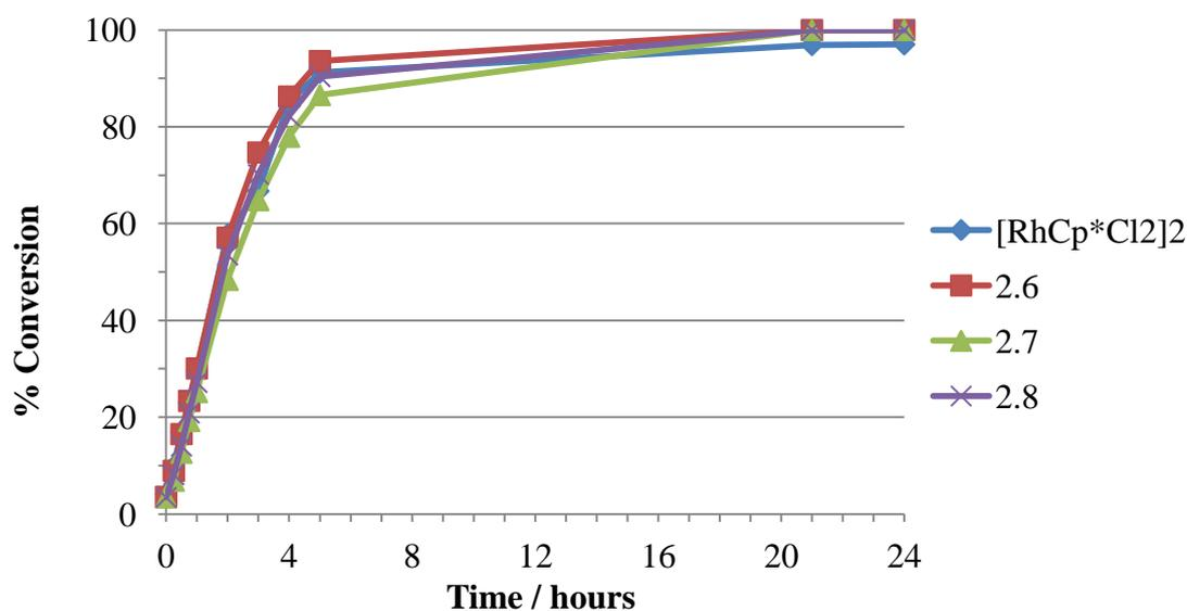
**Chart 6.2** Catalytic reduction of benzaldehyde using hydroxyl tethered  $\text{Cp}^*$  based rhodium chloride dimers
