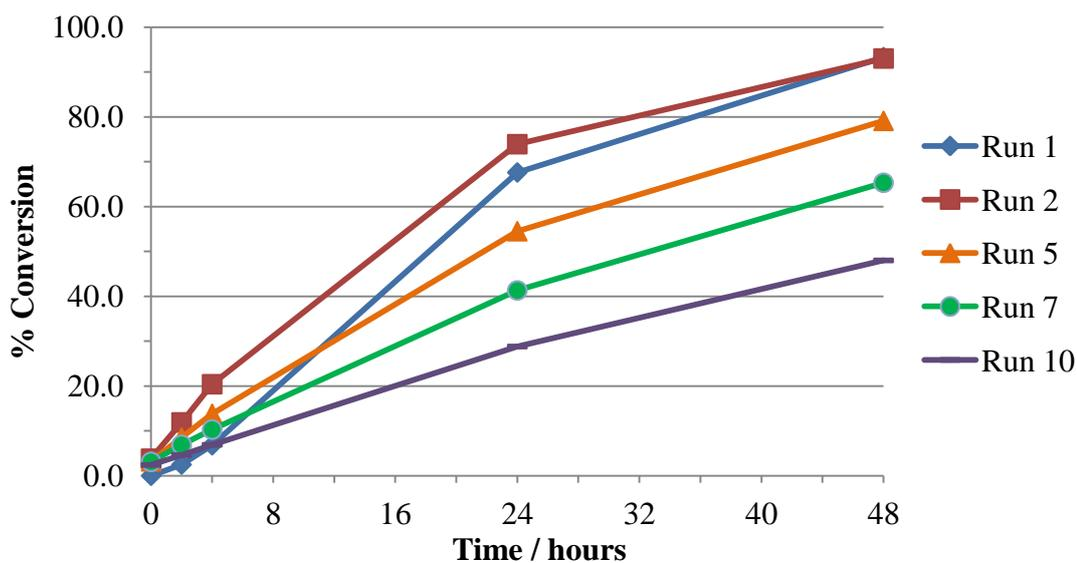
**Chart 7.17** Reuse data for the reduction of acetophenone by catalyst **7.12** via **Scheme 7.5****Scheme 6.1**
