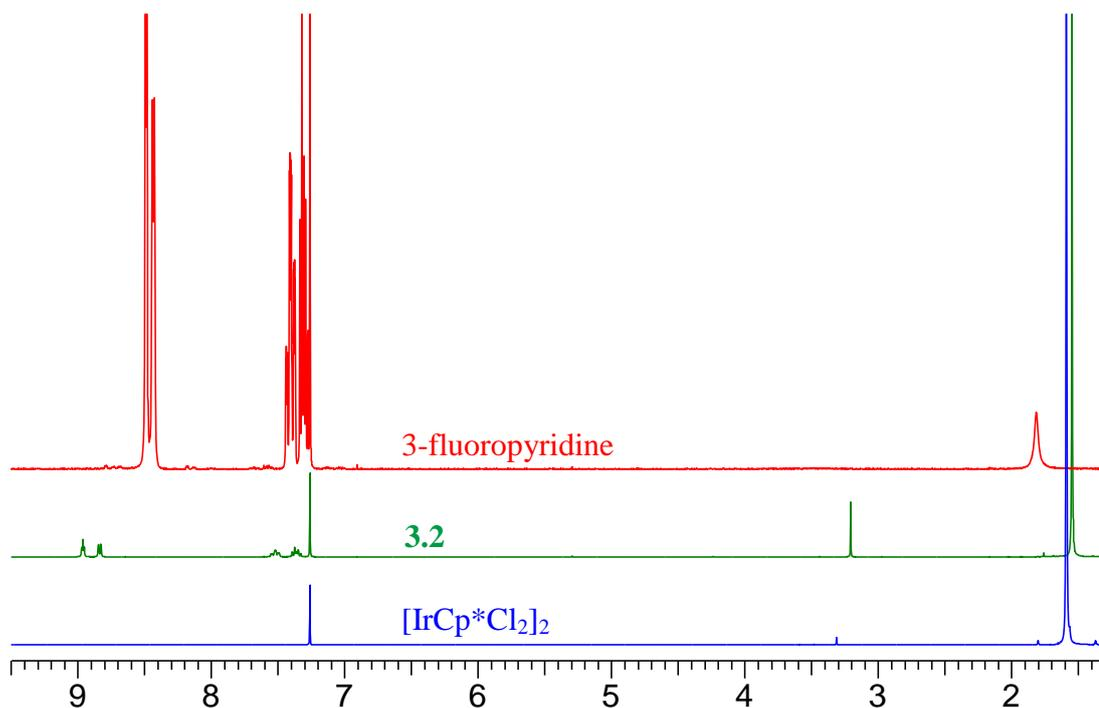
**Figure 3.3** Comparison of the  $^1\text{H}$  NMR spectra of compound **3.2** compared to its precursors,  $[\text{IrCp}^*\text{Cl}_2]_2$  and 3-fluoropyridine
