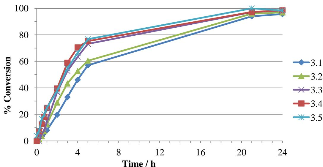
**Chart 6.5** Catalytic reduction of benzaldehyde using iridium Cp\* dichloride pyridine complexes
