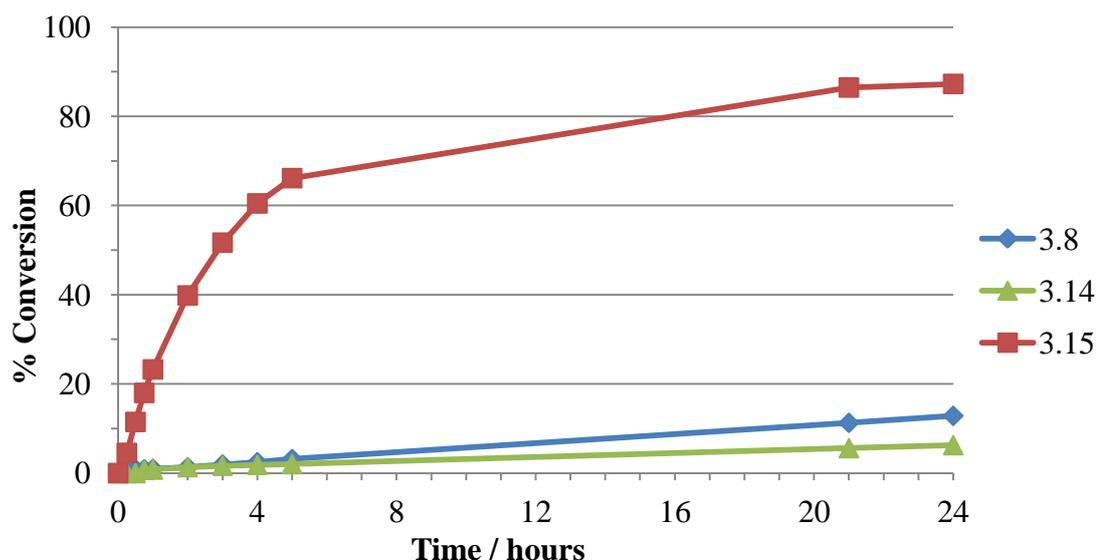
**Chart 6.8** Catalytic reduction of acetophenone using hydroxyl tethered Cp\* based pyridine complexes **3.8**, **3.14** and **3.15**
