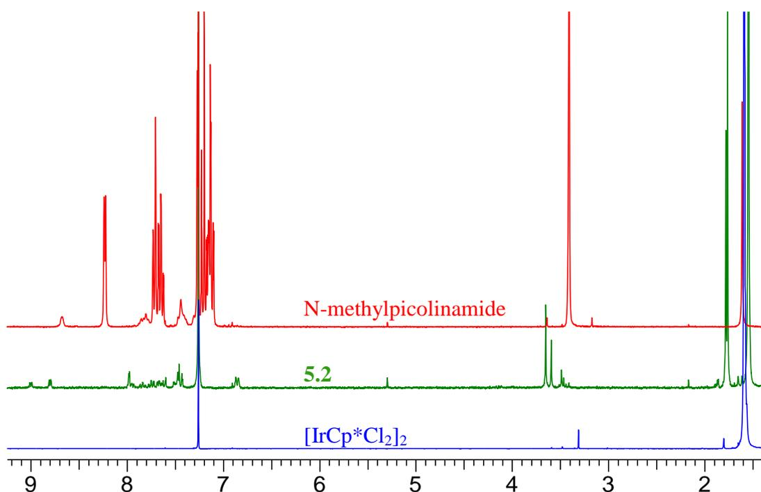
**Figure 5.4** <sup>1</sup>H NMR spectrum of compound **5.2** compared to its constituent starting materials
