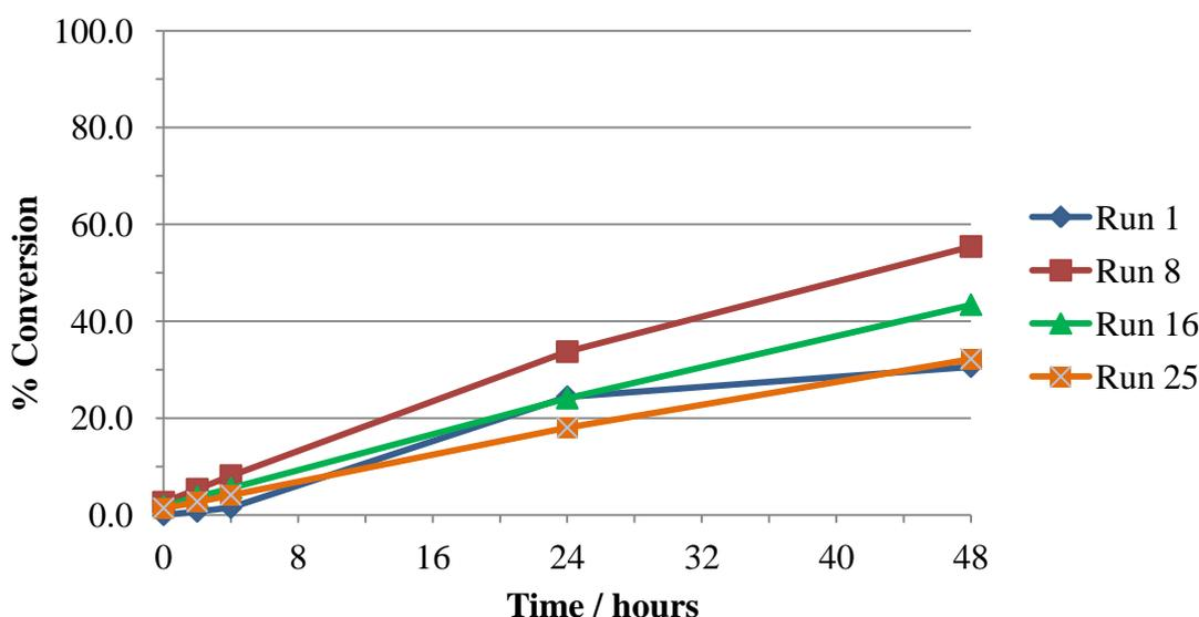
**Chart 7.16** Reuse data for the reduction of acetophenone by catalyst **7.10** via Scheme 7.5
