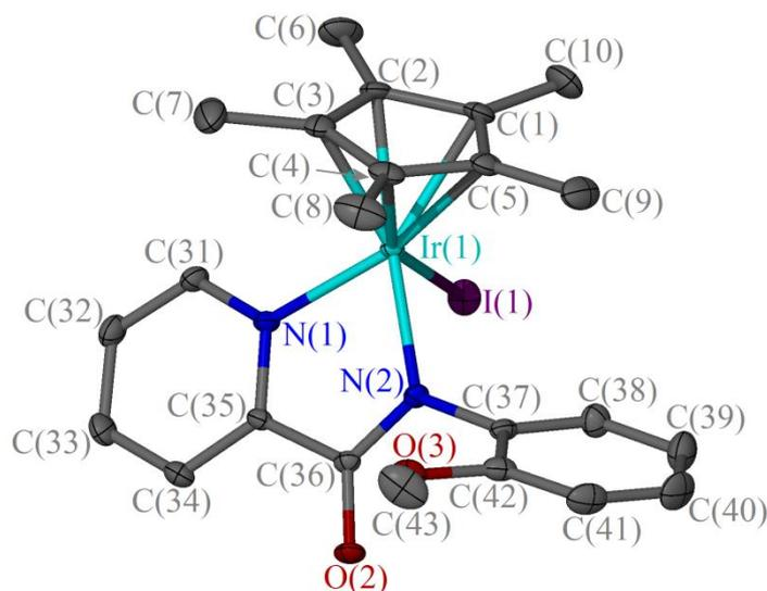
**Figure 1.17** A crystal structure of compound **4.14**, displacement ellipsoids are at the 50% probability level. Sodium iodide, methanol, dichloromethane, water and hydrogen atoms are omitted for clarity
