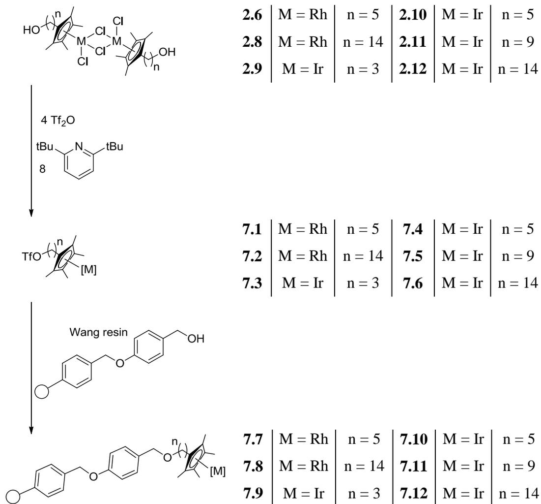
**Scheme 7.1** Immobilisation of hydroxyl tethered Cp\* based metal halide complexes onto polystyrene supported Wang resin
