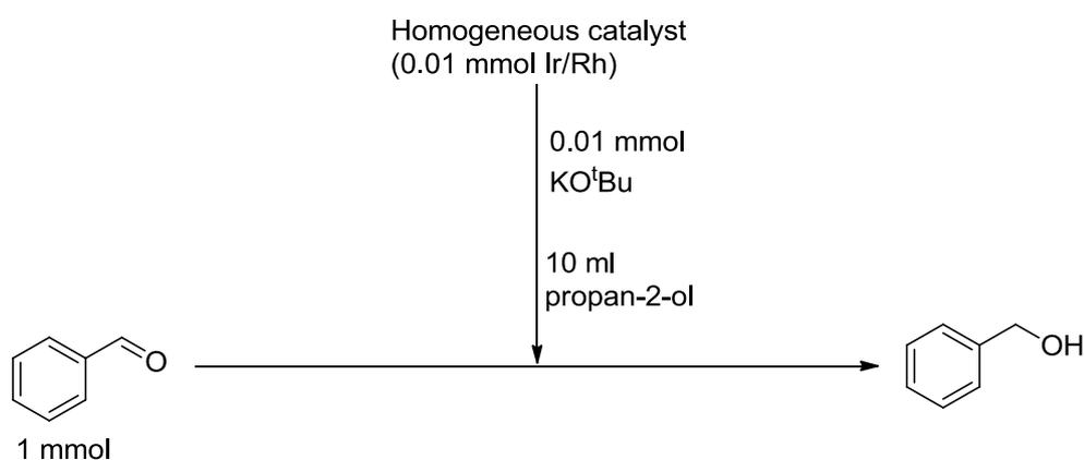
**Scheme 7.3** General scheme for catalytic reduction of benzaldehyde with homogeneous complexes
