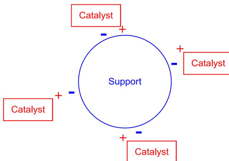
**Figure 1.23** General design of an electrostatically immobilised catalyst
