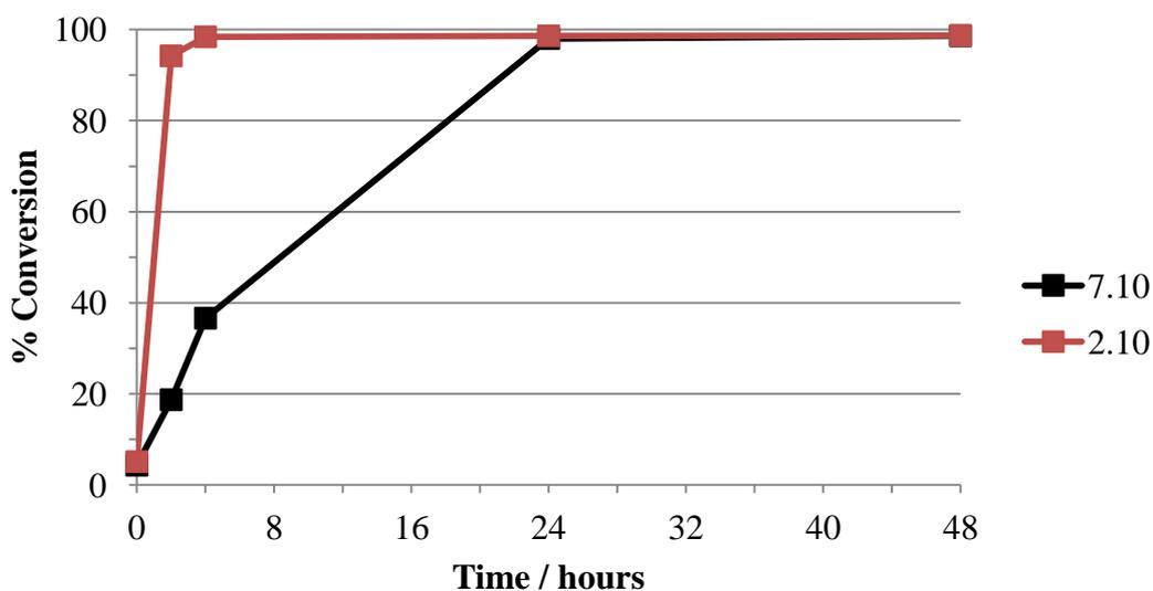
**Chart 7.2** Catalytic activity of the immobilised complex **7.10** compared to the homogeneous analogue **2.10** (1 mol% homogeneous catalyst)
