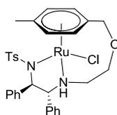
**Figure 1.10** Oxo-tethered Noyori-type catalyst
