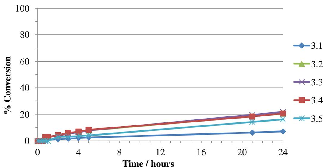
**Chart 6.7** Catalytic reduction of acetophenone using iridium Cp\* dichloride pyridine complexes
