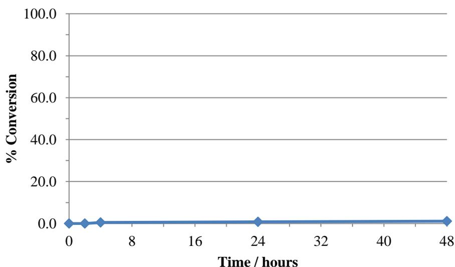
**Chart 7.19** Resin formed from control reaction two as a catalyst for the reduction of benzaldehyde *via* **Scheme 7.5**
