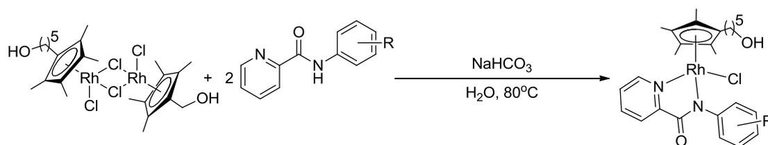
**Scheme 1.5** Synthesis of rhodium hydroxyl tethered Cp\* based chloride picolinamide complexes **4.18** and **4.19**
