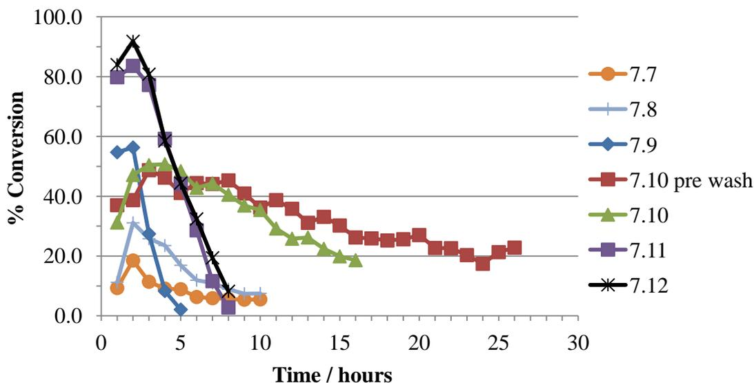
**Chart 7.12** Comparison of the recyclability of the immobilised complexes from the conversion of benzaldehyde to benzyl alcohol at four hours
