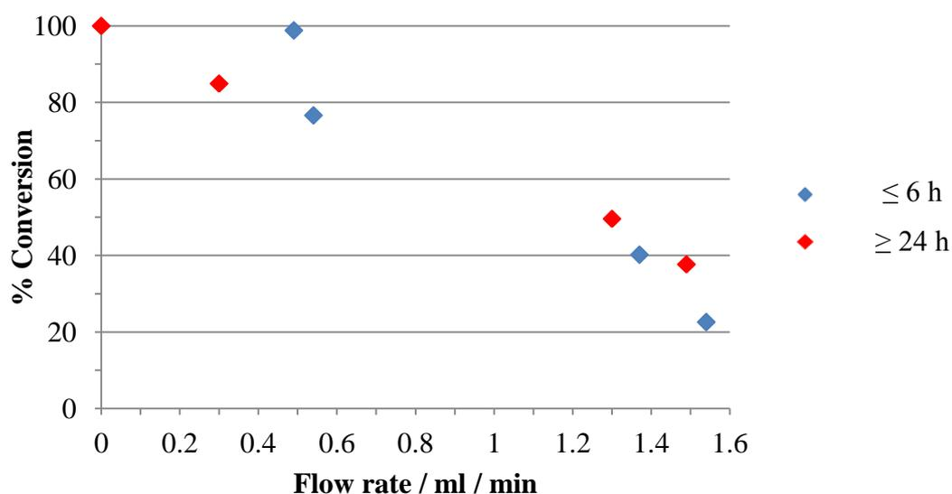
**Chart 7.15** Run two-Conversion of benzaldehyde to benzyl alcohol against the flow rate
