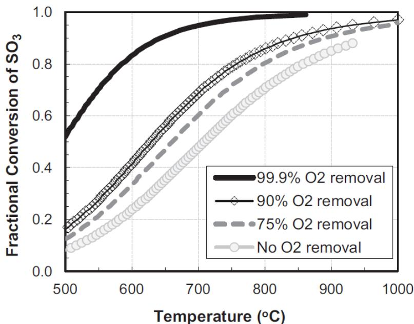
Figure 1.2: Effect of  $O_2$  removal on the fractional conversion of  $SO_3$  to  $SO_2$  as a function of temperature (Mawdsley et al. 2012)
