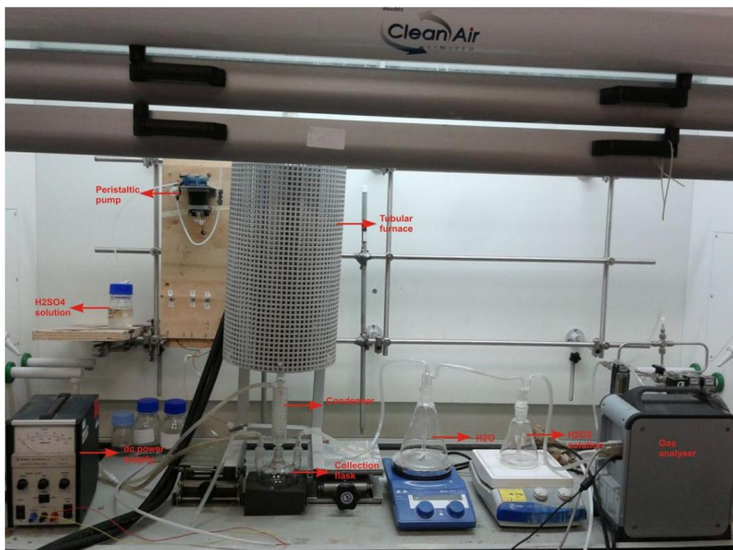
Figure 6.3: Fully instrumental straight-through peristaltic pump, catalytic decomposer, condenser, products collection and separation system.
