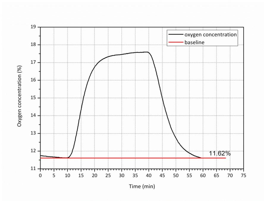
Figure 6.11: Oxygen concentration change with time in  $H_2SO_4$  thermal decomposition (Section II)
