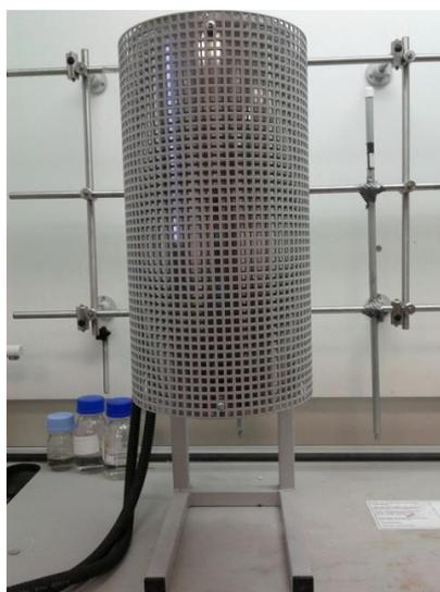
Figure 6.5: Tubular furnace in a fume hood
