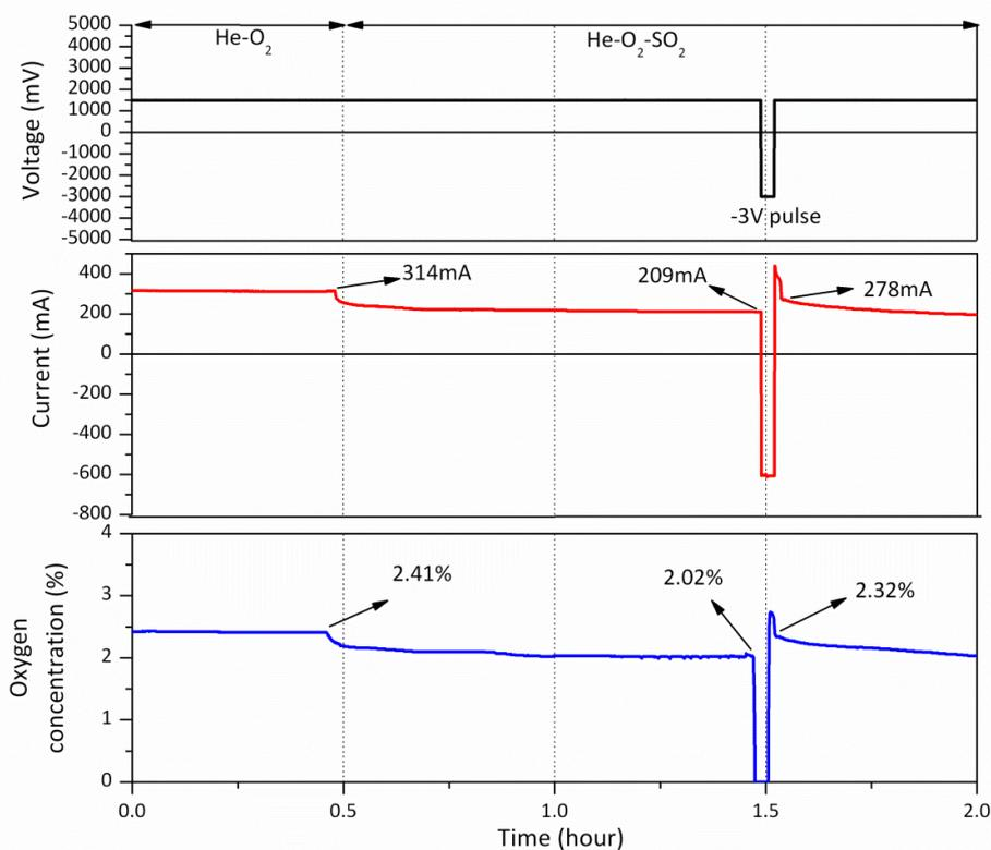
Figure 4.10: Experimental data for YSZ/Pt pellet exposure to  $\text{SO}_2$  and  $\text{O}_2$  at  $850^\circ\text{C}$  with a 2-minute 3V negative pulse treatment
