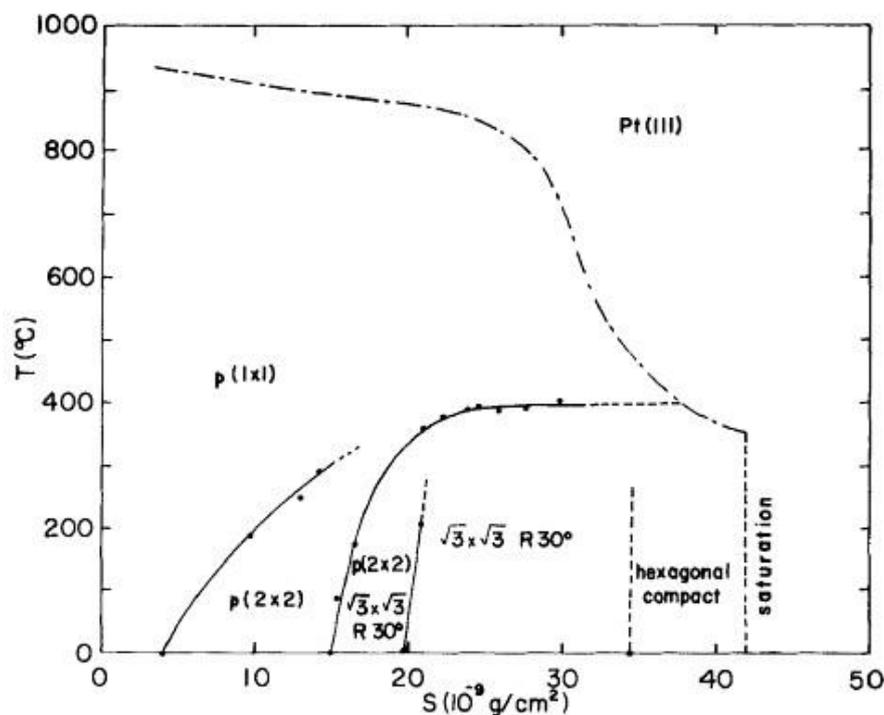
Figure 4.25: Surface structures of sulphur on Pt (111) as a function of coverage and temperature (Bartholomew et al. 1982)
