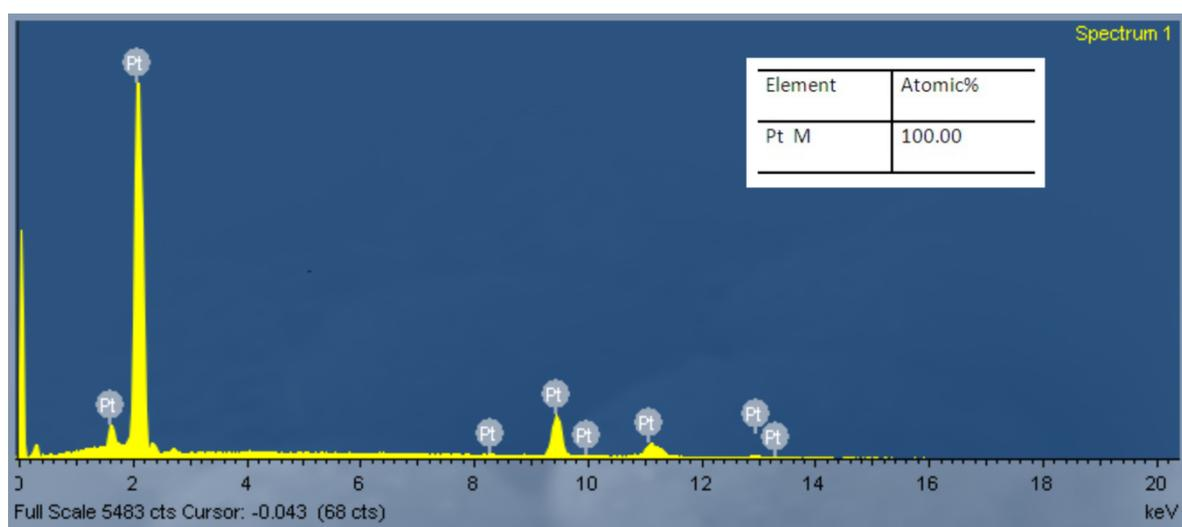
Figure 3.17: EDS elemental analysis spectrum of a fresh Pt/8YSZ pellet
