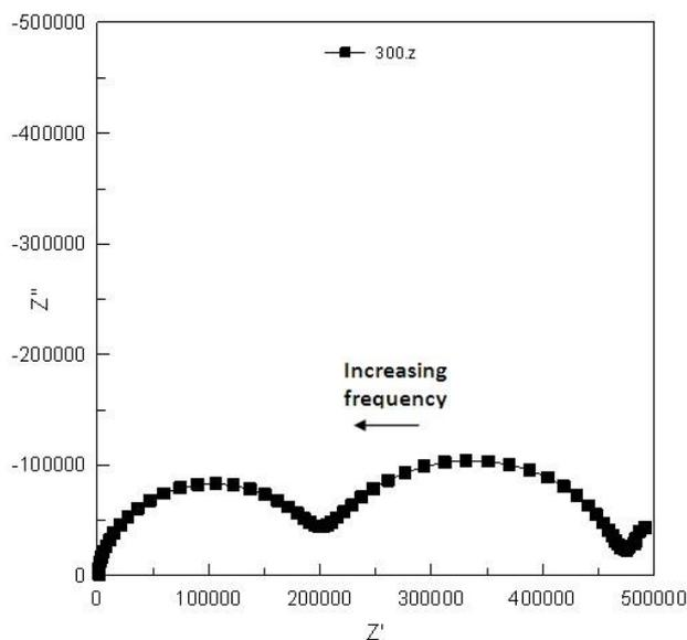
Figure 3.3:  $Z''$  plot for the Pt/8YSZ/Pt pellet at 300°C, full frequency range of 5Hz - 1.3MHz is shown.
