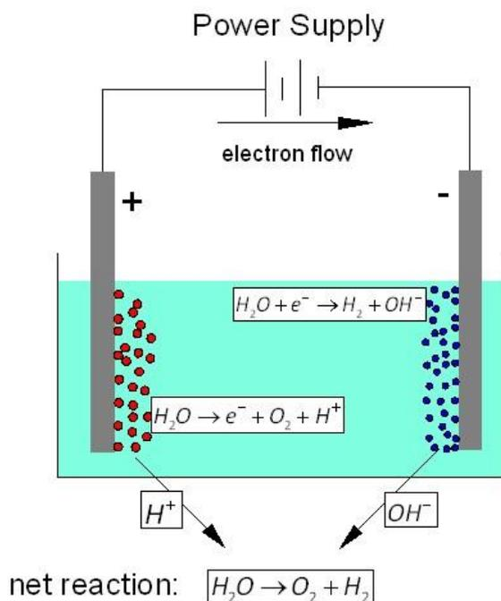
Figure 2.5: Schematic of water electrolysis process
