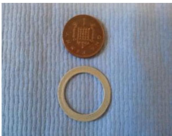
Figure 5.13: A *Thermoculite 866 ring gasket*
