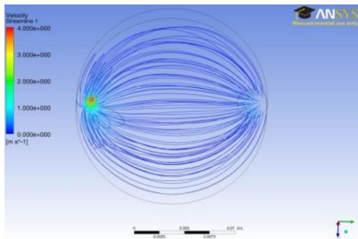
Figure 5.28: Velocity streamline of gas flowing through all domains (top view)
