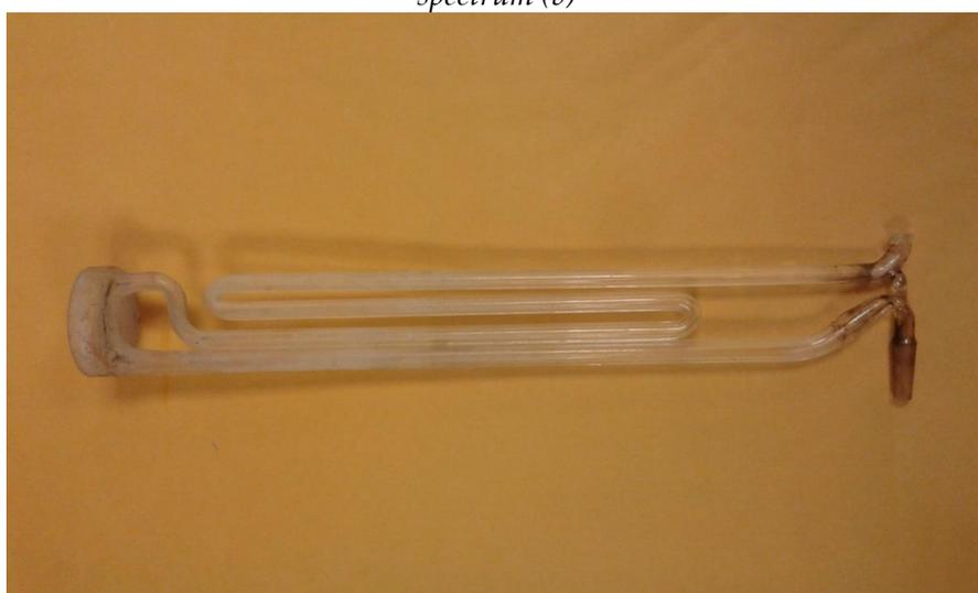
Figure 3.21: Membrane holder after  $\text{SO}_2$  exposure test at  $850^\circ\text{C}$
