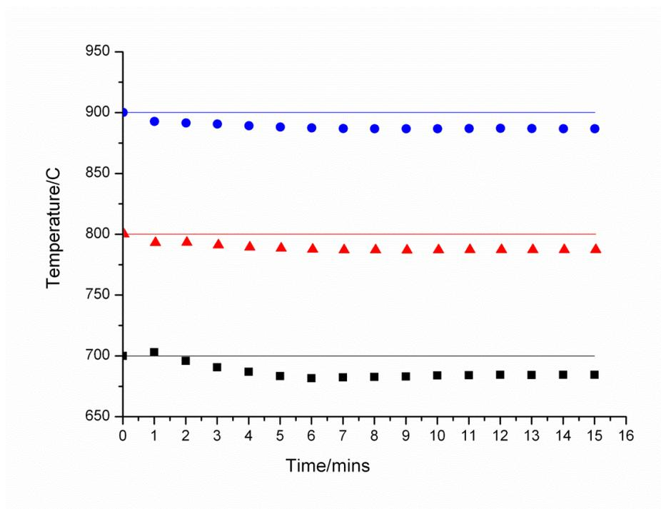
Figure 3.6: Difference of the furnace setpoint and the real temperature at 700, 800 and 900°C
