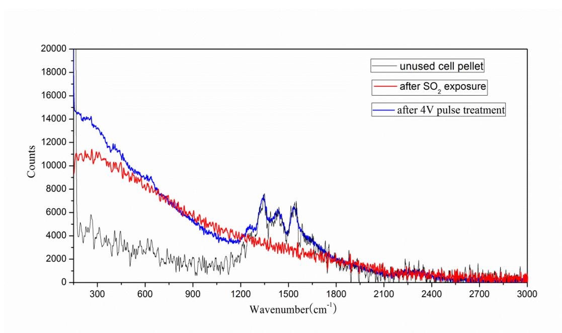
Figure 4.4: Raman spectra of cathode surface for YSZ/Pt pellet after 4V pulse treatment
