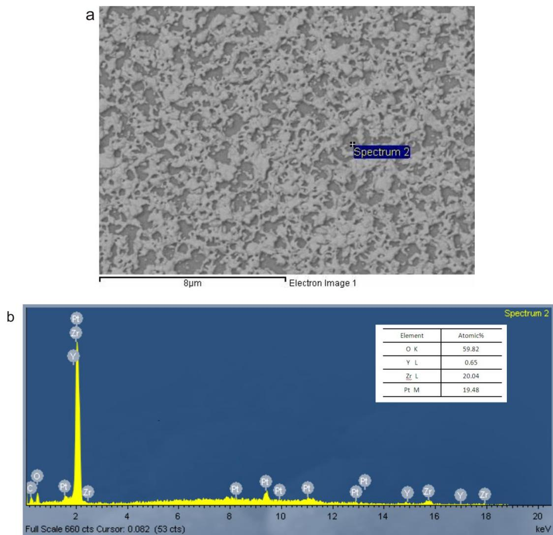
Figure 3.18: EDS element point analysis for fresh pellet: SEM image (a) and EDS spectrum (b)
