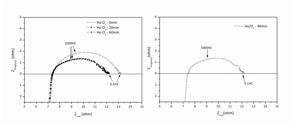
Figure 4.19: Impedance spectra of Pt/8YSZ/Pt cell recorded in  $SO_2$  free period (Group A), at  $850^\circ C$
