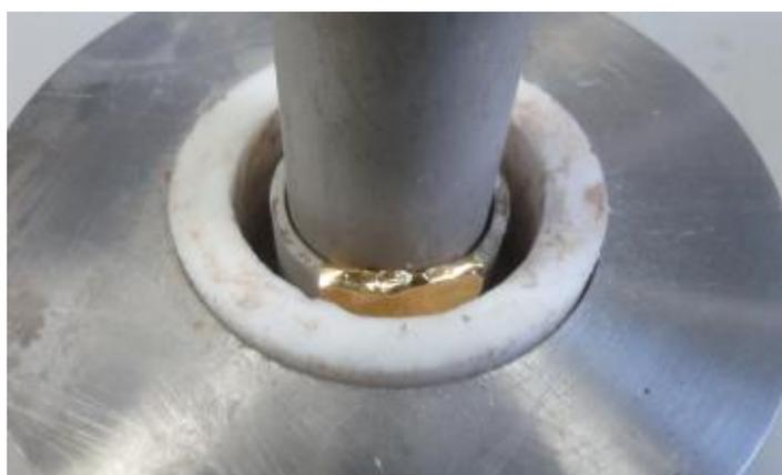
Figure 5.11: *Electrical connection of tube outer electrode surface to power supply*
