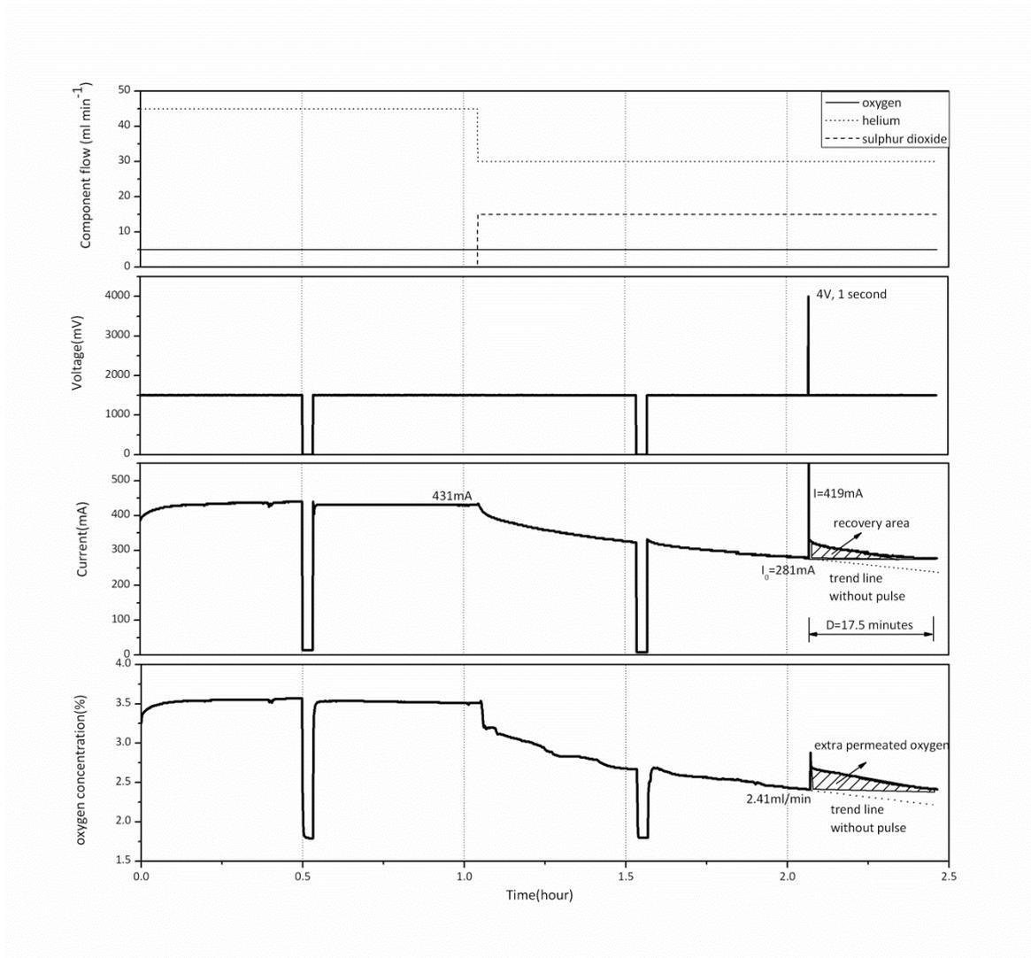
Figure 4.26: *Pt/8YSZ/Pt* performance degradation and recovery at  $850^\circ\text{C}$ , the cathode exposed to  $\text{He-O}_2\text{-SO}_2$  and the anode exposed to  $\text{He}$ .
