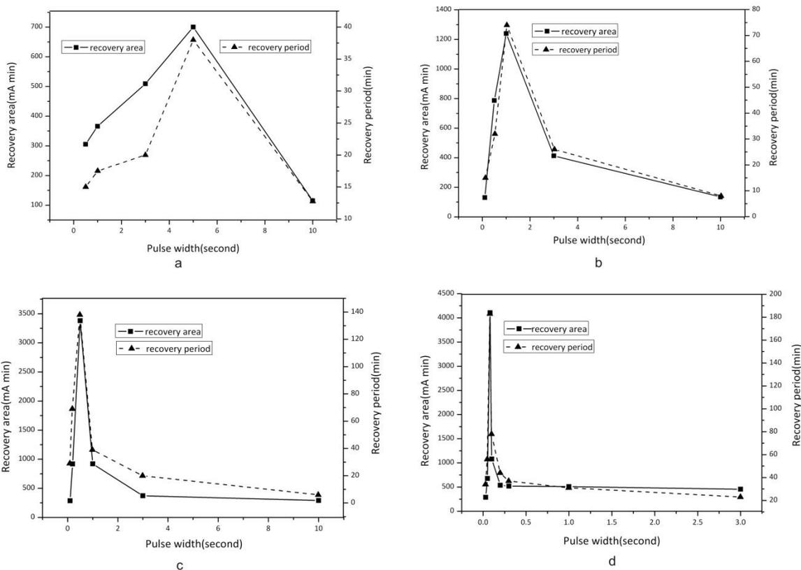
Figure 4.27: Cell performance recovery period and recovery area after pulse treatment, a) 4V pulse with 0.5, 1, 3, 5 and 10 seconds; b) 6V pulse with 0.1, 0.5, 1, 3 and 10 seconds; c) 7V pulse with 0.1, 0.2, 0.5, 1, 3 and 10 seconds; d) 10V pulse with 0.03, 0.05, 0.08, 0.1, 0.2, 0.5, 1 and 3 seconds
