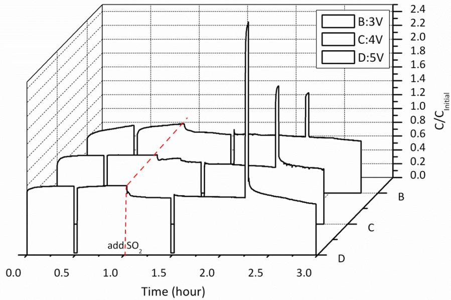
Figure 4.12: Performance change after current normalization of Pt/8YSZ/Pt membrane pellet exposed to  $\text{SO}_2\text{-O}_2$  at  $850^\circ\text{C}$ , with different positive voltage pulses
