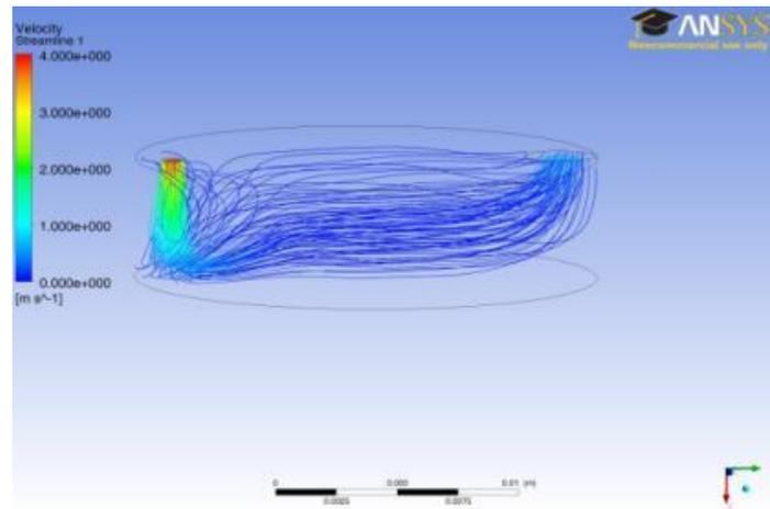
Figure 5.27: Velocity streamline of gas flowing through all domains (front view)
