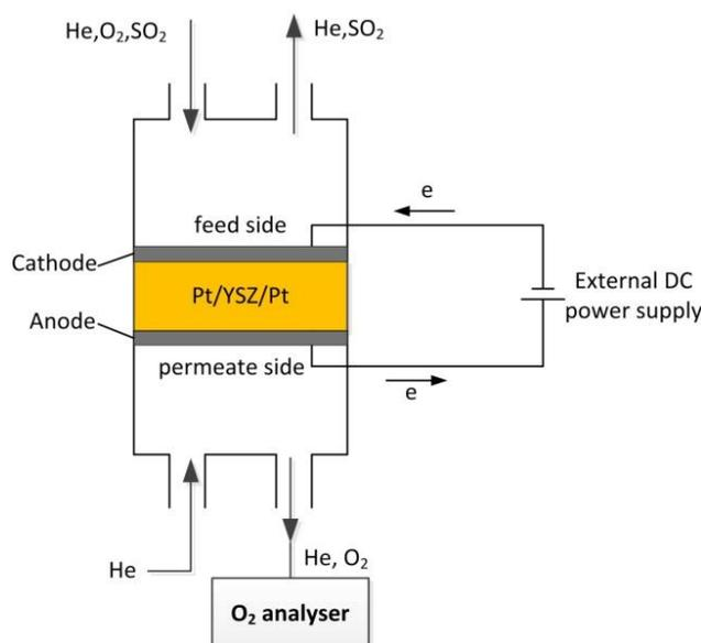
Figure 2.15: *The schematic of the oxygen permeation through Pt/8YSZ membrane*
