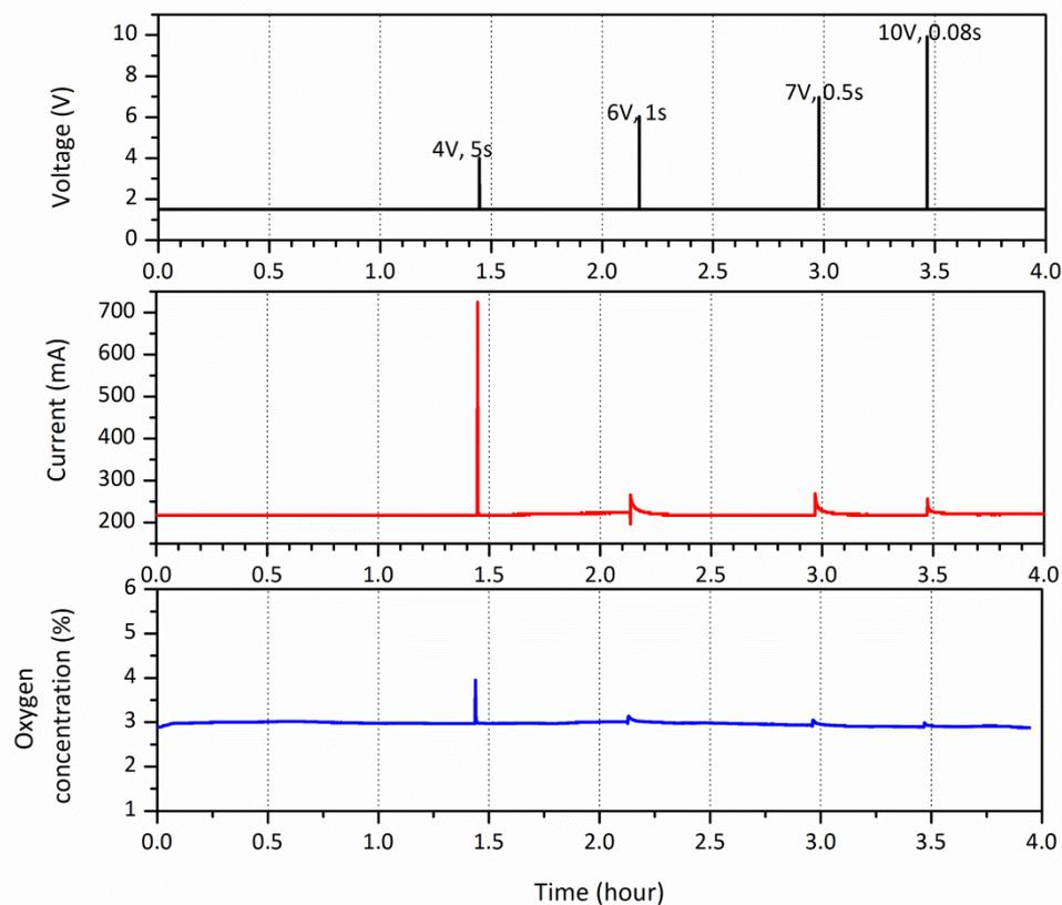
Figure 4.8: Experimental result of Pt/8YSZ membrane pellet exposed to He-O<sub>2</sub> with four positive voltage pulses, at 850°C
