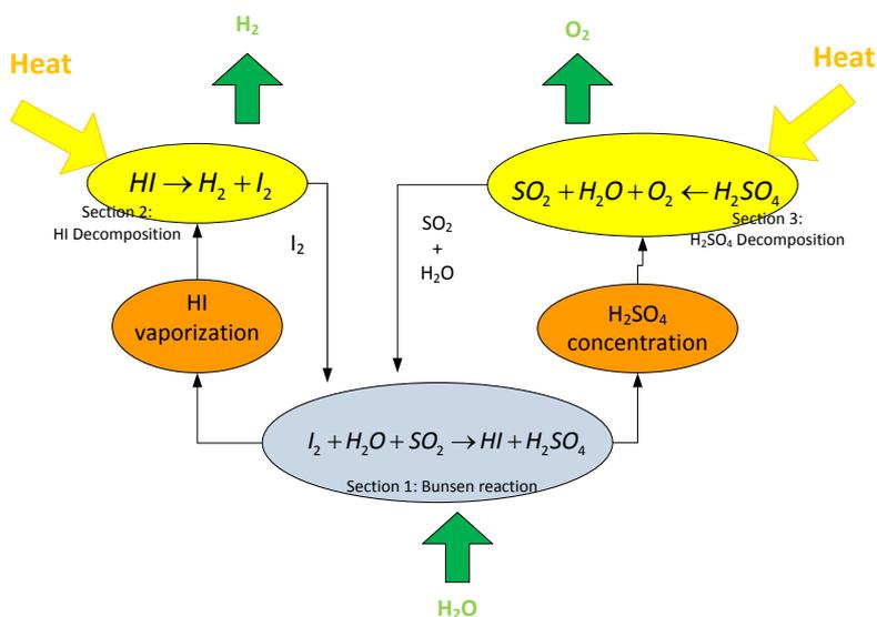
Figure 2.6: Schematic representation of the S-I cycle
