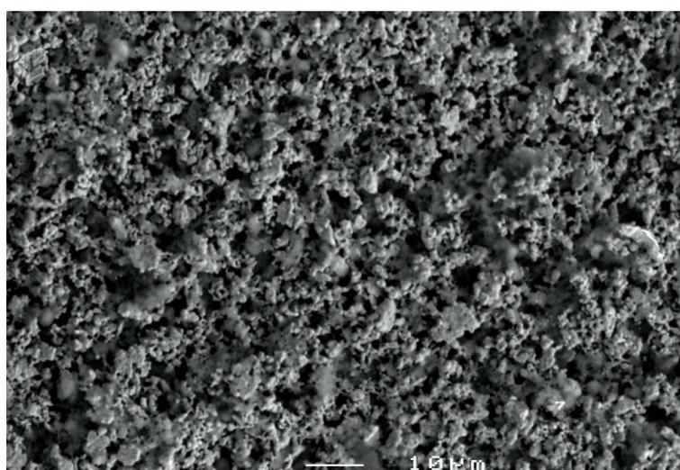
Figure 3.19: SEM image of the cathode surface of the pellet exposed by  $\text{SO}_2$
