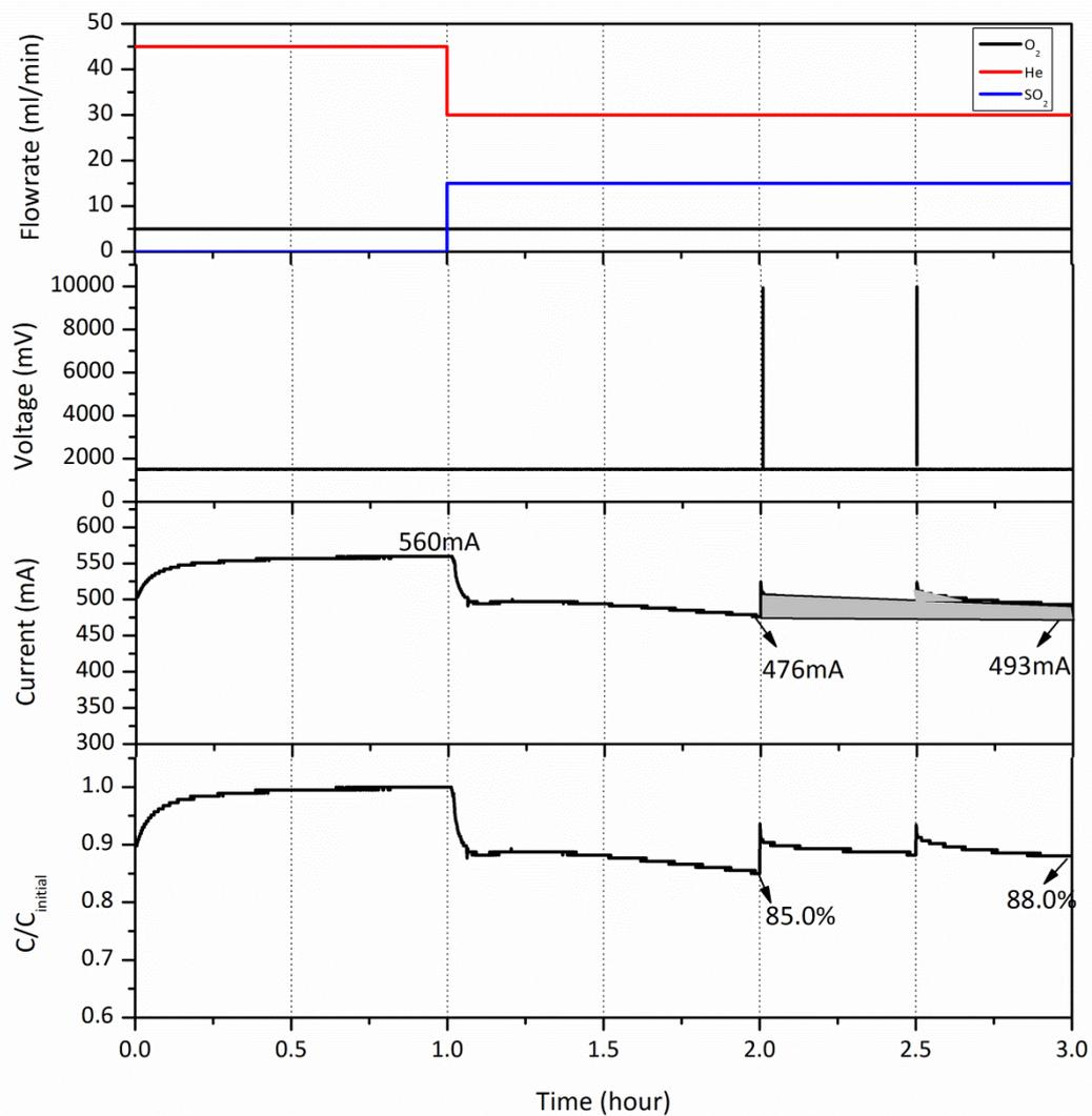
Figure 4.33: Performance change under  $\text{SO}_2$  of Pt/YSZ membrane treated by voltage pulse frequency of 2 pulses per hour, at  $850^\circ\text{C}$
