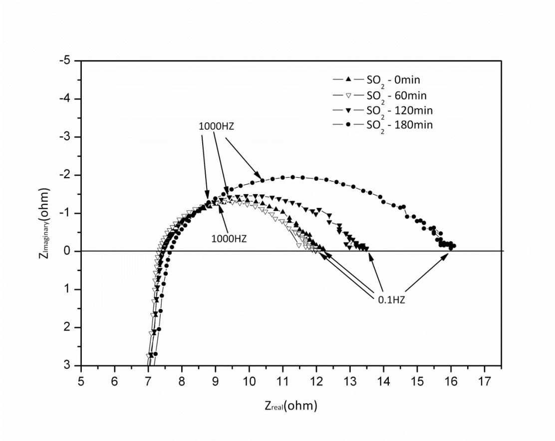
Figure 4.20: Impedance spectra of Pt/8YSZ/Pt cell recorded before and after  $SO_2$  addition to feed (Group B), at  $850^\circ C$
