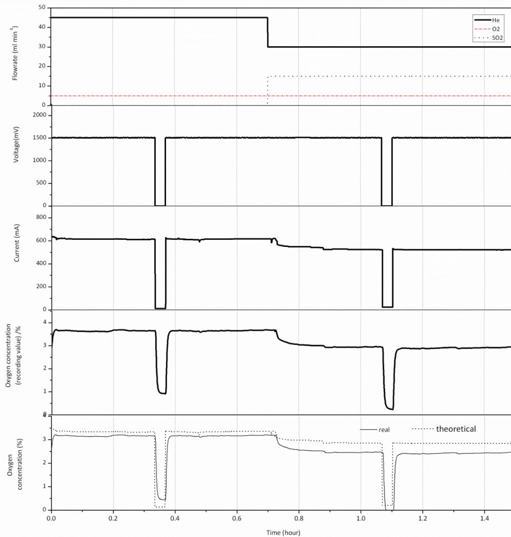
Figure 5.17: Experimental results of oxygen permeation when the feed is He-O<sub>2</sub>-SO<sub>2</sub>, at 850°C.
