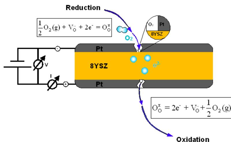
Figure 3.1: Schematic of oxygen permeation process
