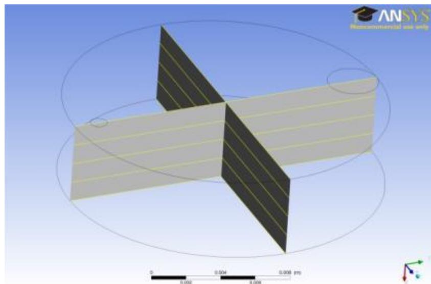
Figure 5.25: Outline of flow domain for FLUENT simulations showing lines and planes along which velocity magnitude data is collected. These lines run parallel and perpendicular to an imaginary line joining the entry and exit holes. The lines are 0, 1.25, 2.5, 3.75, 5mm from the inlet face.
