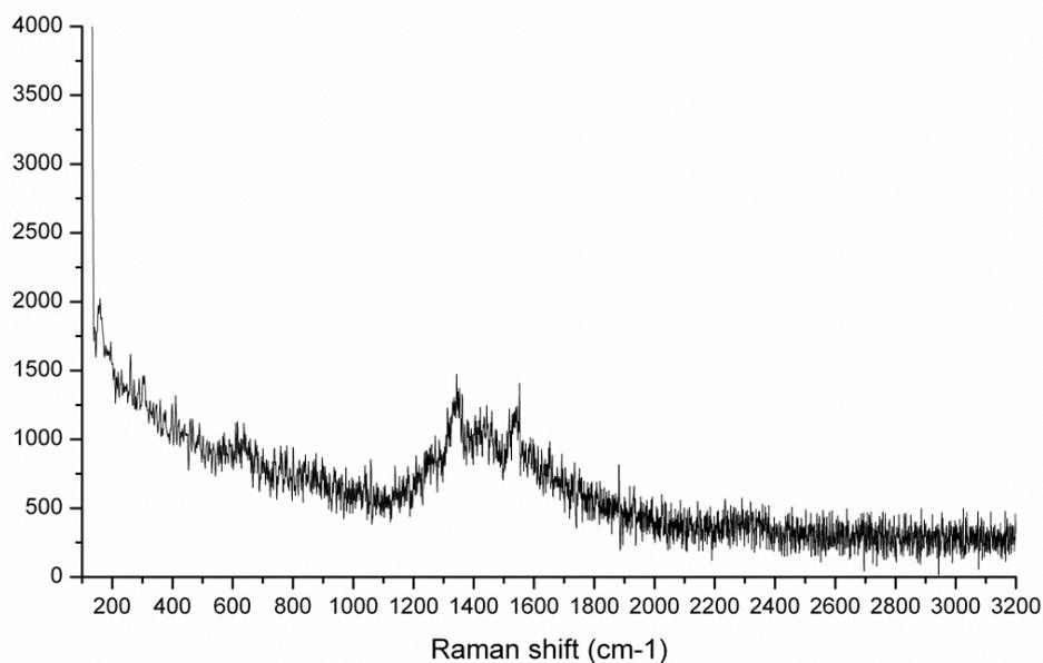
Figure 3.14: Raman spectrum for 8YSZ/Pt membrane before  $\text{SO}_2$  exposure at 850 $^{\circ}\text{C}$ , feed side
