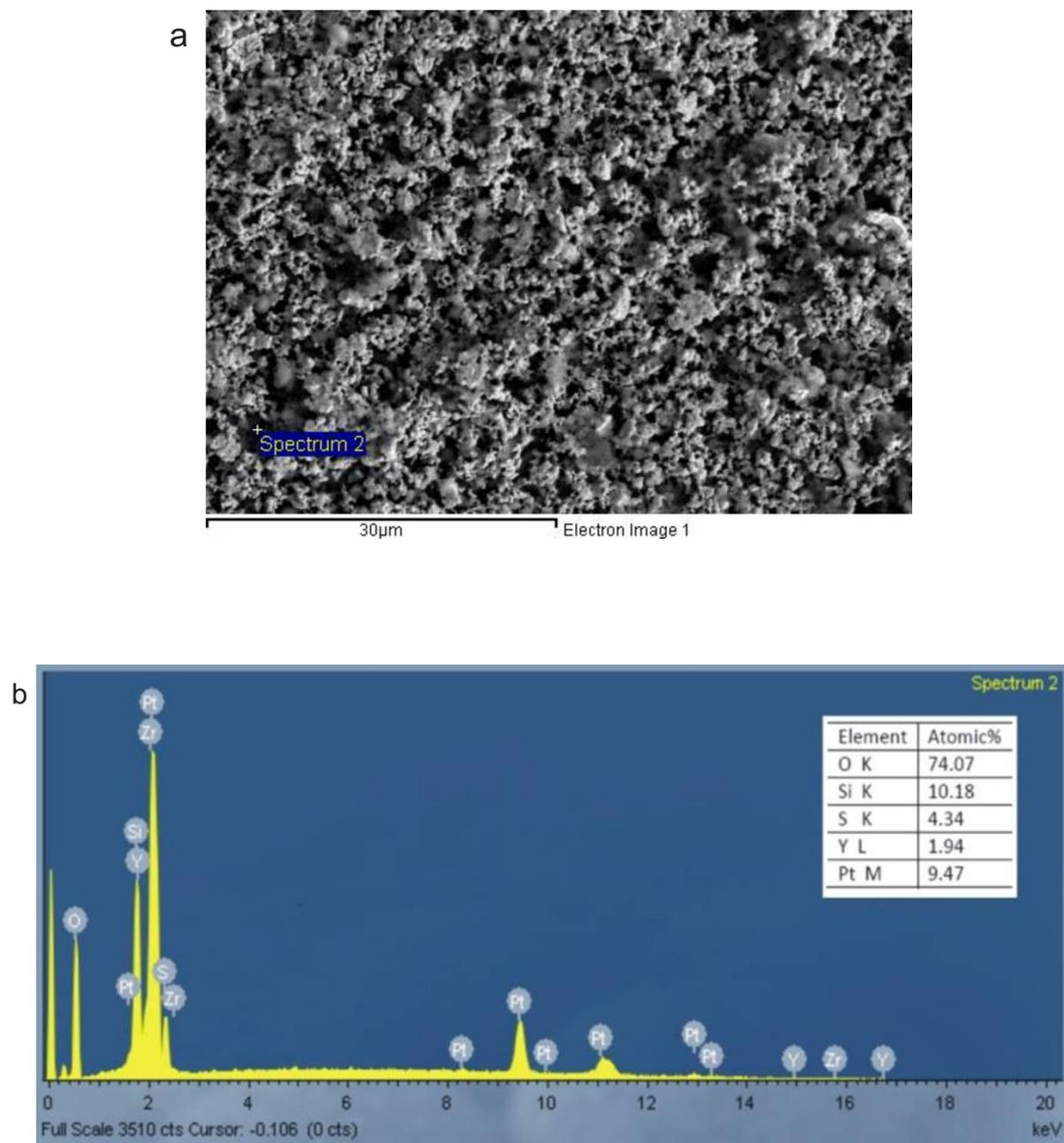
Figure 3.22: EDS elemental point analysis for the pellet treated by  $\text{SO}_2$  exposure: SEM image (a) and EDS spectrum (b)
