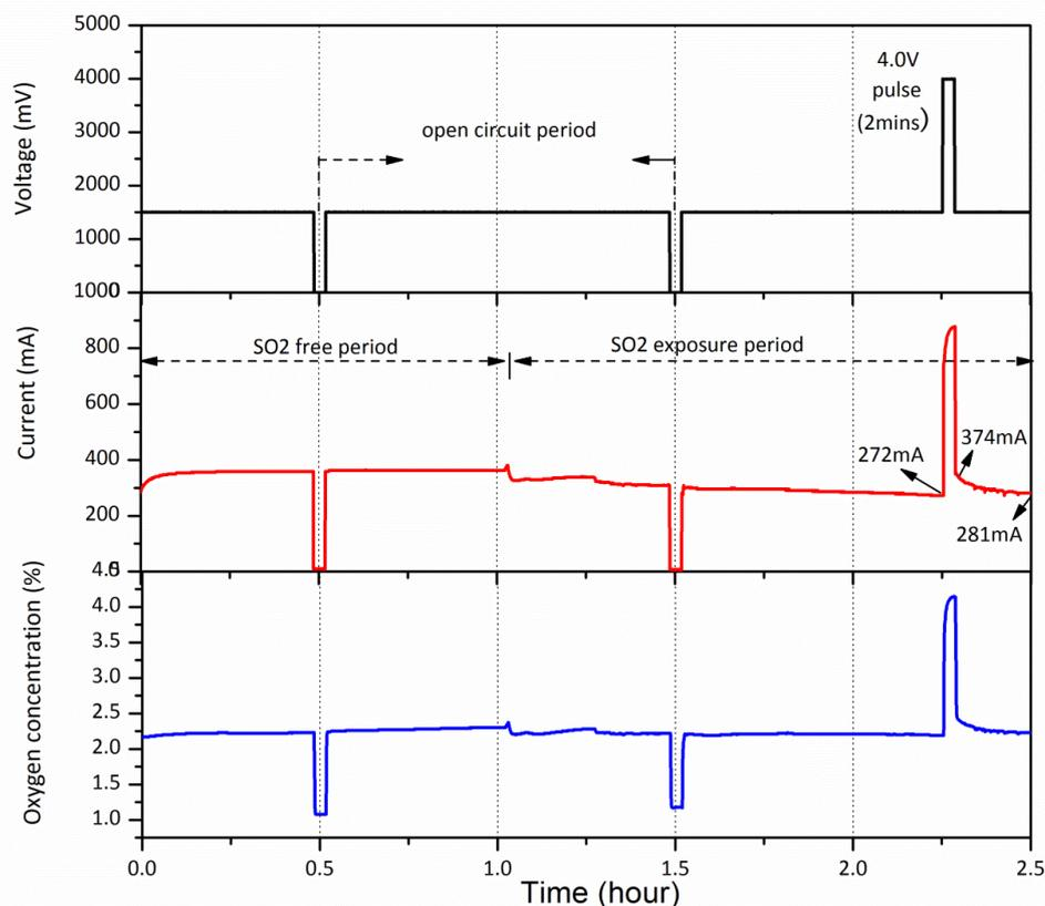
Figure 4.2: *Experimental data for YSZ/Pt pellet exposure to SO<sub>2</sub> and O<sub>2</sub> at 850°C with a 2-minute 4V positive pulse treatment*
