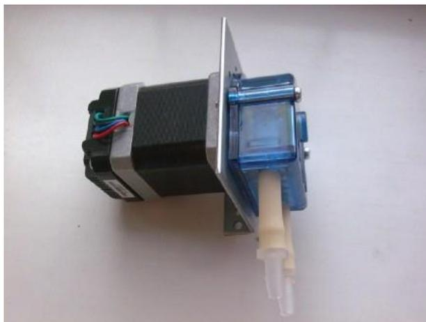
Figure 6.4: A 200 series stepper motor powered pump
