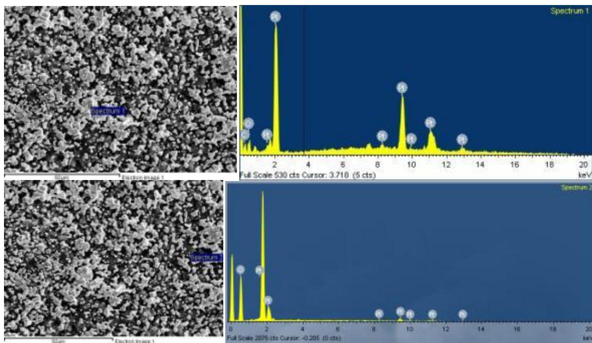
Figure 5.21: The SEM-EDX spectrum of the outer membrane surface
