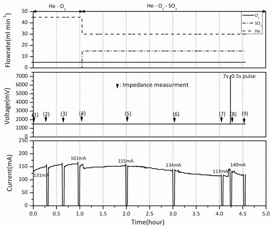
Figure 4.18: Performance degradation and recovery of Pt/8YSZ/YSZ exposed to He-O<sub>2</sub>-SO<sub>2</sub> at 850°C
