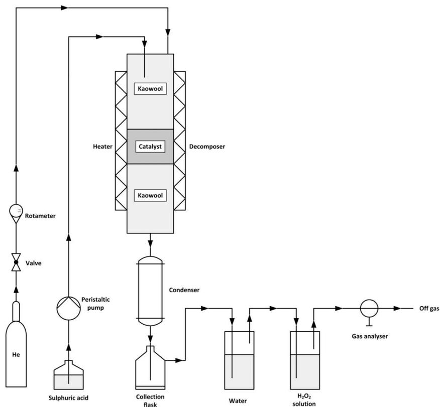
Figure 6.1: Schematic of straight-through sulphuric acid injector, catalytic decomposer, condenser, products collection flask and separation process
