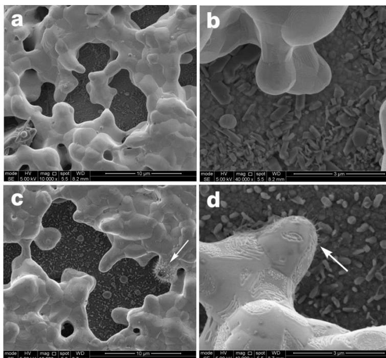
Figure 4.24: Electron microscopy images of the surface of freshly prepared cell before the test (a) and (b), the cathode surface of the cell used in the SO<sub>2</sub> exposure test (c) (d).
