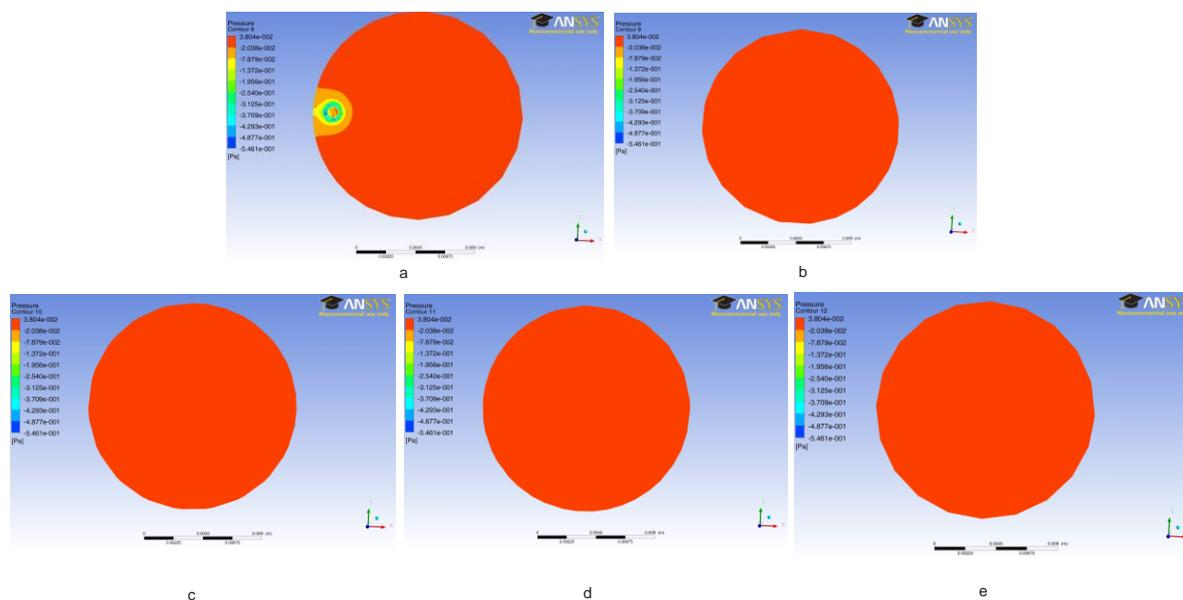
Figure 5.45: Pressure contour in the planes which are parallel to the outlet face: a)  $z=0$  (inlet); b)  $z=46.25$ ; c)  $z=92.5$ ; d)  $z=138.75$ ; e)  $z=185$  (outlet)
