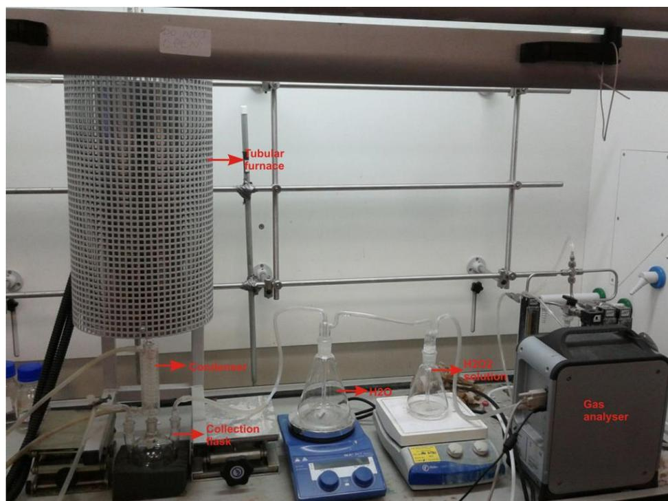
Figure 6.2: Straight-through sulphuric acid tubular, catalytic decomposer, condenser, collection flask and products separation system, prior to installing peristaltic pump
