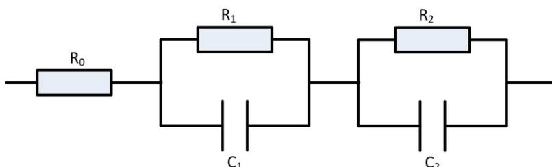
Figure 3.12: Equivalent circuit for Pt/8YSZ/Pt pellet
