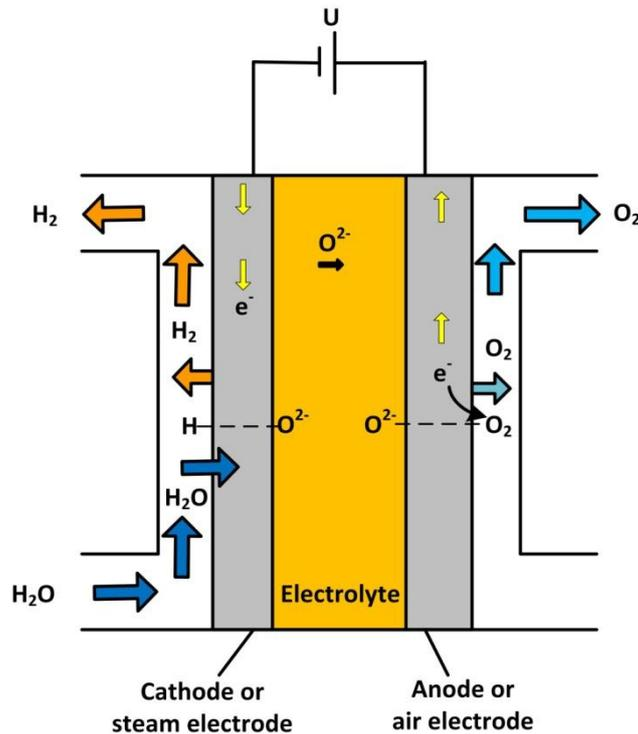
Figure 2.12: Schematics of SOEC hydrogen production (Ulrich Vogt et al.)
