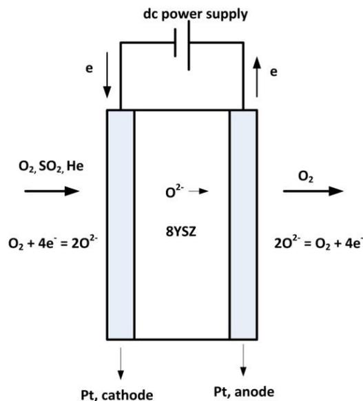
Figure 4.9: Schematic of a Pt/8YSZ/Pt oxygen separation membrane with an external dc power supply
