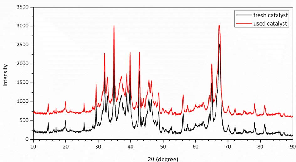
Figure 6.13: XRD data of Pt/Al<sub>2</sub>O<sub>3</sub> catalyst before and after acid decomposition
