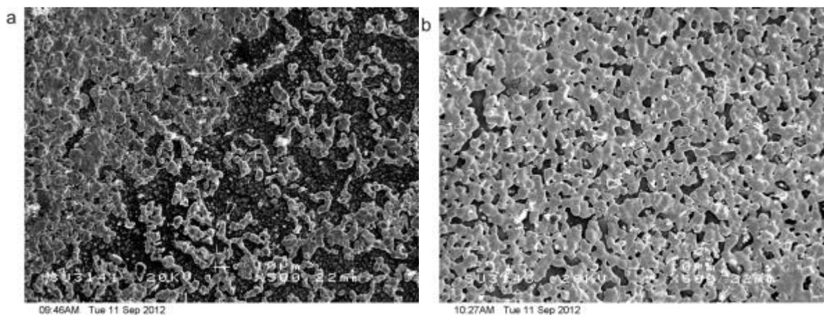
Figure 5.3: The SEM image of the inner Pt electrode layer (a) and outer Pt electrode layer(b)
