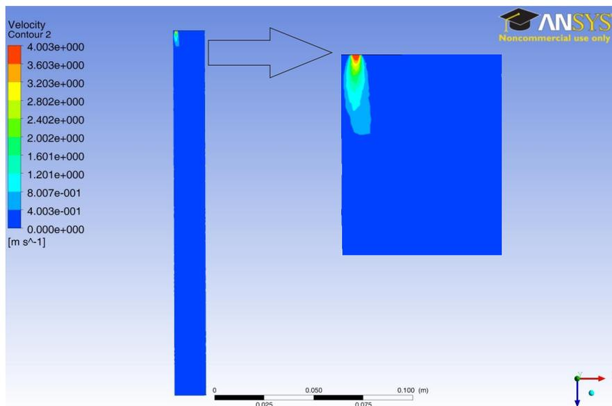
Figure 5.41: Velocity contour in the middle plane which across the inlet and outlet
