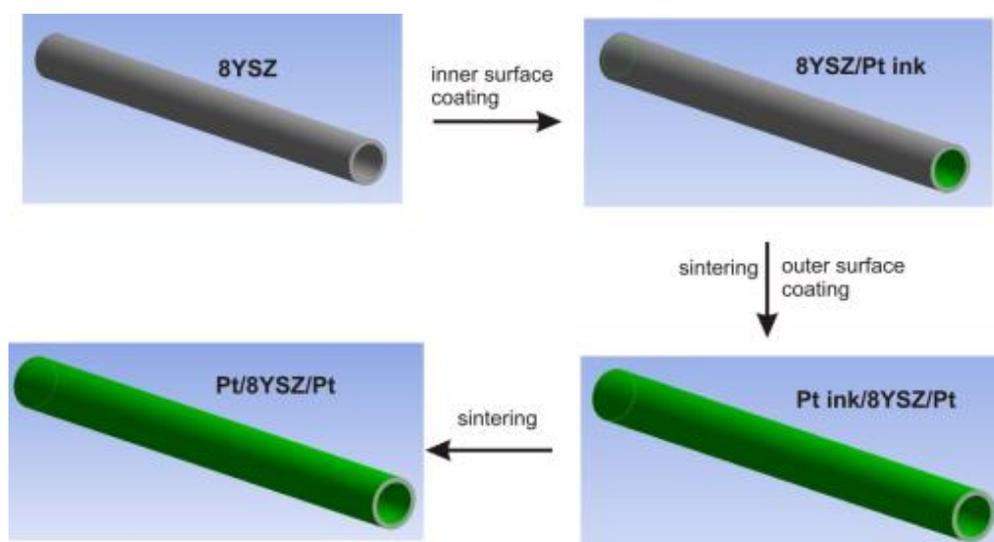
Figure 5.2: Preparation of Pt/8YSZ/Pt tubular membrane
