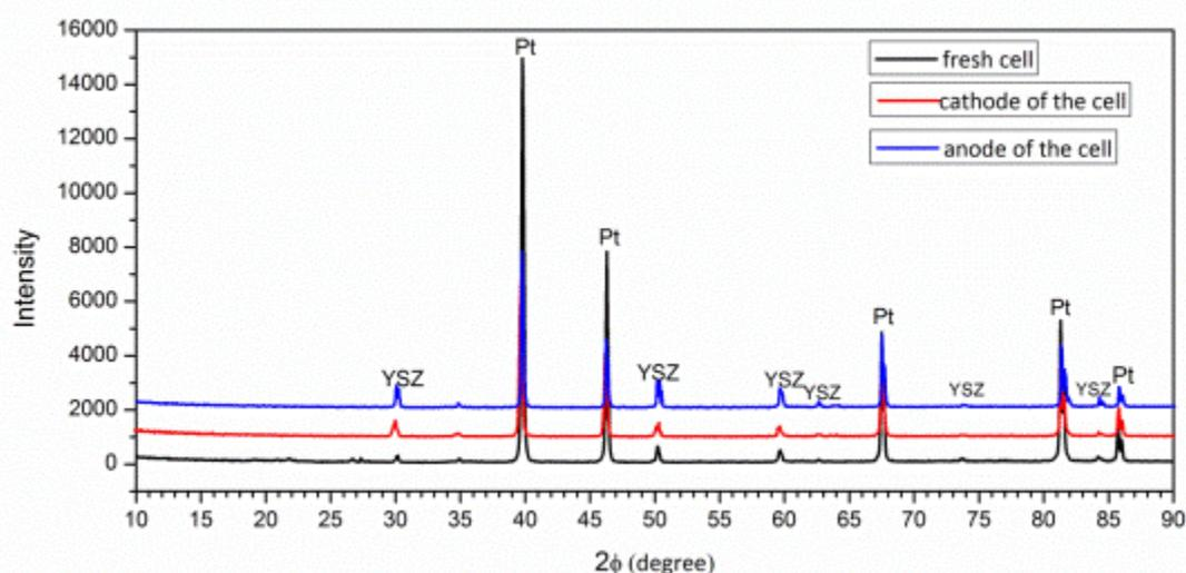
Figure 5.19: XRD data of membrane tube feed side, permeate side after experiments
