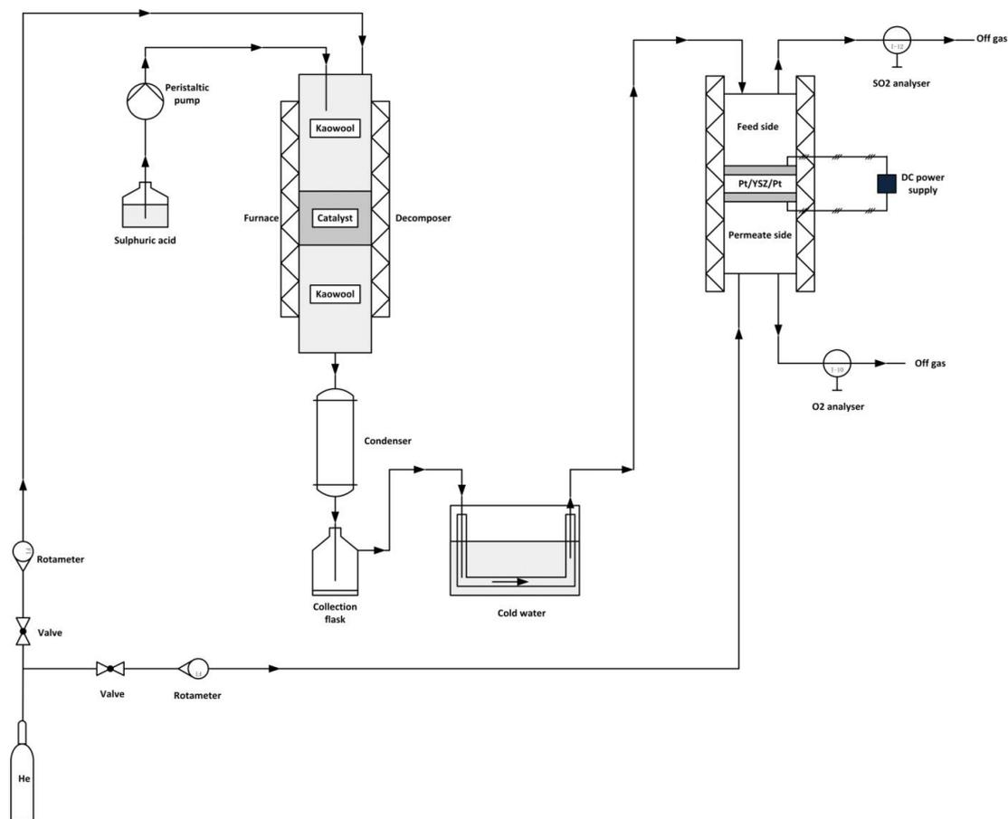
Figure 7.1: Schematic of experimental rig
