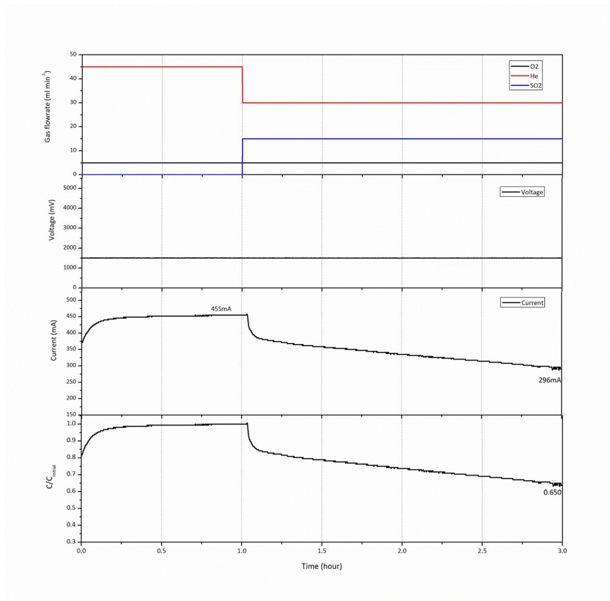
Figure 4.31: Performance change of Pt/YSZ membrane exposed to SO<sub>2</sub>, at 850°C
