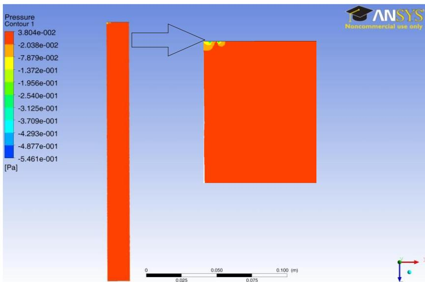
Figure 5.42: Pressure contour in the middle plane which across the inlet and outlet
