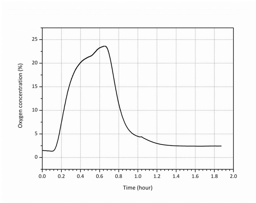
Figure 6.10: *Oxygen concentration change with time in  $\text{H}_2\text{SO}_4$  thermal decomposition (Section I)*
