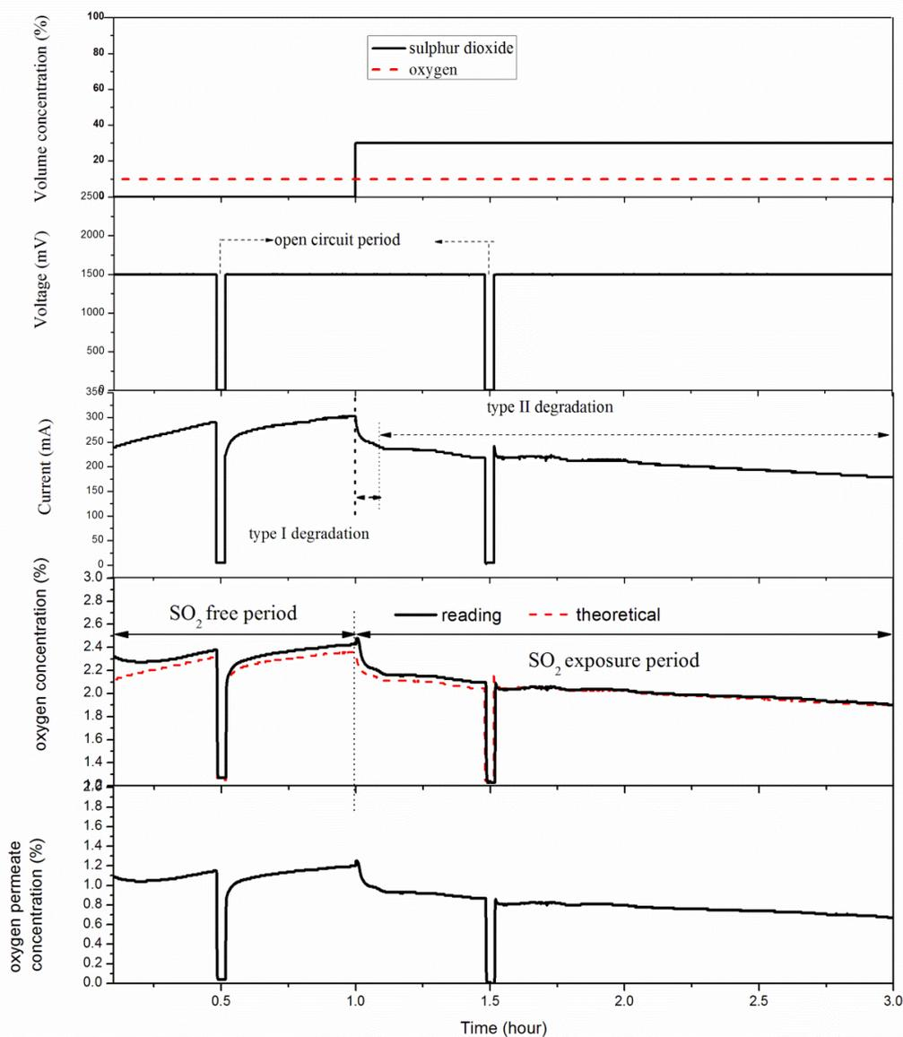
Figure 3.9: Experimental results of Pt/8YSZ/Pt membrane pellet performance with  $\text{SO}_2$  free period and  $\text{SO}_2$  exposure period at  $850^\circ\text{C}$
