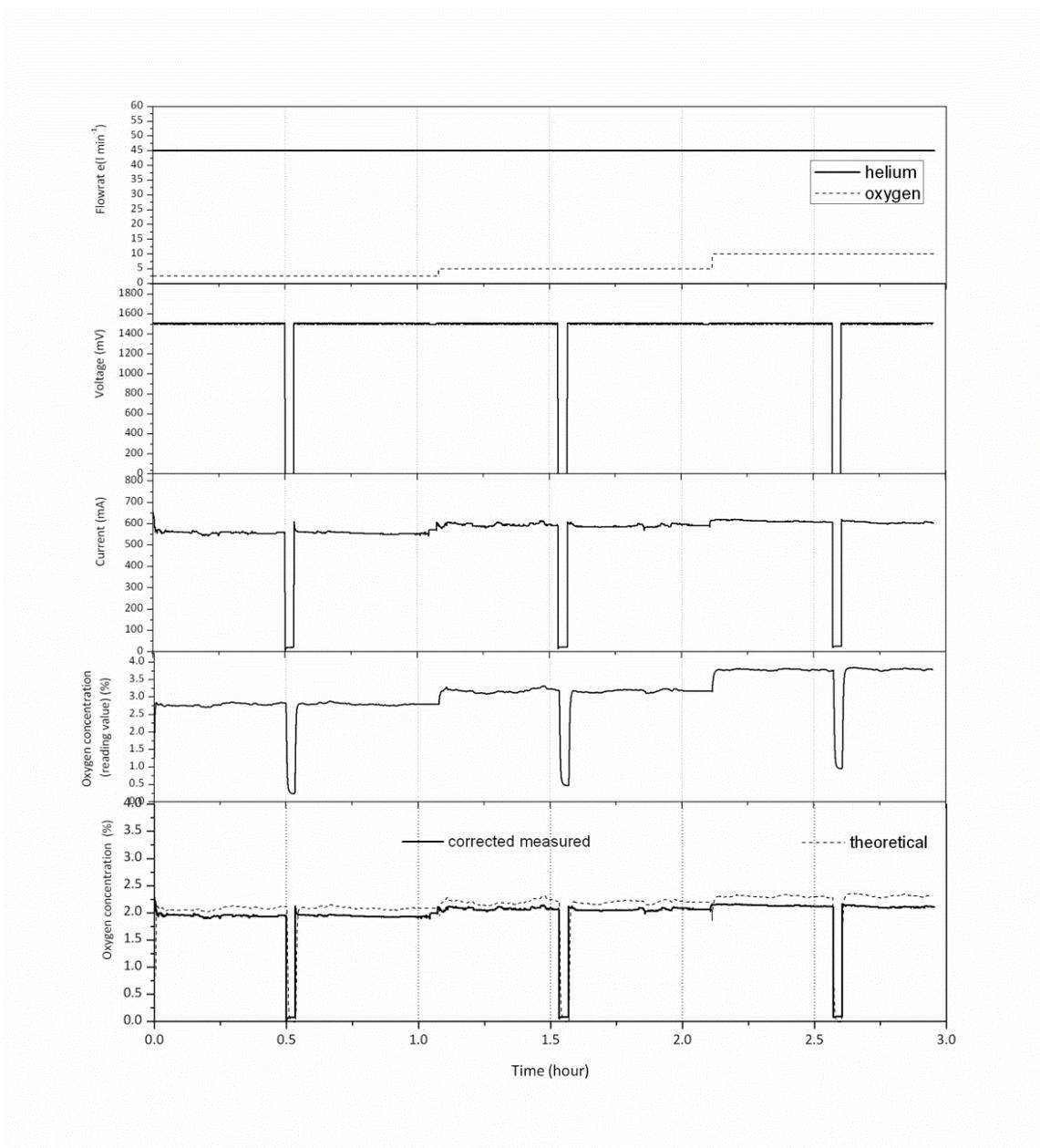
Figure 5.16: Experimental results of oxygen permeation when the feed is  $\text{He-O}_2$ , at  $850^\circ\text{C}$ .
