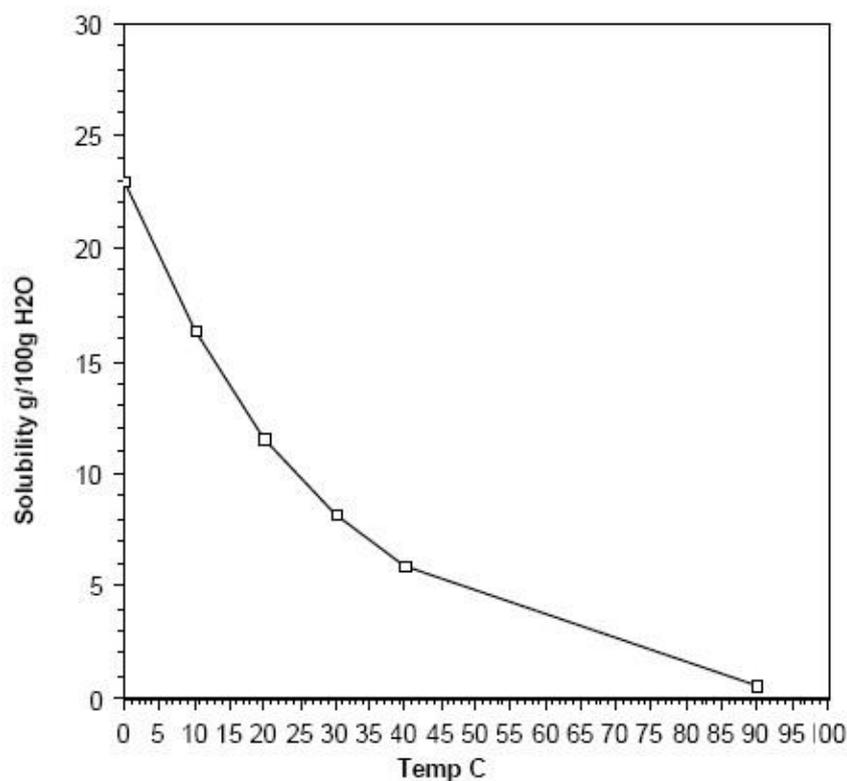
Figure 6.9:  $\text{SO}_2$  solubility in  $\text{H}_2\text{O}$  at different temperature (Source: Kirk Othmer Ency of Chemical Technology)
