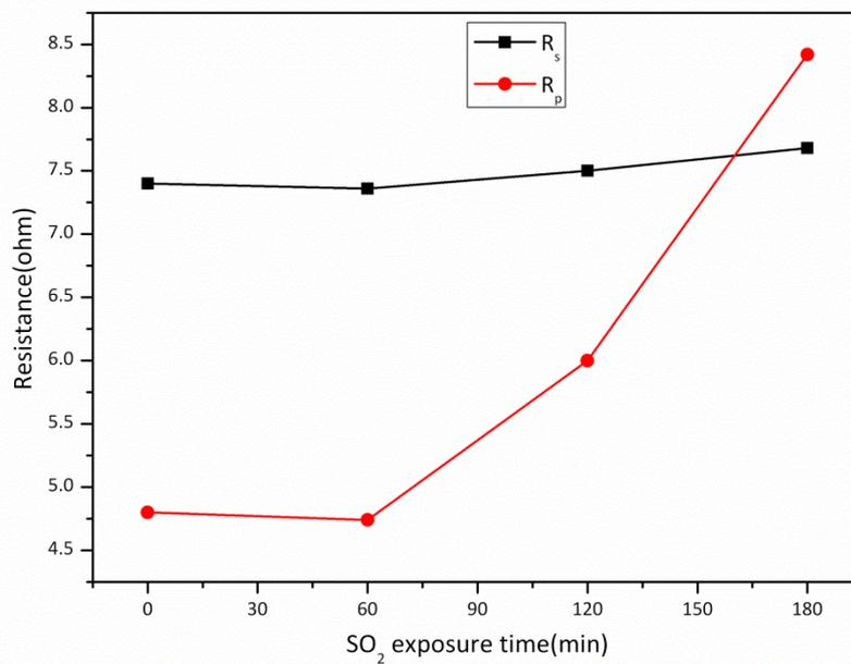
Figure 4.22: Pt/8YSZ/Pt cell, serial resistance ( $R_s$ ) and polarization resistance ( $R_p$ ) derived from impedance spectra (Group B) recorded in  $\text{SO}_2$  exposure period, at  $850^\circ\text{C}$ .
