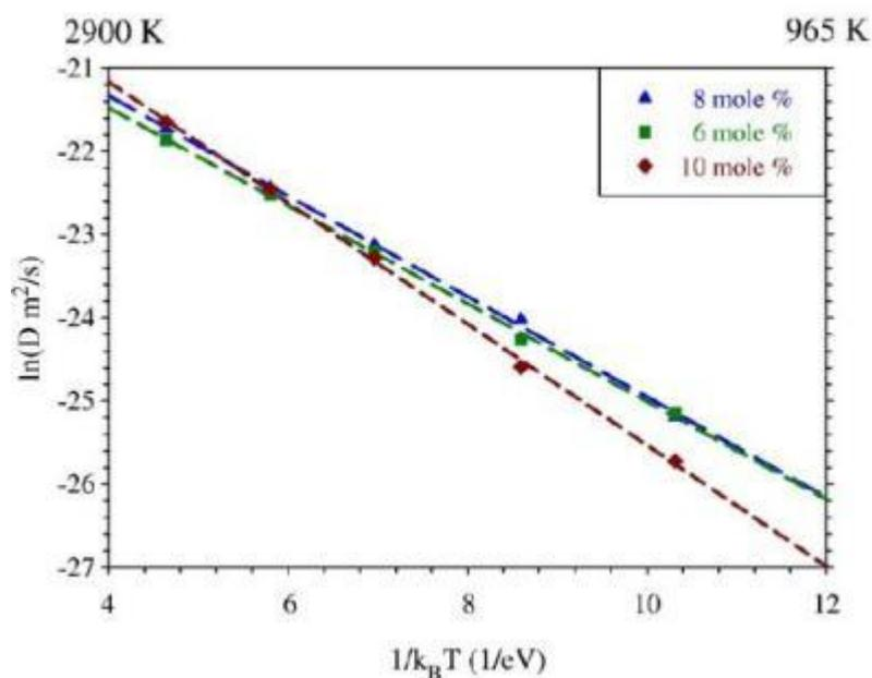
Figure 5.23: Arrhenius plot of the diffusion coefficient as a function of reciprocal temperature ( $1/T$ ) for 6, 8, and 10 mol% YSZ (Devanathan et al. 2006).
