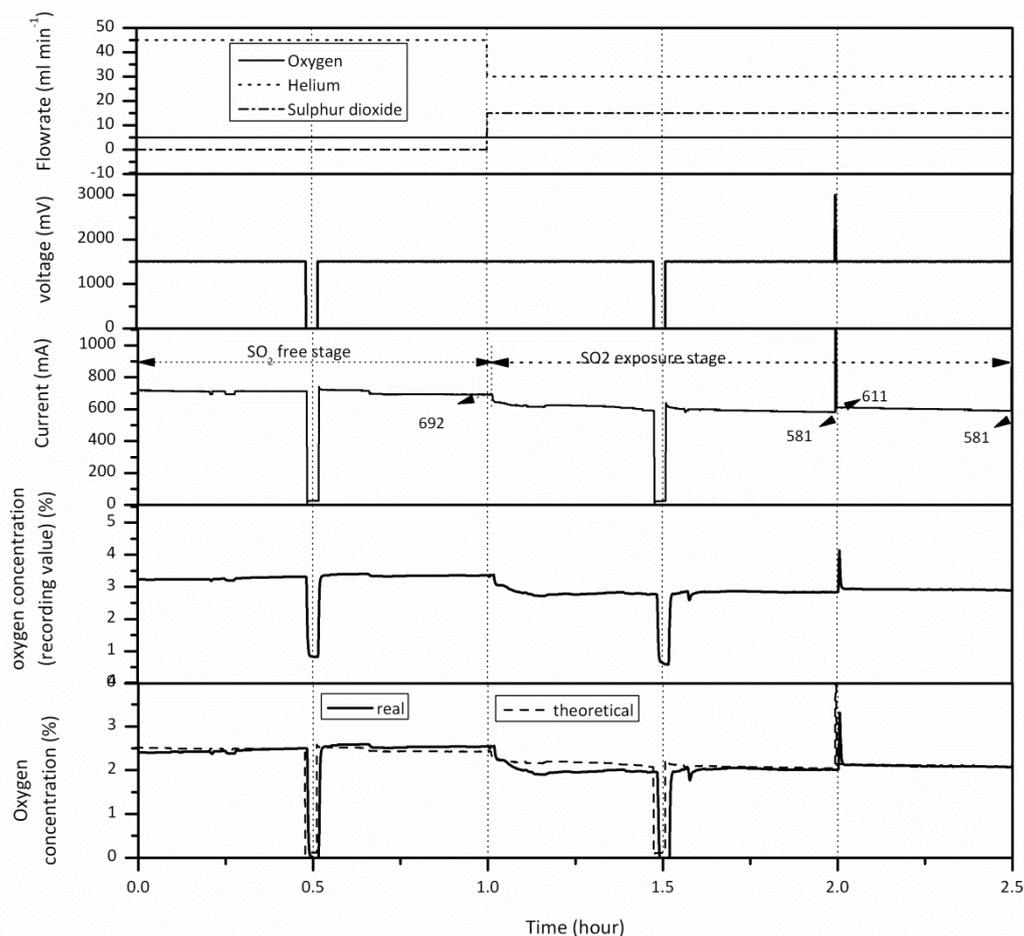
Figure 5.18: Results of oxygen permeation when the feed is He-O<sub>2</sub>-SO<sub>2</sub>, with a 3V, 10 seconds voltage pulse treatment.
