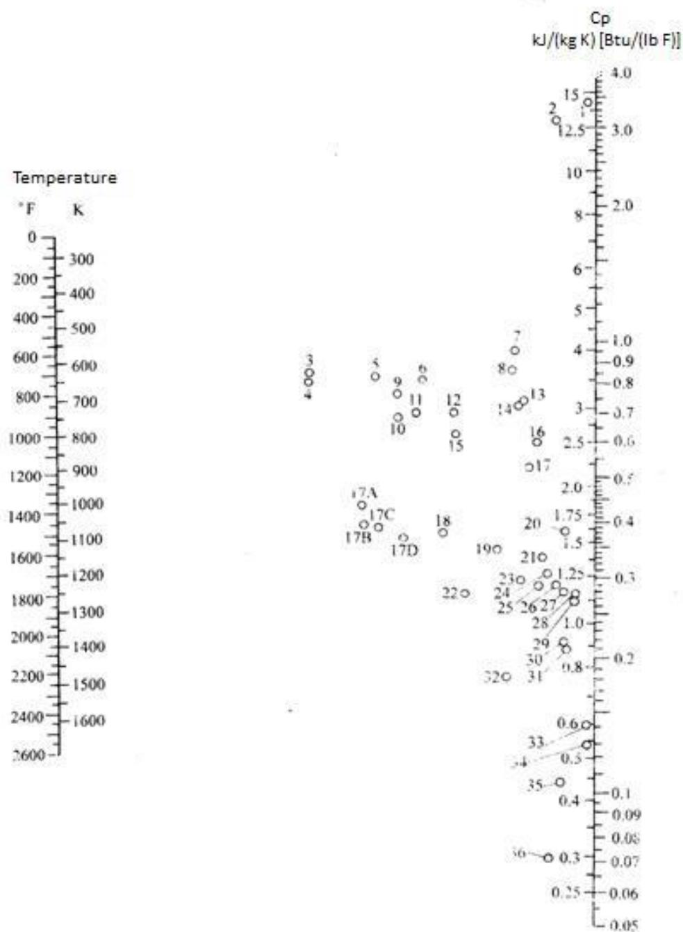
Figure A.1: Specific heat capacity ( $C_p$ ) of gases at 101.33kPa (Y. Y. Yao 1999)
