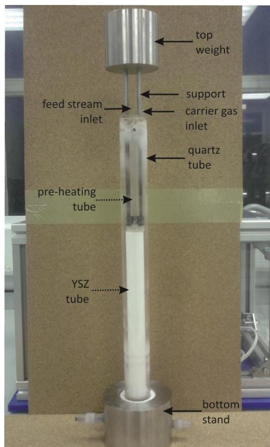
Figure 5.10: Assembly of the rig
