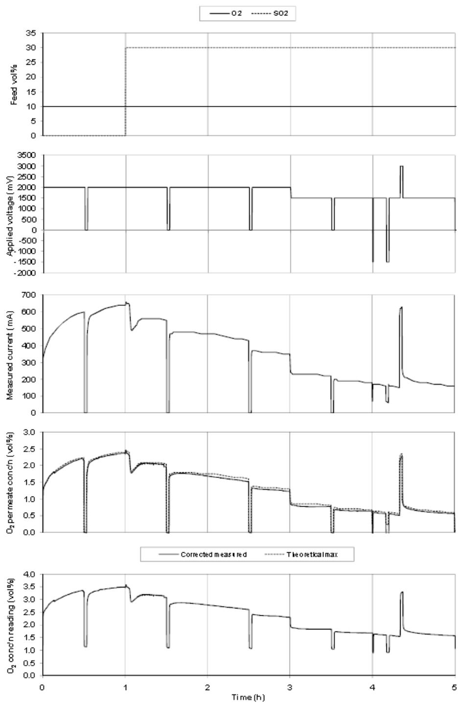
Figure 2.17: Pt/8YSZ/Pt membrane performance exposed to SO<sub>2</sub> and O<sub>2</sub> at 850°C with negative and positive dc voltage pulses
