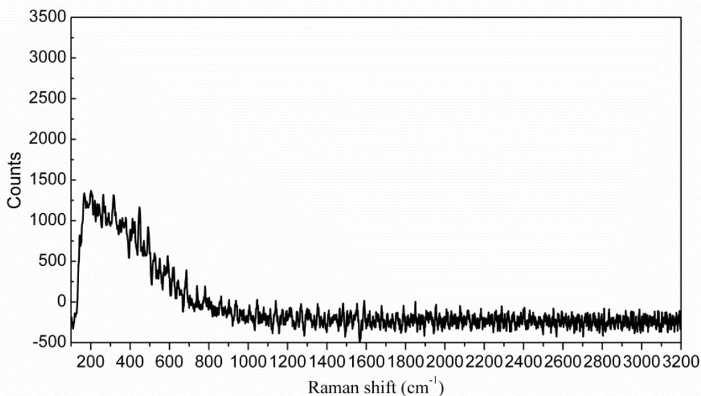
Figure 3.15: Raman spectrum for YSZ/Pt membrane after  $\text{SO}_2$  exposure at 850 $^{\circ}\text{C}$ , feed side
