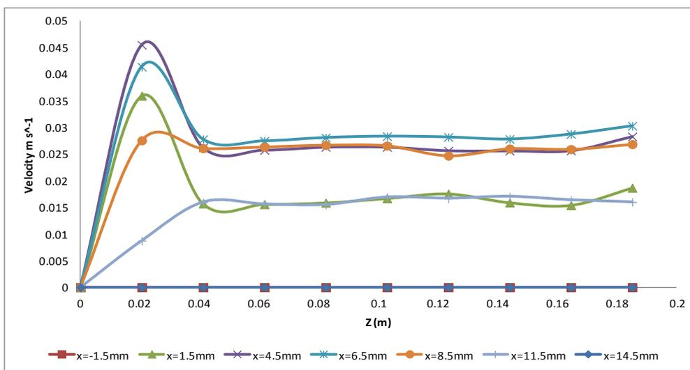
Figure 5.43: Velocity change along the lines on the middle plane
