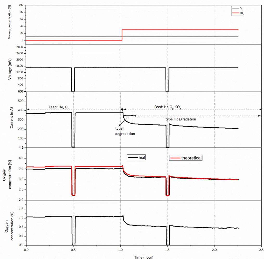
Figure 3.13: Experimental results of Pt/8YSZ membrane performance exposed to  $\text{SO}_2$  at  $850^\circ\text{C}$ , the 2nd run.
