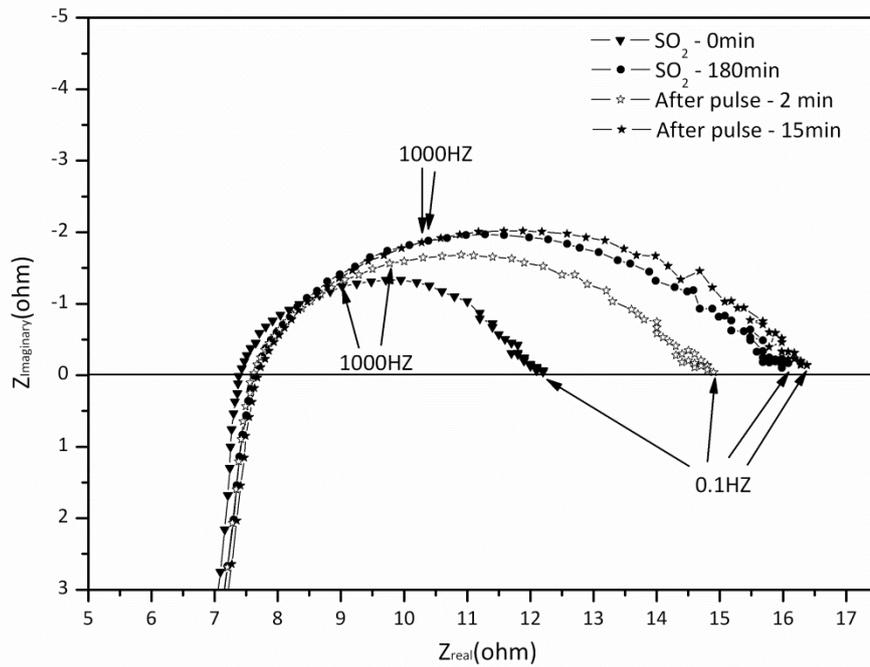
Figure 4.21: Impedance spectra of Pt/8YSZ/Pt cell recorded before  $\text{SO}_2$  addition, before and after voltage pulse treatment (Group C), at  $850^\circ\text{C}$
