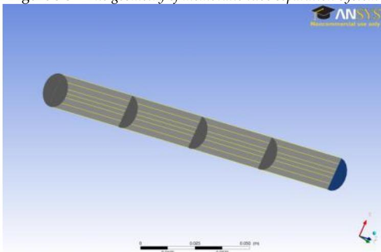
Figure 5.38: Outline of flow domain for FLUENT simulations showing lines and planes along which velocity magnitude data is collected. One plane crosses the inlet and outlet. The other five planes is parallel to outlet face [from inlet face,  $z=0$ , 46.25, 92.5, 138.75 and 185mm (outlet)]. These lines run parallel to Z axis. X coordinates of these lines are -1.5, 1.5, 4.5, 6.5, 8.5, 11.5 and 14.5mm.
