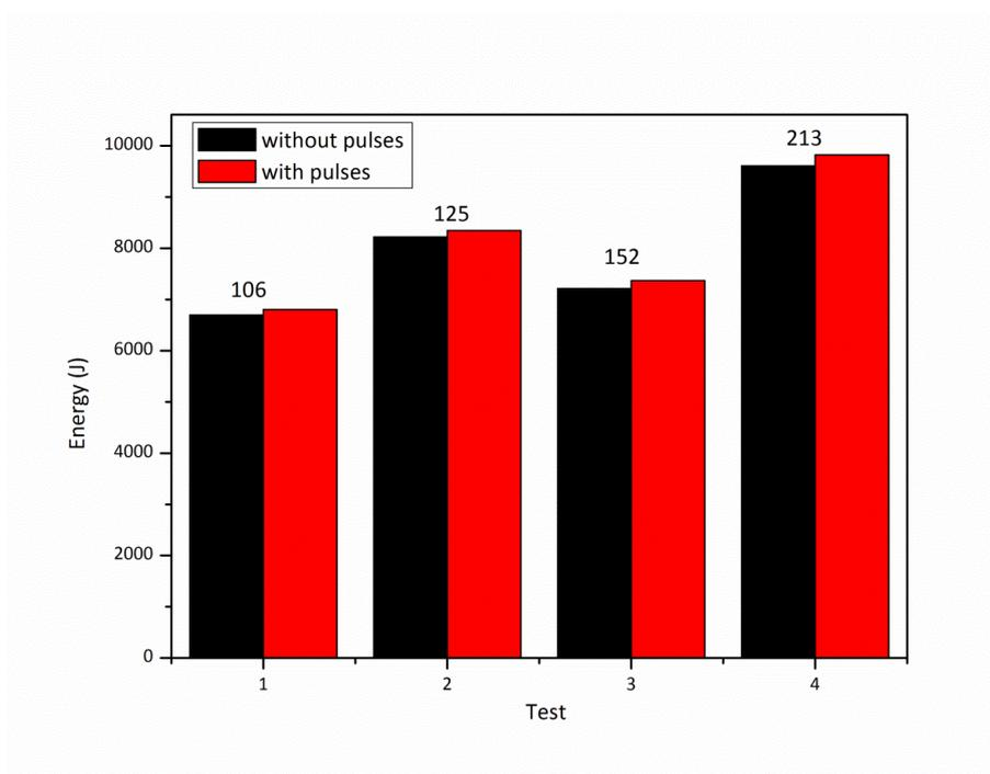
Figure 4.38: The comparison of energy consumed in the four tests without and with pulses
