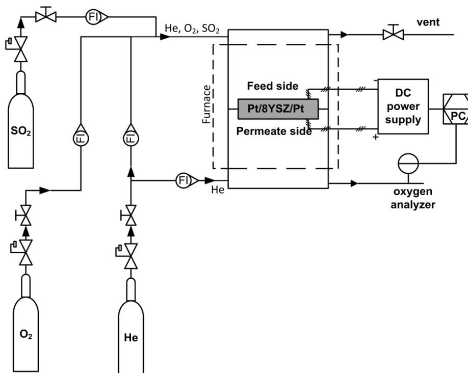
Figure 3.8: Schematic diagram of experimental apparatus
