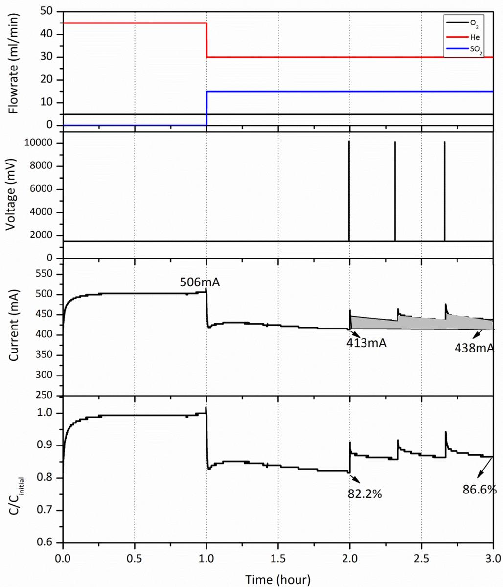
Figure 4.34: Performance change under  $\text{SO}_2$  of Pt/YSZ membrane treated by voltage pulse frequency of 3 pulses per hour, at  $850^\circ\text{C}$
