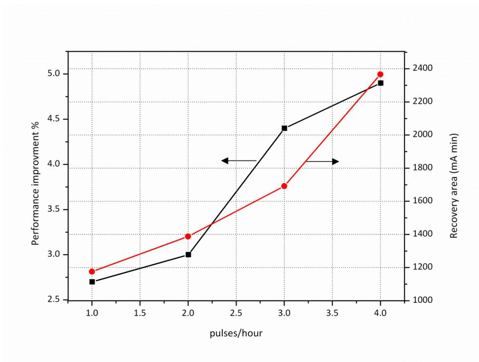
Figure 4.36: The extent of membrane performance recovery by voltage pulses
