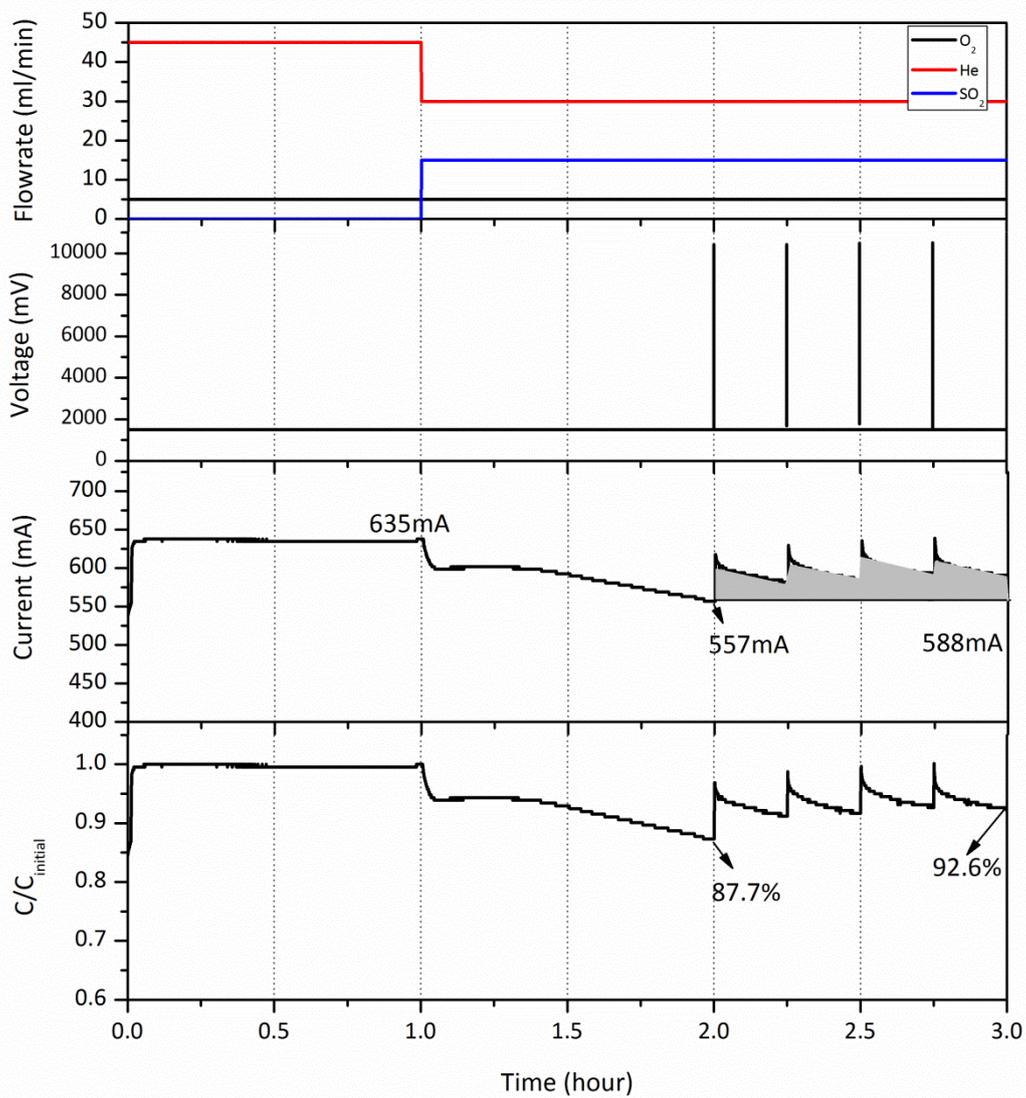
Figure 4.35: Performance change under  $\text{SO}_2$  of Pt/YSZ membrane treated by voltage pulse frequency of 4 pulses per hour, at  $850^\circ\text{C}$
