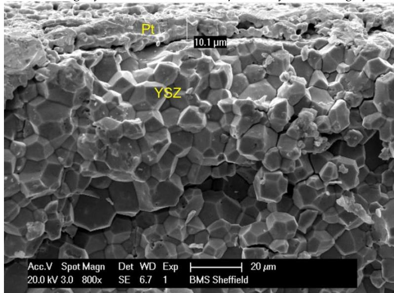
Figure 3.5: SEM image of a Pt/8YSZ membrane pellet cross section, the magnification is 800x
