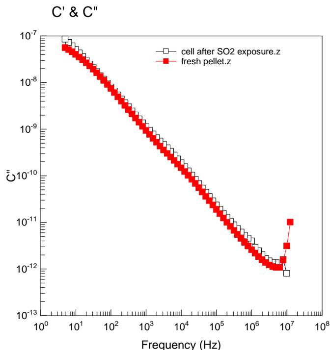
Figure 3.11: The frequency dependence of the capacitance plot for YSZ/Pt at 306 °C before and after SO<sub>2</sub> exposure
