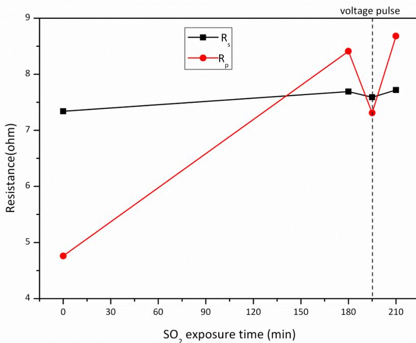
Figure 4.23: Pt/8YSZ/Pt cell, serial resistance ( $R_s$ ) and polarization resistance ( $R_p$ ) derived from impedance spectra (Group C), at 850°C
