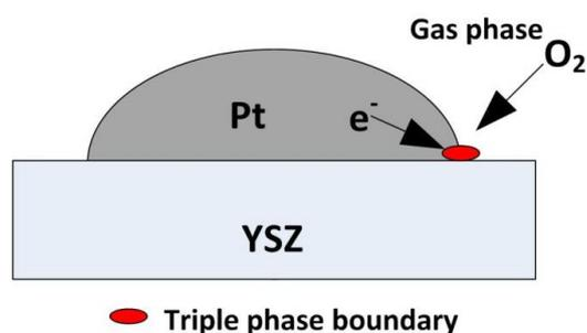
Figure 3.2: Schematic diagram of the triple-phase boundary
