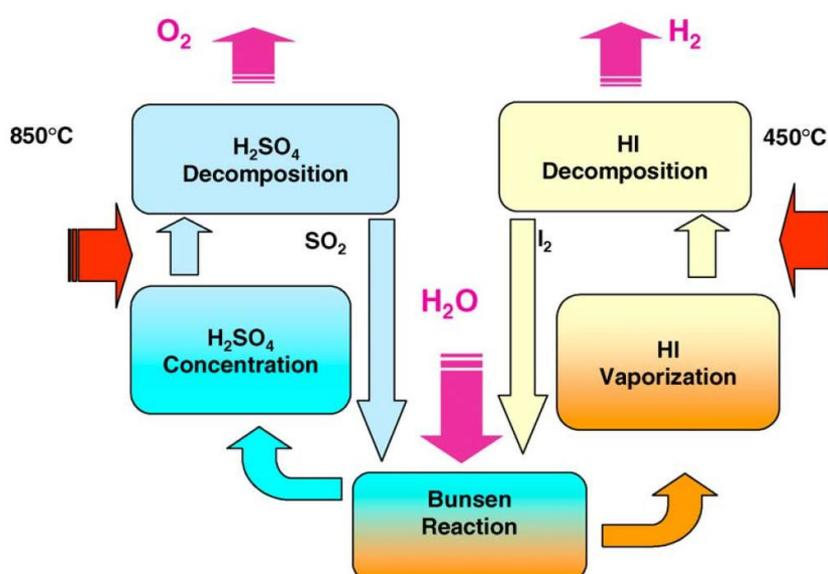
Figure 1.1: Schematic representation of the S-I cycle (Vitart et al. 2006)
