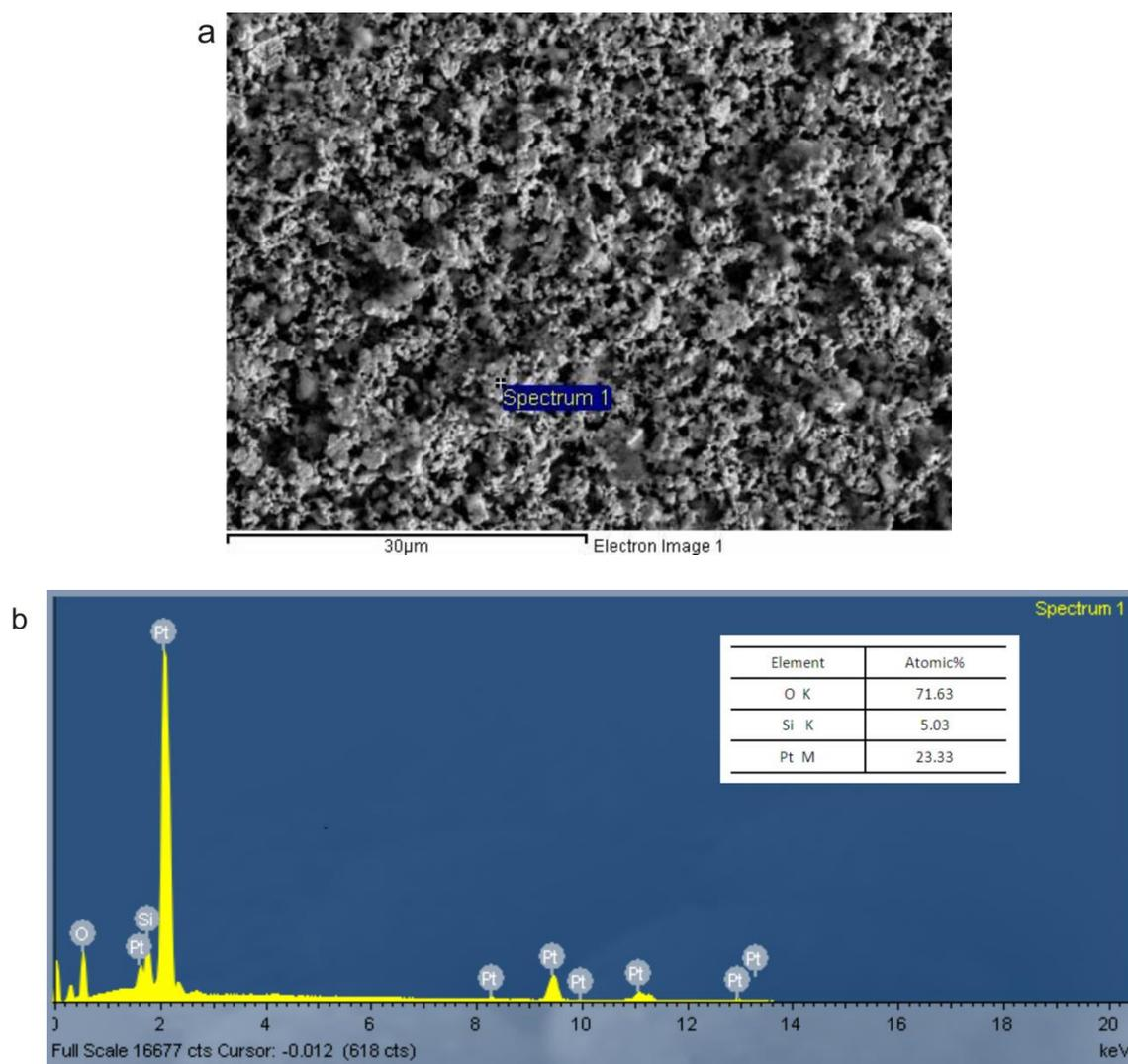
Figure 3.20: EDS elemental point analysis for the pellet treated by  $\text{SO}_2$  exposure: SEM image (a) and EDS spectrum (b)
