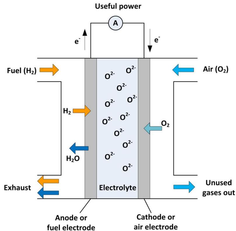
Figure 2.11: Concept diagram of SOFC based on oxygen-ion conductors
