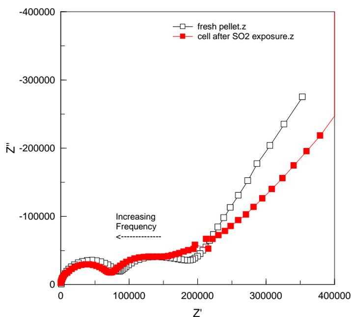
Figure 3.10:  $Z^*$  plot for YSZ/Pt at 306°C before and after  $SO_2$  exposure
