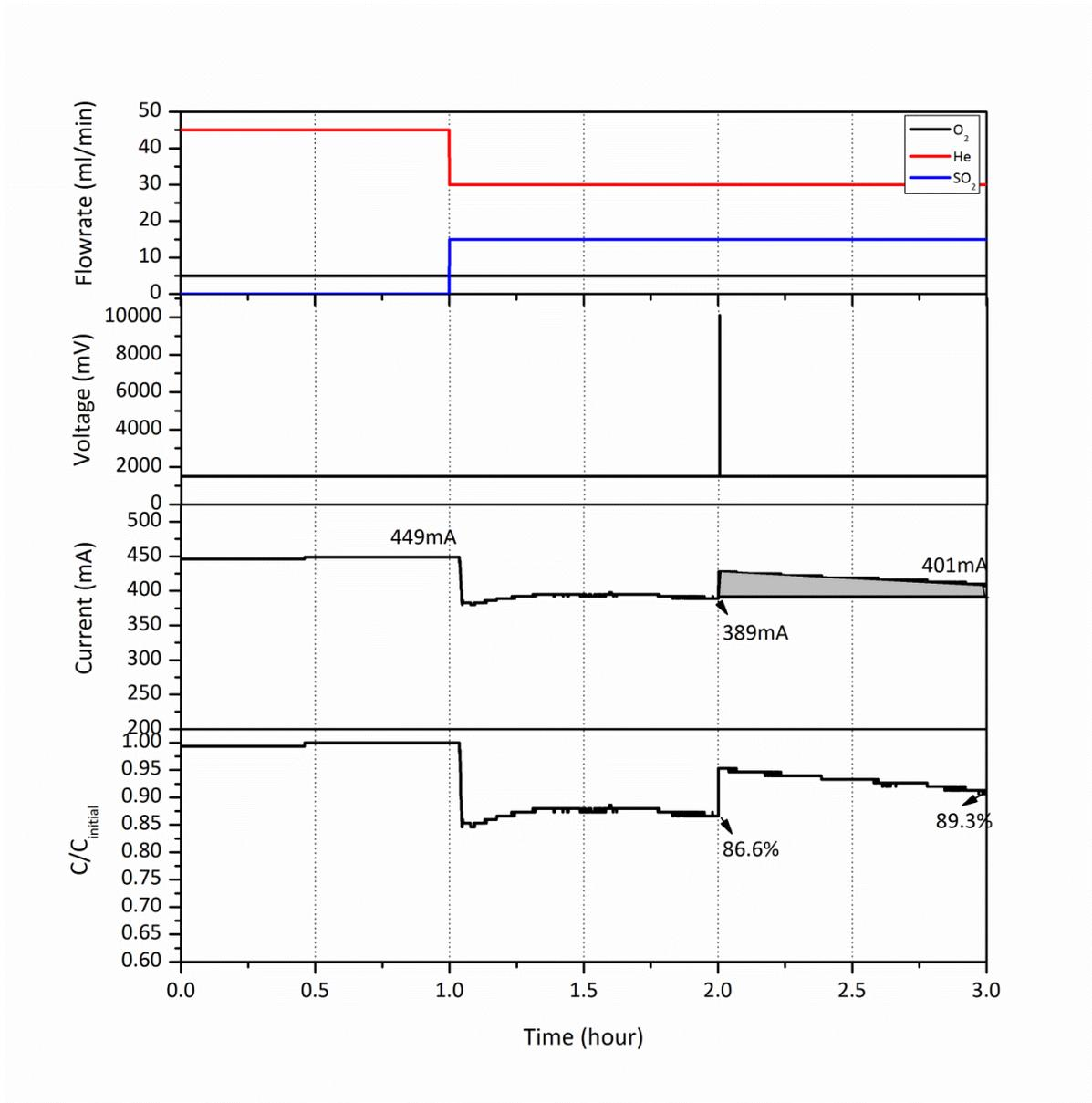
Figure 4.32: Performance change under  $\text{SO}_2$  of Pt/YSZ membrane treated by voltage pulse frequency of 1 pulse per hour, at  $850^\circ\text{C}$
