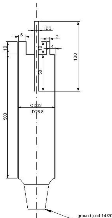
Figure 6.6: Schematic diagram of quartz decomposer for sulphuric acid decomposition. All measurements are in mm
