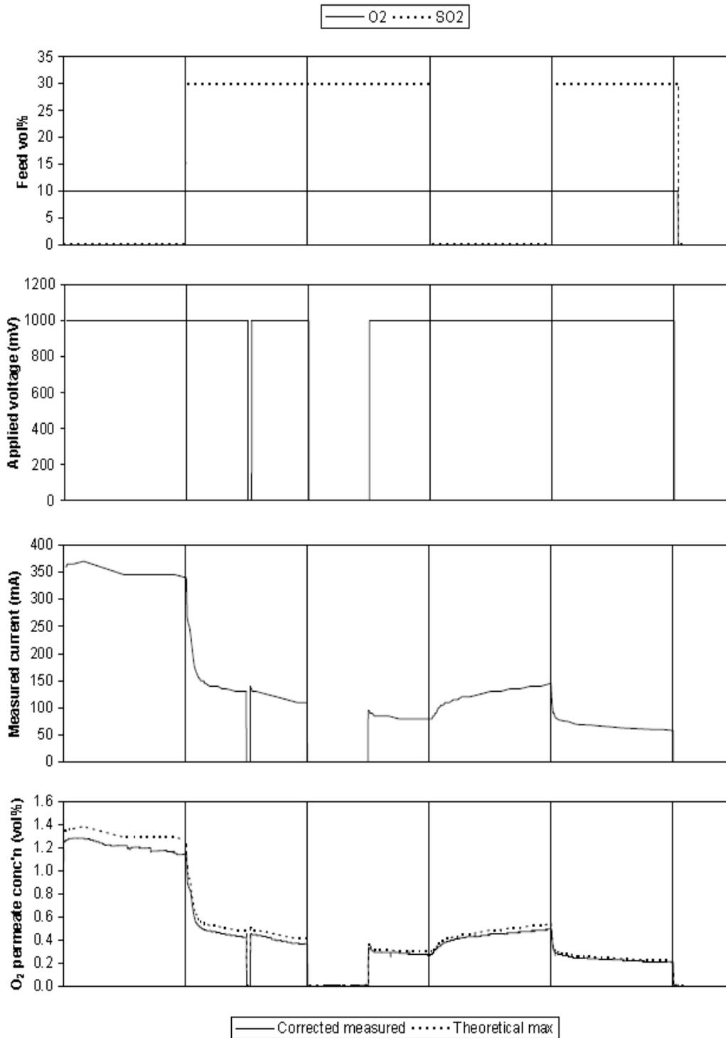
Figure 2.16: Experimental result of membrane exposure He-O<sub>2</sub>-SO<sub>2</sub> at 800°C with external voltage application—100ml/min pure He in permeate side, 50ml/min 20% O<sub>2</sub> in feed.
