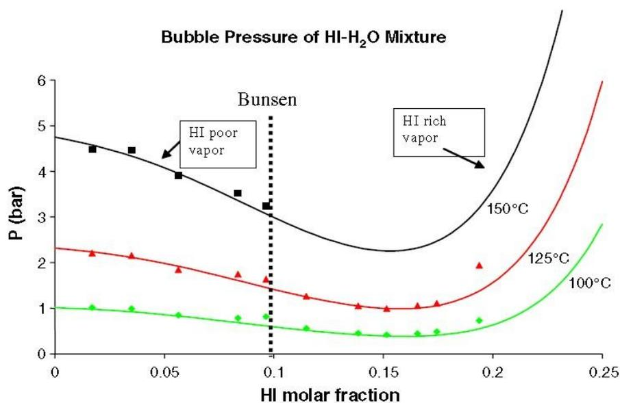
Figure 2.9: Azeotropic lines of  $\text{HI}_x$  mixture
