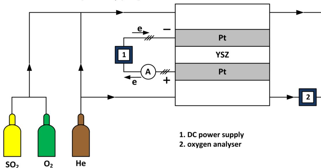
Figure 4.1: Experimental setup
