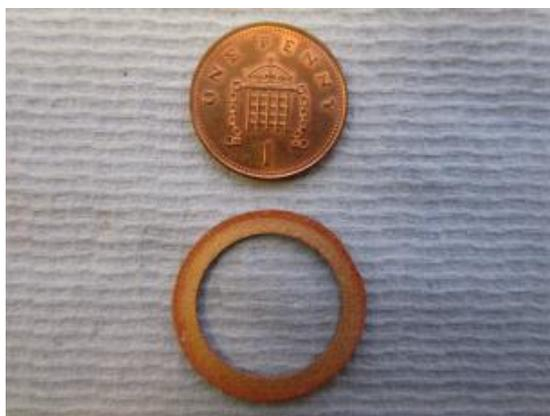
Figure 5.14: Thermoculite 866 gasket after sealing test at 850°C
