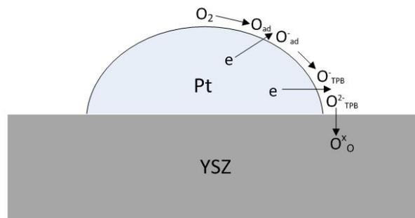
Figure 4.29: Schematic of oxygen reduction path on Pt electrode
