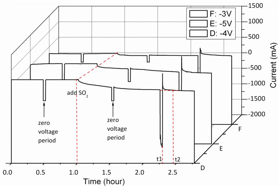
Figure 4.13: Current change of Pt/8YSZ/Pt membrane pellet exposed to  $\text{SO}_2\text{-O}_2$  at  $850^\circ\text{C}$ , with different negative voltage pulses
