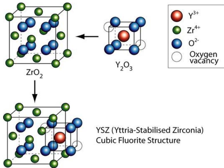
Figure 2.13: How the oxygen vacancy produces
