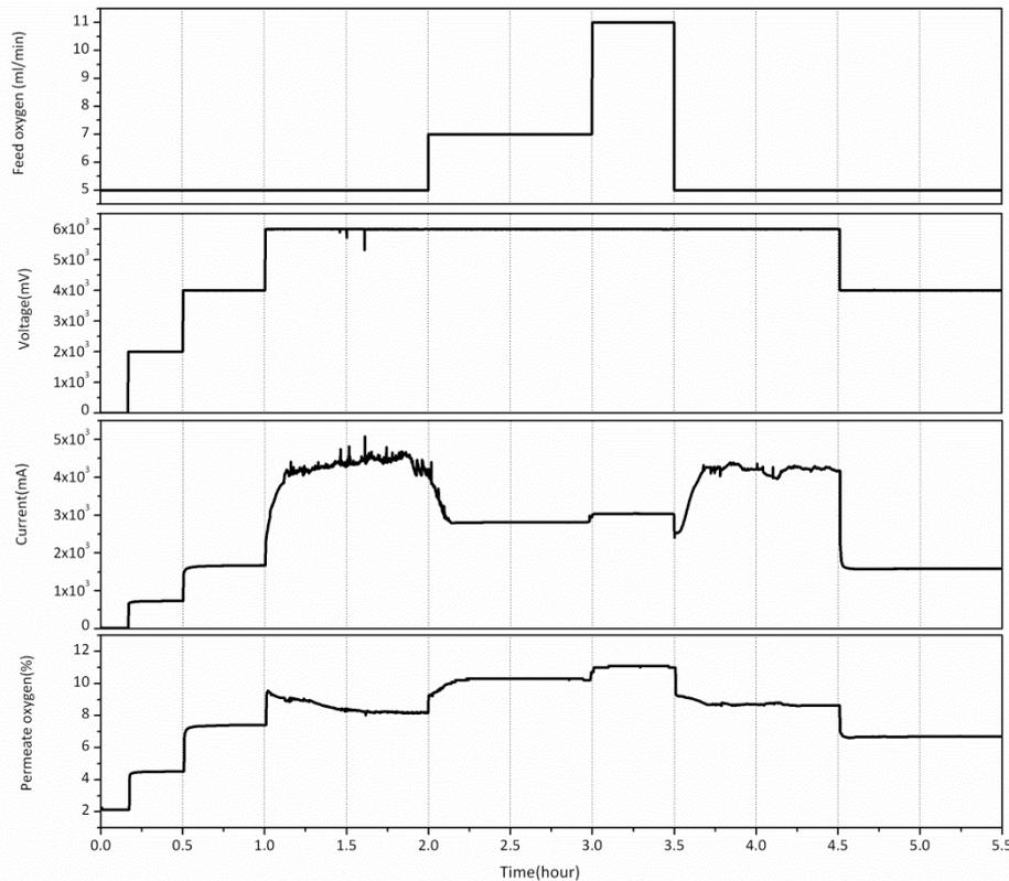
Figure 4.30: Current and permeate oxygen concentration with external DC voltage and oxygen in feed, Pt/8YSZ/Pt at 850°C
