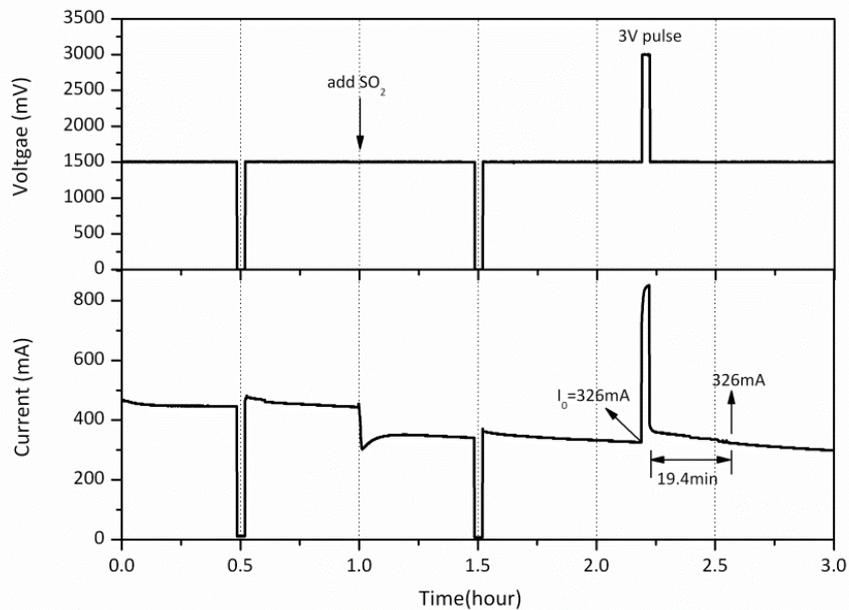
Figure 4.15: Experimental data for YSZ/Pt pellet exposure to  $SO_2$  and  $O_2$  at  $850^\circ C$  with a 2-minute 3V positive pulse treatment
