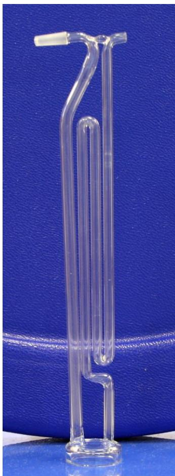
Figure 3.7: Quartz membrane holder for oxygen permeation experiment
