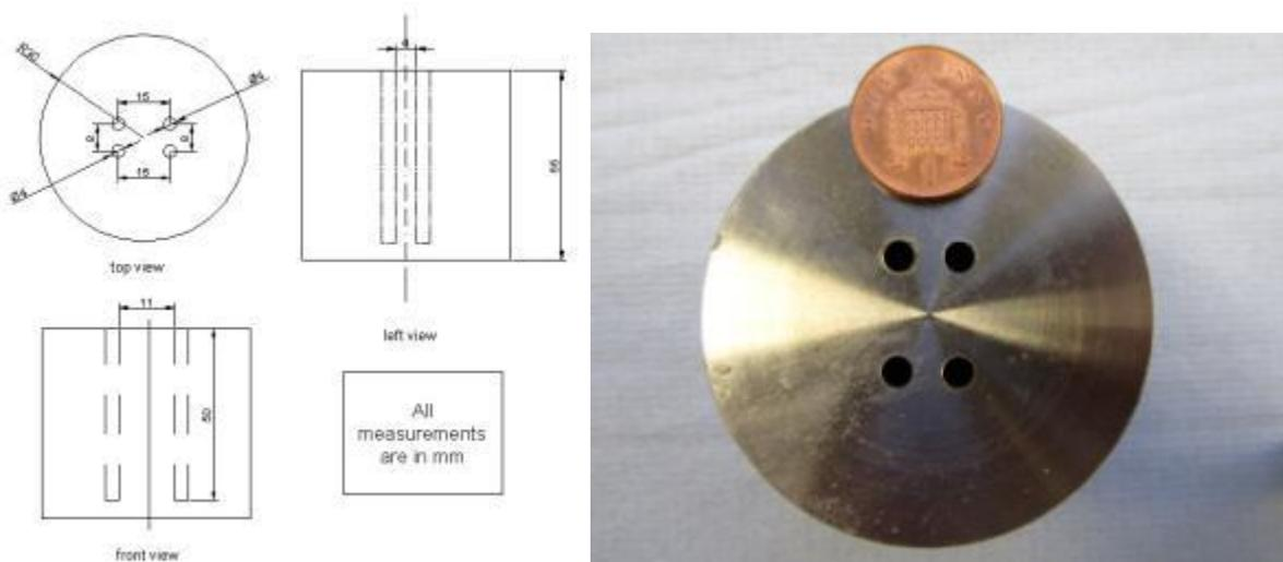
Figure 5.7: Schematic design and fabrication of the top weight
