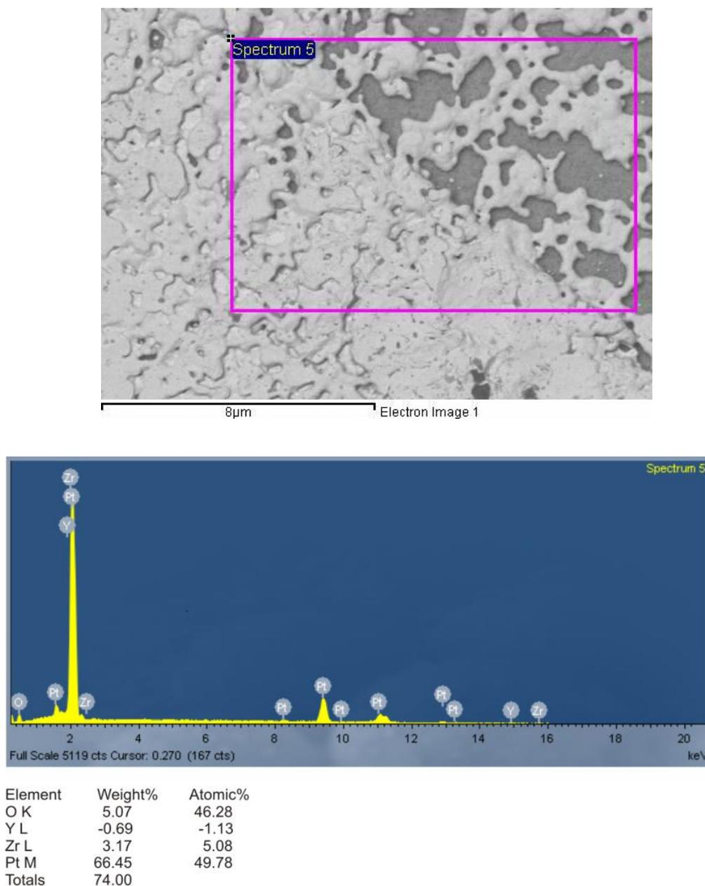
Figure 4.7: SEM-EDS spectra of the cathode surface for the YSZ/Pt pellet after 4V pulse treatment, Pt/YSZ area
