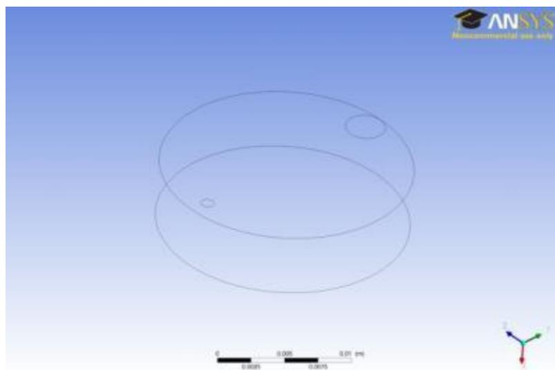
Figure 5.24: Outline of flow domain for FLUENT simulations. The smaller hole is the flow inlet and the larger hole is the flow outlet.
