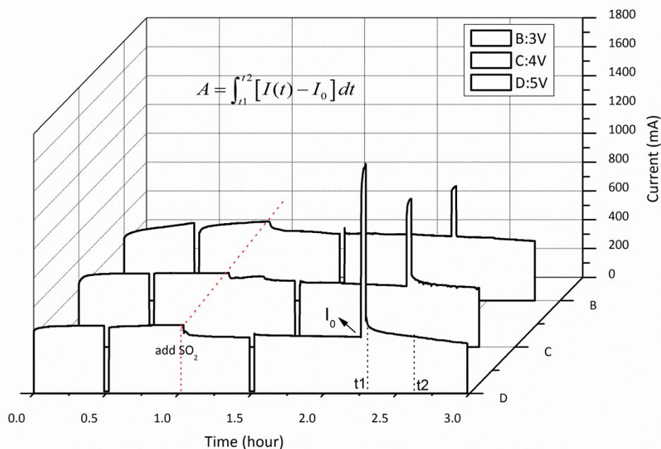
Figure 4.11: Current change of Pt/8YSZ/Pt membrane pellet exposed to SO<sub>2</sub>-O<sub>2</sub> at 850°C, with different positive voltage pulses
