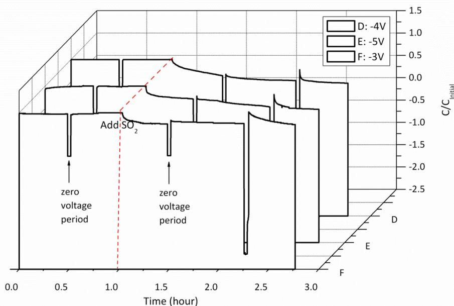
Figure 4.14: Performance change after current normalization of Pt/8YSZ/Pt membrane pellet exposed to  $\text{SO}_2\text{-O}_2$  at  $850^\circ\text{C}$ , with different negative voltage pulses
