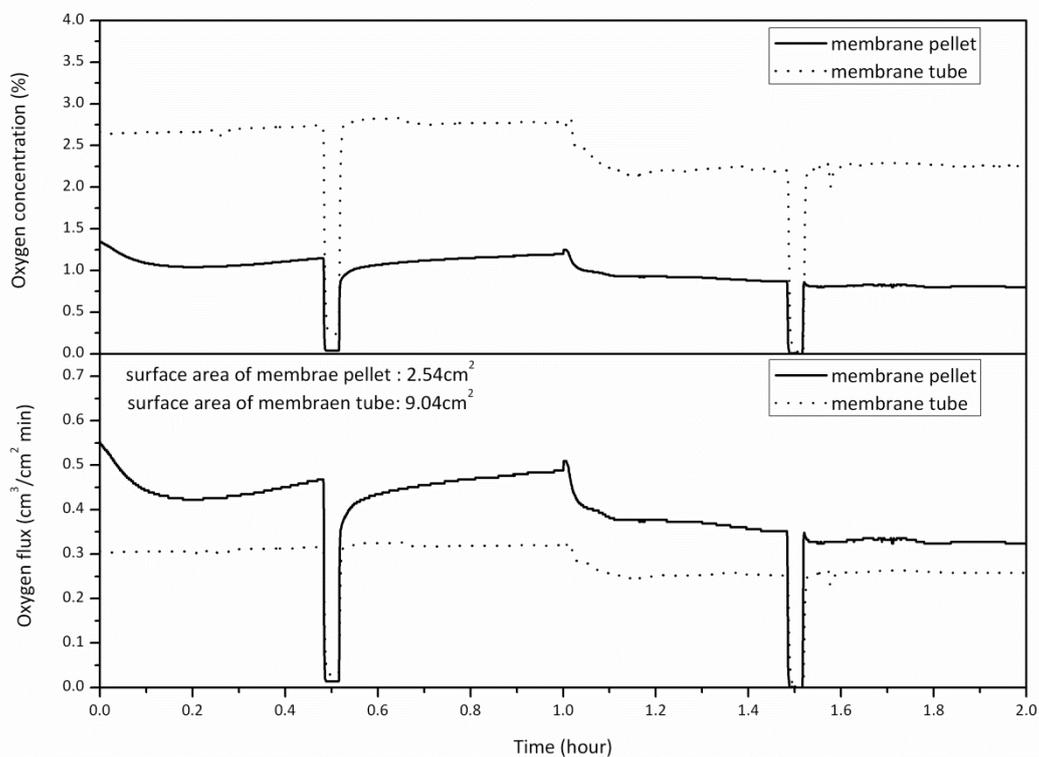
Figure 5.22: Oxygen permeation flux of membrane pellet and membrane tube
