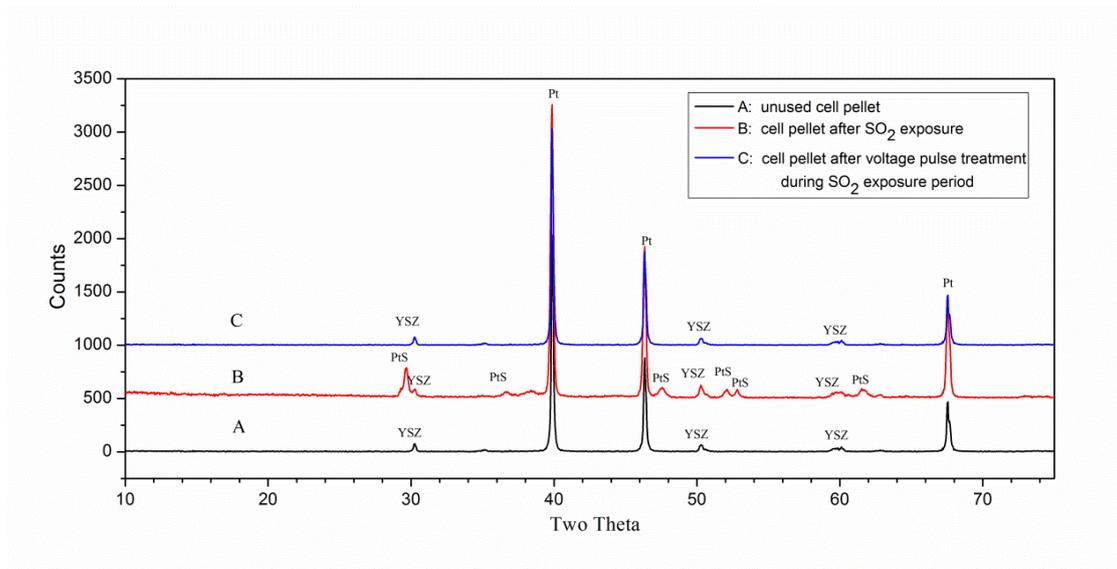
Figure 4.3: XRD data for the cathode side of YSZ/Pt pellet after 4V pulse treatment
