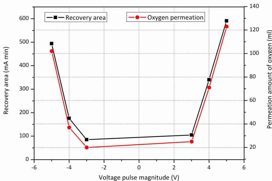
Figure 4.16: Performance recovery of membrane achieved by different voltage pulse
