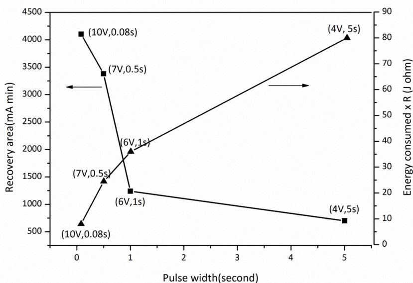
Figure 4.28: Membrane performance recovery and energy consumed of optimum voltage pulses
