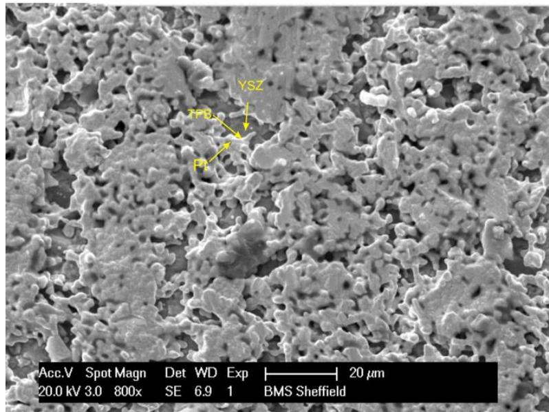
Figure 3.4: SEM image of a Pt/8YSZ membrane pellet surface, the magnification is 800x
