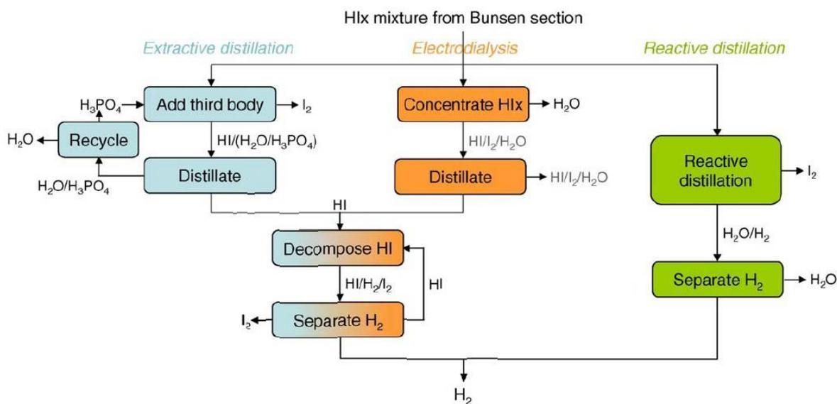
Figure 2.10: Schematic representation of the main options for the HI section (Vitart et al. 2006)
