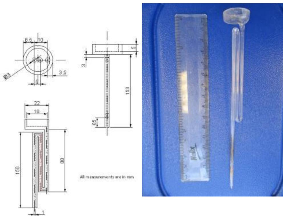
Figure 5.5: Schematic design and fabrication of pre-heating quartz tube
