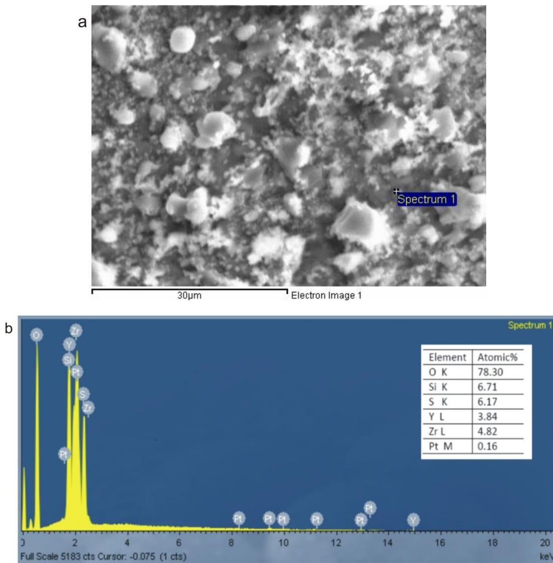
Figure 3.23: EDS elemental point analysis for a new pellet treated by  $\text{SO}_2$  exposure: SEM image (a) and EDS spectrum (b)
