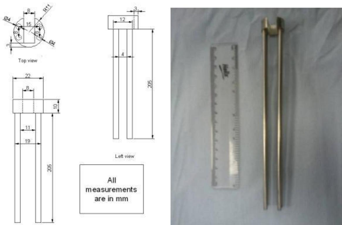
Figure 5.6: Schematic design and fabrication of the support
