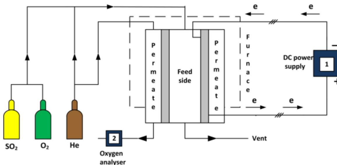
Figure 5.4: Schematic of membrane tubular separation process
