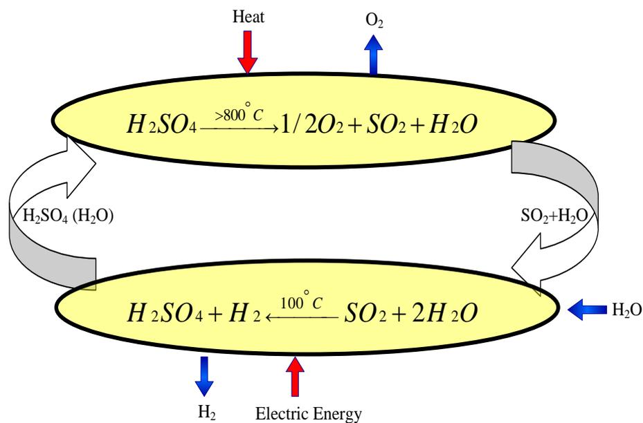
Figure 2.7: *The hybrid sulphur process scheme*
