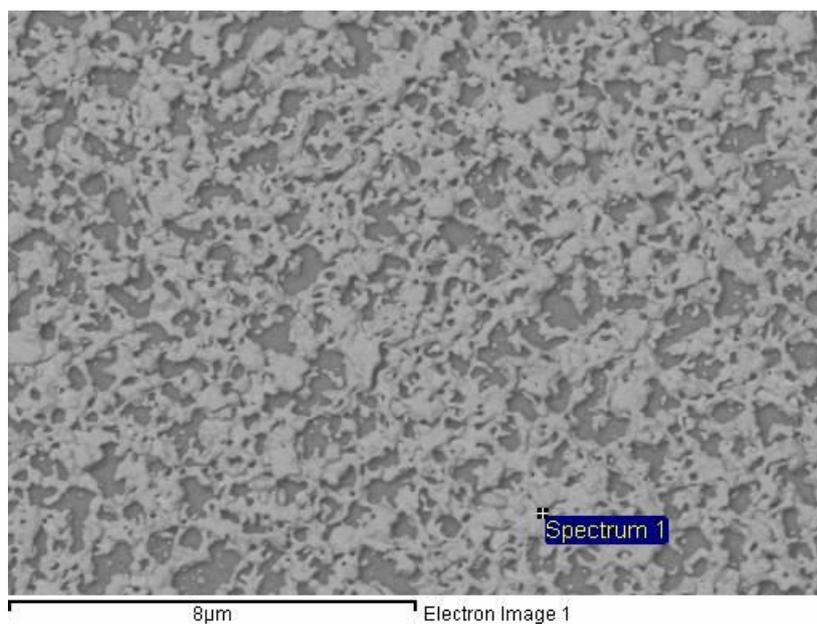
Figure 3.16: SEM image of a fresh Pt/8YSZ pellet
