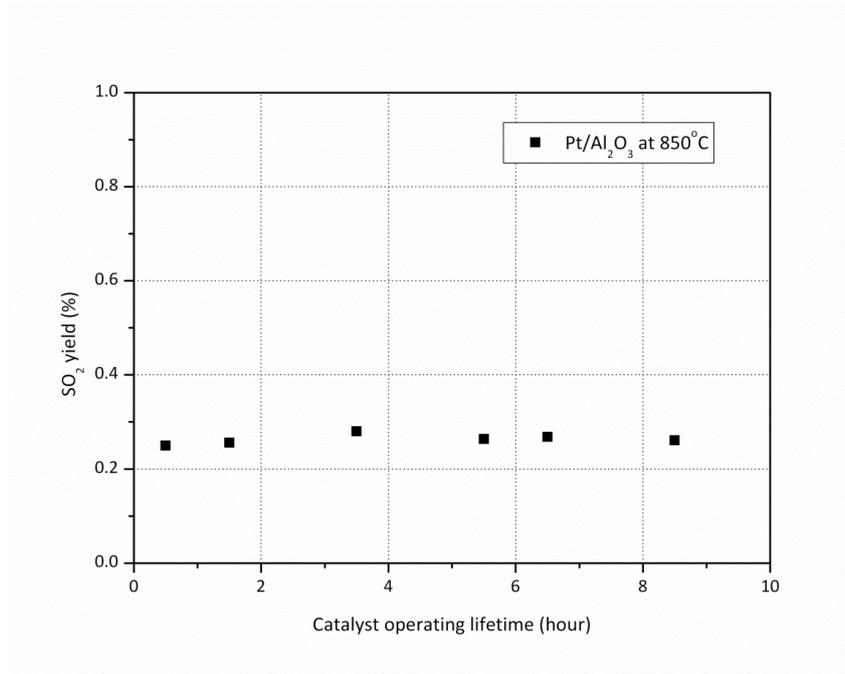
Figure 6.12:  $Pt/Al_2O_3$  catalyst activity based on  $SO_2$  yield as a function of the catalyst operating lifetime (Section III)
