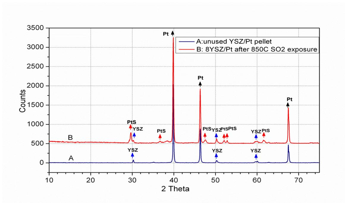
Figure 3.24: Before and after XRD data for 8YSZ/Pt membrane at 850°C SO<sub>2</sub> exposure, feed side
