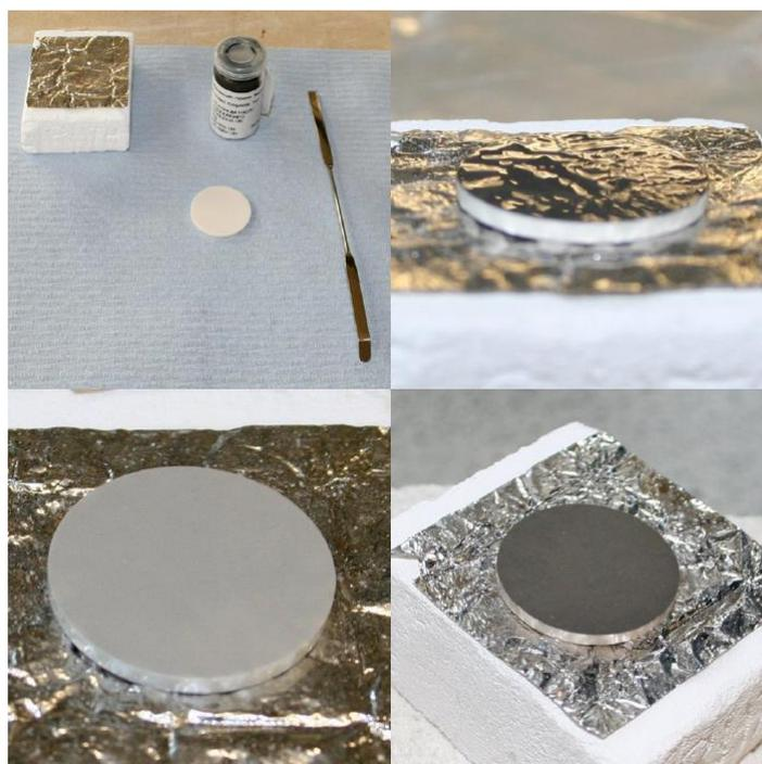
Figure 2.14: *Photo mosaic of platinum electrode application process.*
