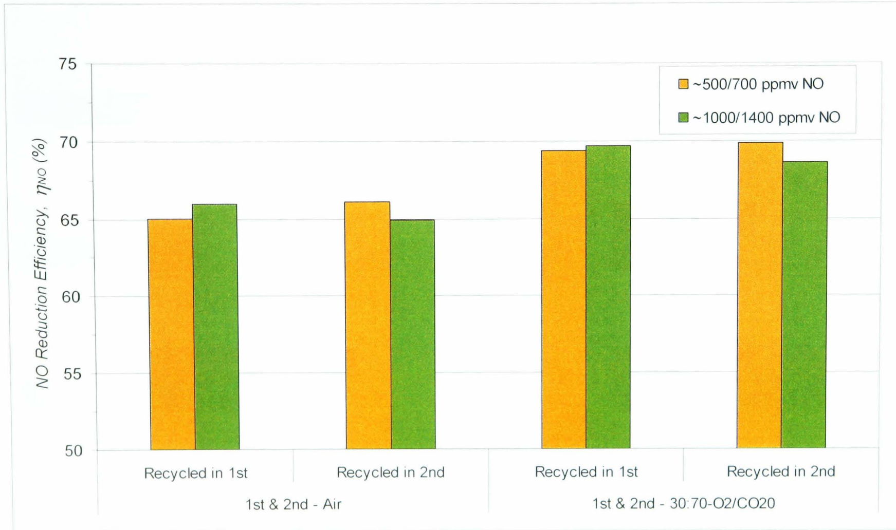
Figure 4.32a. The effect recycled NO concentrations on NO Reduction Efficiency ( \eta_{NO} ). (Unstaged, SR=1.20, Coal A).
