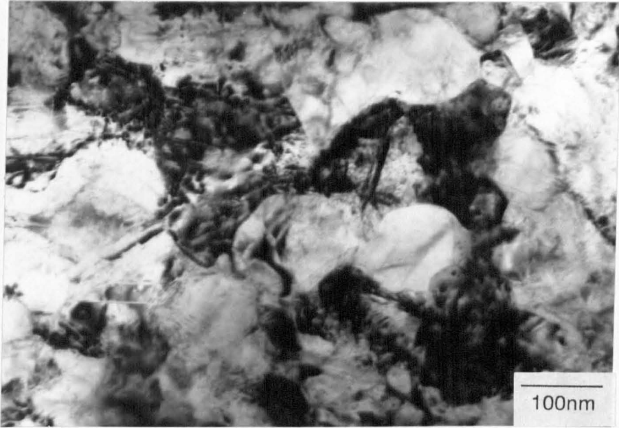
Fig. 5.65. TEM micrograph of the extruded debris showing grains which may have undergone dynamic recrystallisation.
