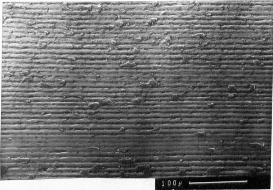
Fig. 6.66. Optical micrograph (Nomarski) showing abrasive grooves and evidence of chattering. (59 N/pin 3Y).
