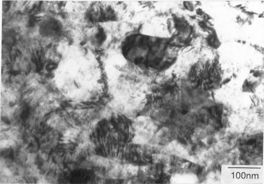
Fig. 5.62. TEM micrograph showing an occasional crystallite which appears equiaxed. This was not as a result of dynamic recrystallisation.
