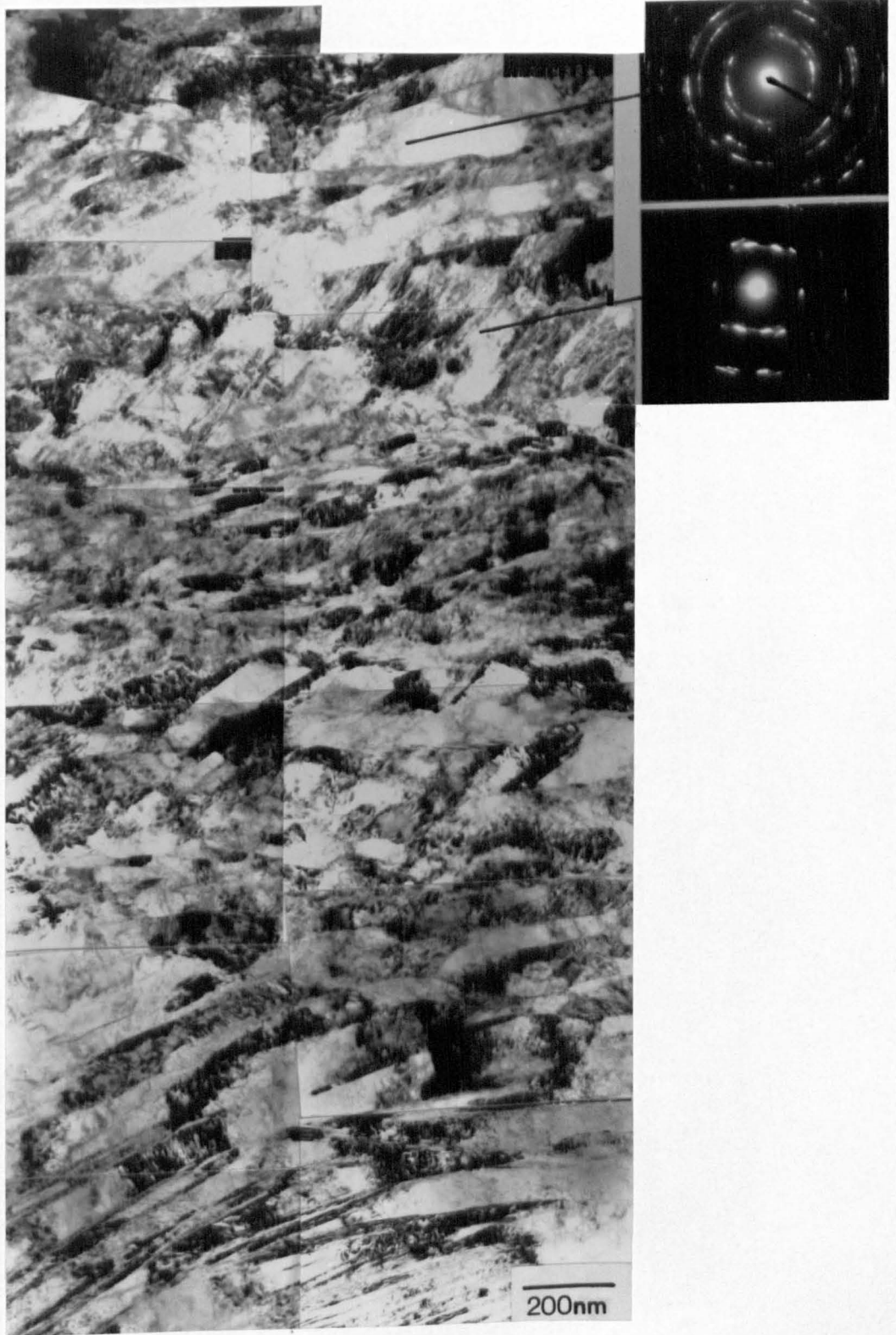
Fig. 5.41. Composite TEM micrograph showing the typical structure of the transition region. The different regions of twins and shear bands can only be clearly differentiated by the diffraction patterns. A schematic is provided on the facing page.
