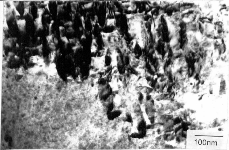
Fig. 6.15. Back-thinned TEM micrograph of the surface of the Mg-PSZ disc. The outer region is the non equilibrium oxide described in chapter 5. Note how the centre consists mainly of precipitates, with a diffuse boundary between the metal oxide and the zirconia. Very little cubic could be imaged in the dark field mode suggesting it has been preferentially eroded. The precipitates are monoclinic even though no twin boundaries could be imaged. (24 N/pin).
