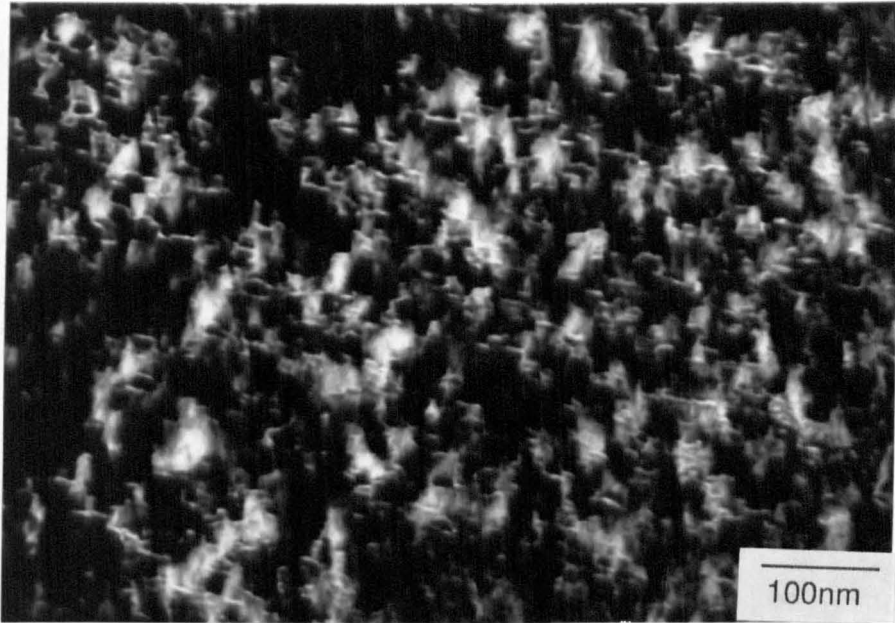
Fig. 3.14. Dark field micrograph showing very fine tetragonal precipitates produced by a rapid cool from sintering (after Rainforth & Nettleship [272]).
