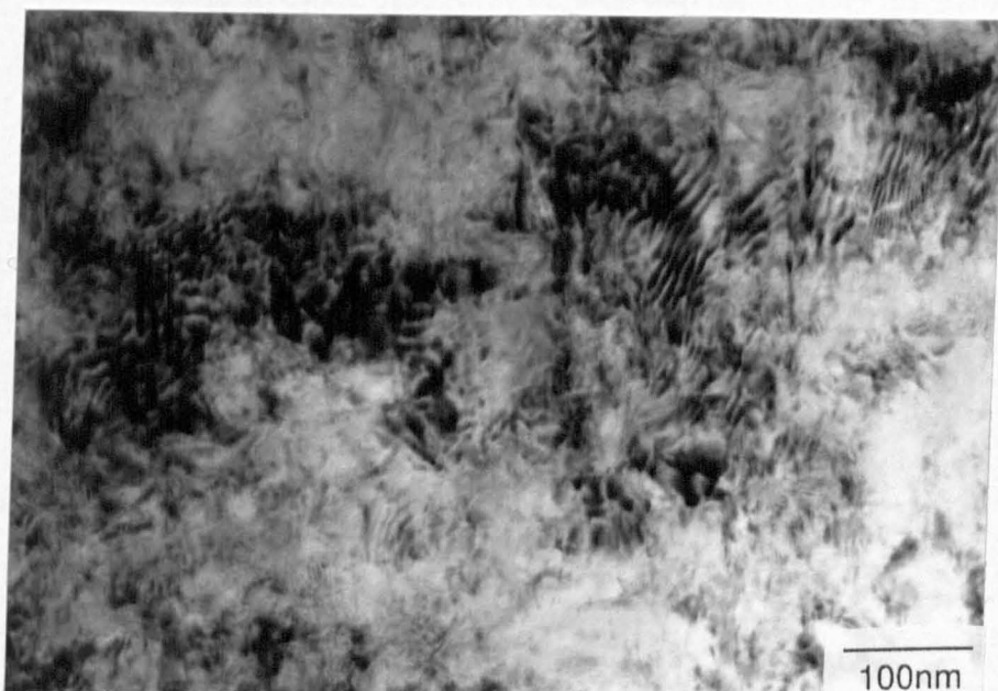
Fig. 6.41. Detail from the groove in fig 6.38 of a region which contained no grain boundaries or monoclinic. Some tetragonal is still present. The structure has undergone considerable rotation compared to the parent structure.
