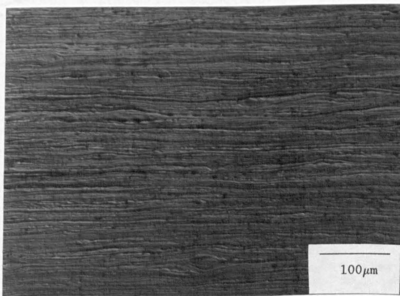
Fig. 4.5. After a reduction of 96% the majority of the structure had become aligned with the R.D. but few twin colonies remained. No macro-shear bands are present.
