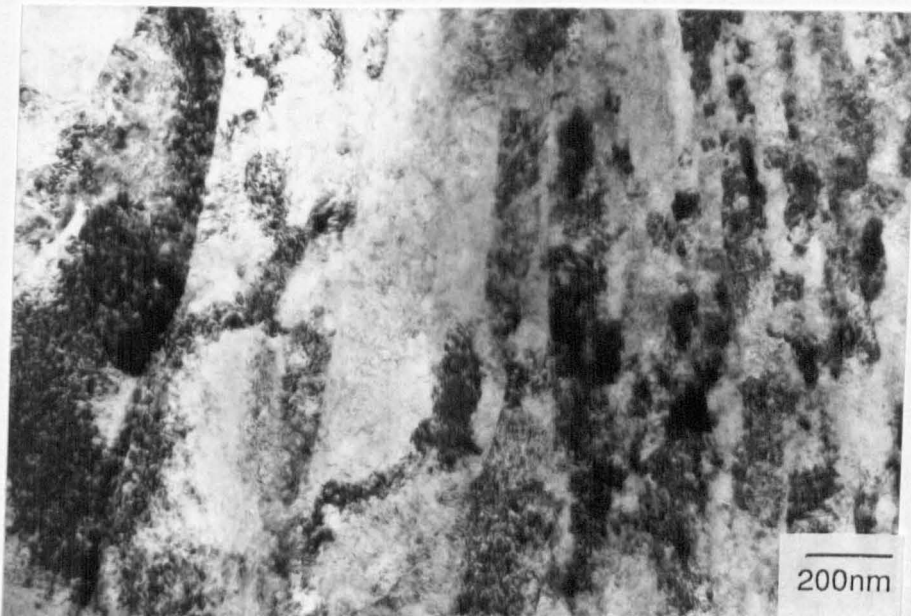
Fig.7.21. Detail of the transition from region 3 to 4. Less microcracking had occurred. The very high strain contrast made it difficult to establish the dislocation density.
