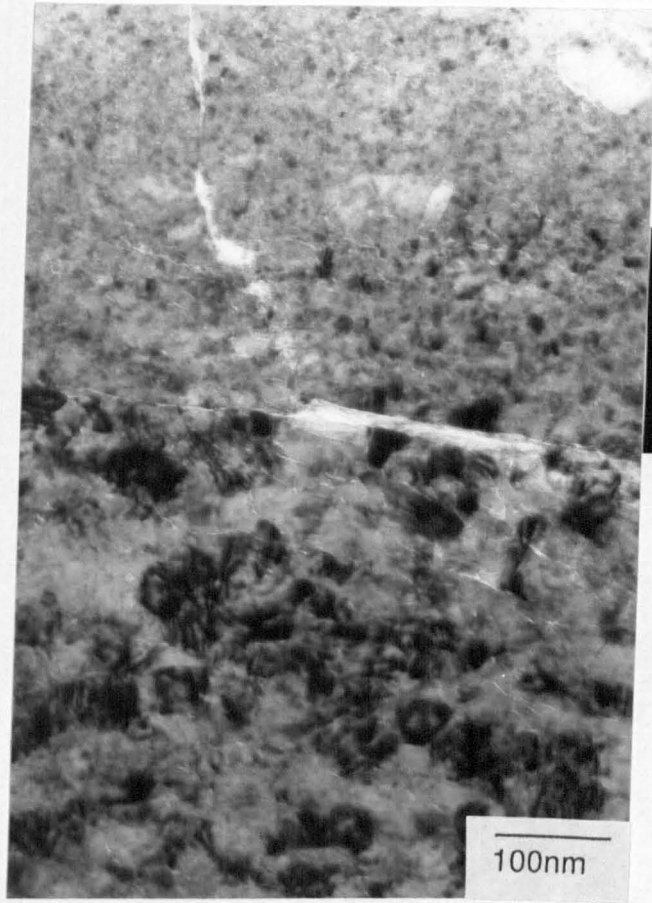
Fig. 7.15. Detail of the transition between regions 1 and 2. Note the extensive microcracking in the crystalline region and the lower portion of region 1. Some areas of region 2 were more equiaxed than this example. The average grain size in this region was about 50nm, representing an order of magnitude reduction from the starting material. Note also, the small dark particles in region 1 close to the interface. This could represent a transition from the crystalline to amorphous state. Alternatively, these could be tetragonal particles precipitated from the amorphous phase on cooling at the end of the wear test.
