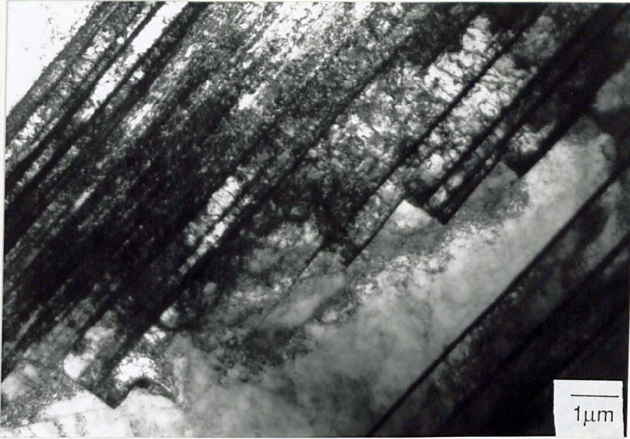
Fig. 5.36. TEM micrograph of a twin colony within a grain which is not fully twinned. Note that individual dislocations can be imaged within the twins.
