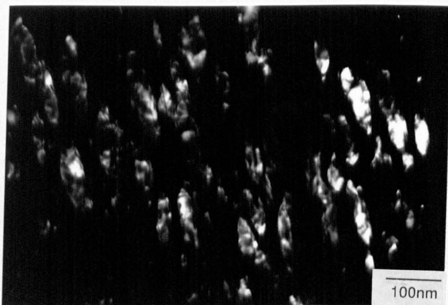
Fig. 6.19. Dark field TEM micrograph from the worn surface using the monoclinic/ tetragonal diffraction spot. Occasional twin boundaries can be seen.
