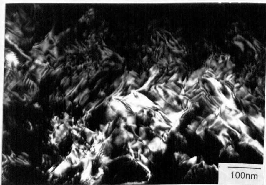
Fig 6.21. Cubic dark field image of the above. There is still considerable residual strain in the matrix induced by the wear process.
