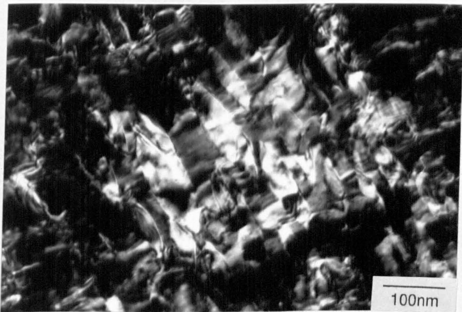
Fig. 6.44. Dark field micrograph which has included diffraction spots from the cubic matrix and the precipitates from very close to the original surface. Note the residual strains, the absence of twin boundaries and that the precipitates have retained their original shape.
