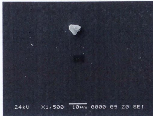
Figure 5.8: SEM observations of crystals of calcium carbonate formed under polarization conditions with 4ppm of PPCA after a 60 minute experiment
