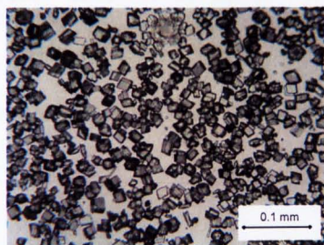
Figure 4.10: Calcium carbonate deposit obtained by electrocrystallization after 4 hours with no inhibitor
