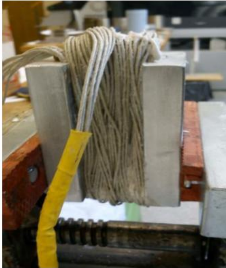
Figure 6.13: Initial winding trials with 9 parallel wires wound simultaneously.
