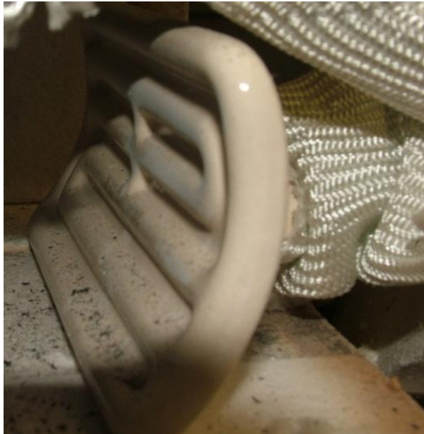
Figure 6.21: Supplementary ceramic heater used in 350°C tests.
