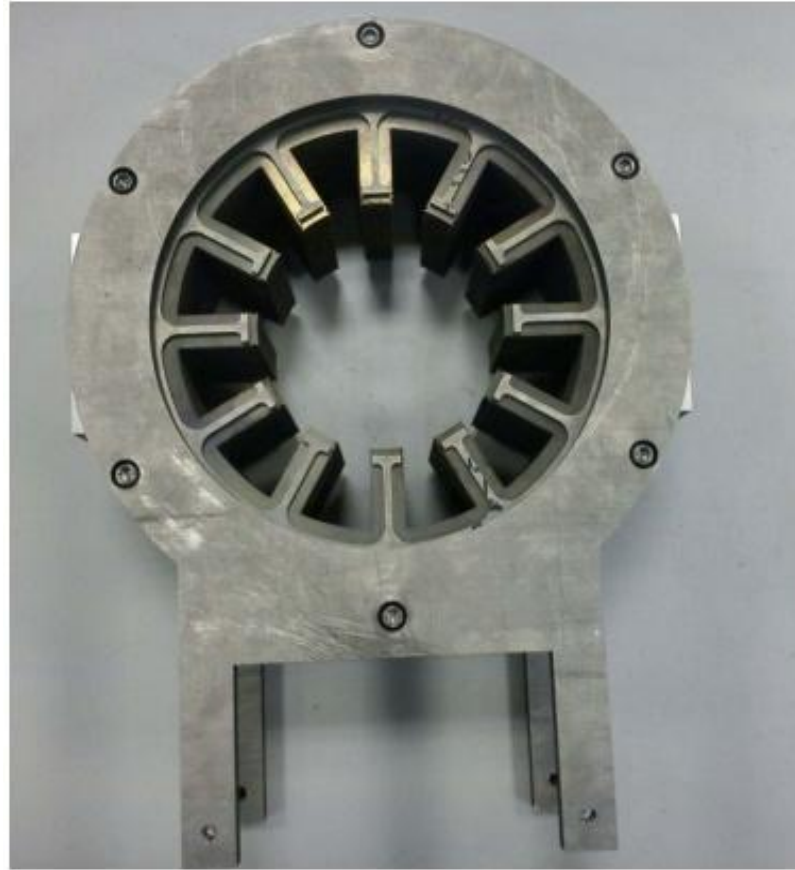
Figure 6.10: Assembled stator casing, core and Titanium clamping plates.
