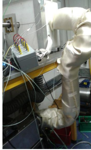
(b) Single layer of additional insulation with Silica cloth over-wrap
