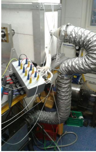
(a) Flexible duct with no insulation
