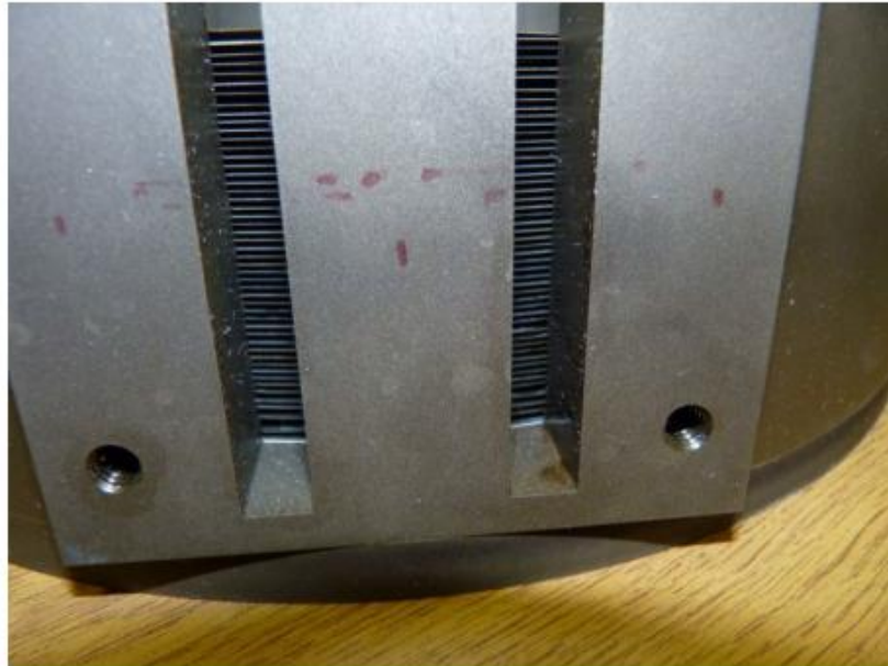
Figure F.5: Close up of cooling apertures illustrating the cooling channels realised in the stator core.
