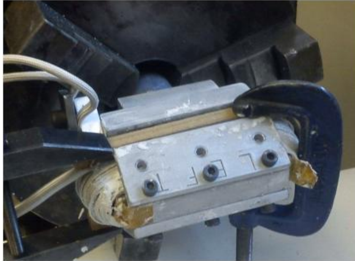
Figure 6.12: Wound coil clamped in jig during curing of the encapsulant.
