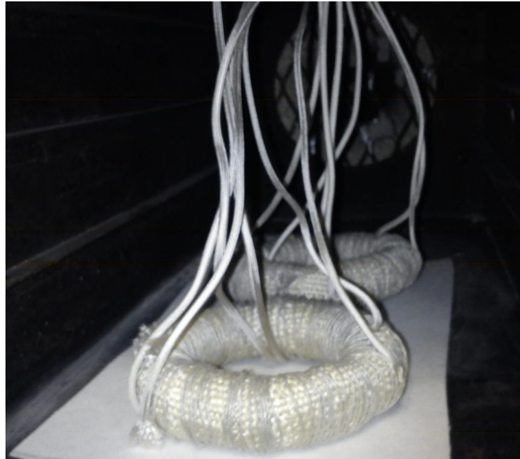
Figure 4.2: Prepared core samples placed in a high temperature oven.
