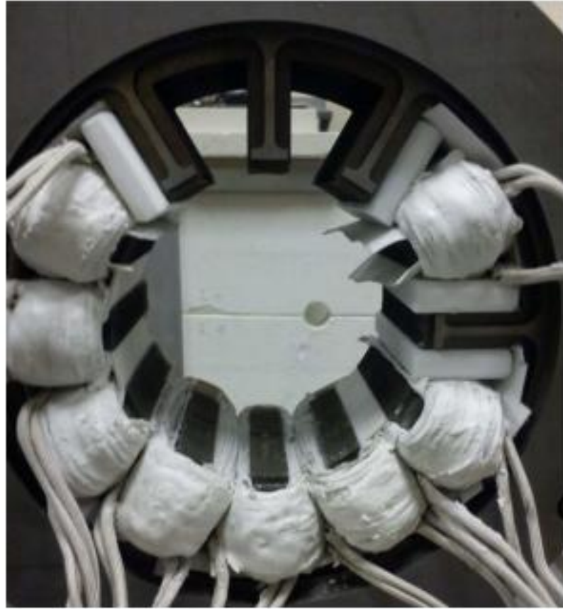
Figure 6.15: Part populated stator core illustrating the PTFE wedges employed to retain coil geometry during final cure.
