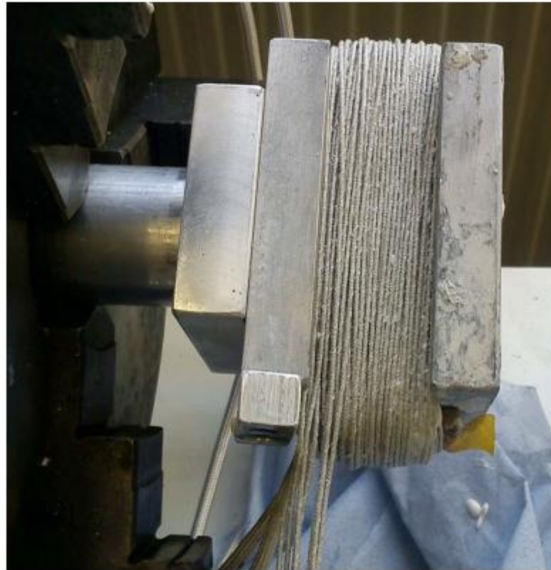
Figure 6.14: Coil part-way through manufacture based on winding with two sets of 4 parallel strands.
