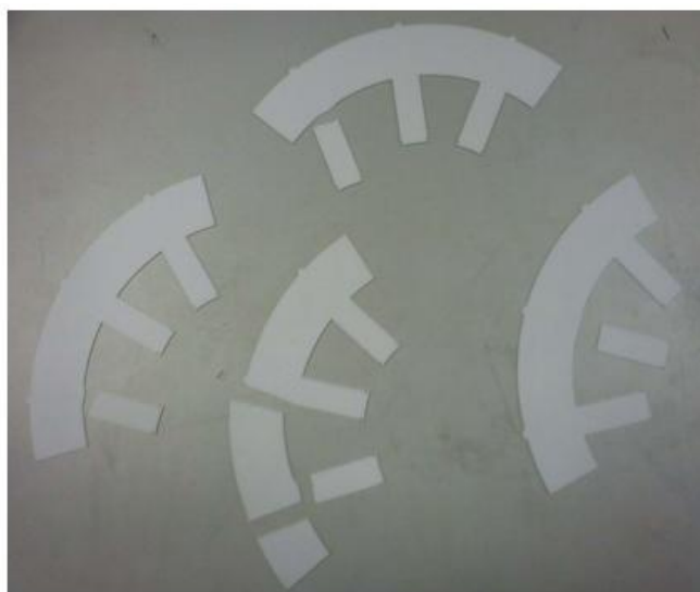
Figure F.9: Failed Alumina clamping plates.
