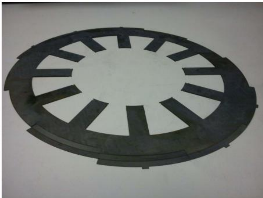
Figure F.2: Indexing of laminations along length to form the stator core.
