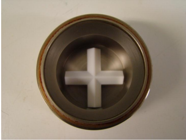
Figure 2.1 – 49 cm 3 stainless steel reactor with magnetic stirrer.
