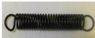
Figure 5.15: Picture of the short spring fabricated to form part of the vertical tensile structural member
