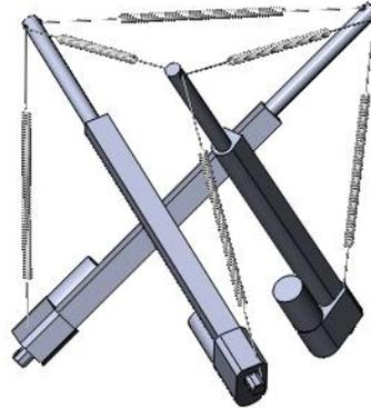
Figure 5.8: SolidWorks® dimensional drawing of the 3-bar tensegrity prism with cables approximated by elastic springs and the three bottom nodes rigidly attached to the base
