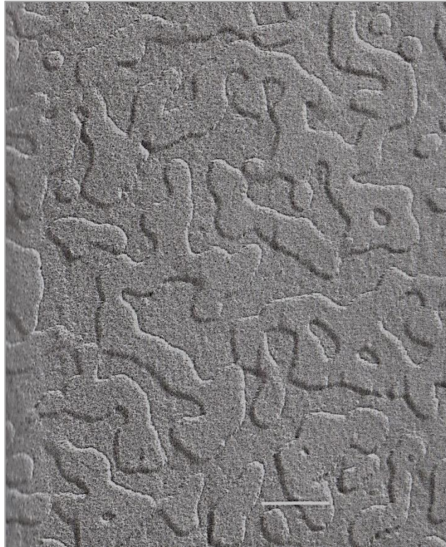
Figure 2.7: Micrograph of spinodal decomposition with an interconnected morphology [62].
