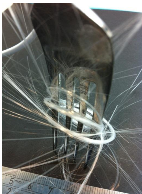
Figure 5.21: Bent LAS glass fibres with a mean diameter of 50 \mu m.
