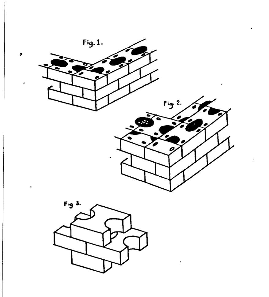
Figure 9.10. Beedle and Rogers ventilating bricks.
