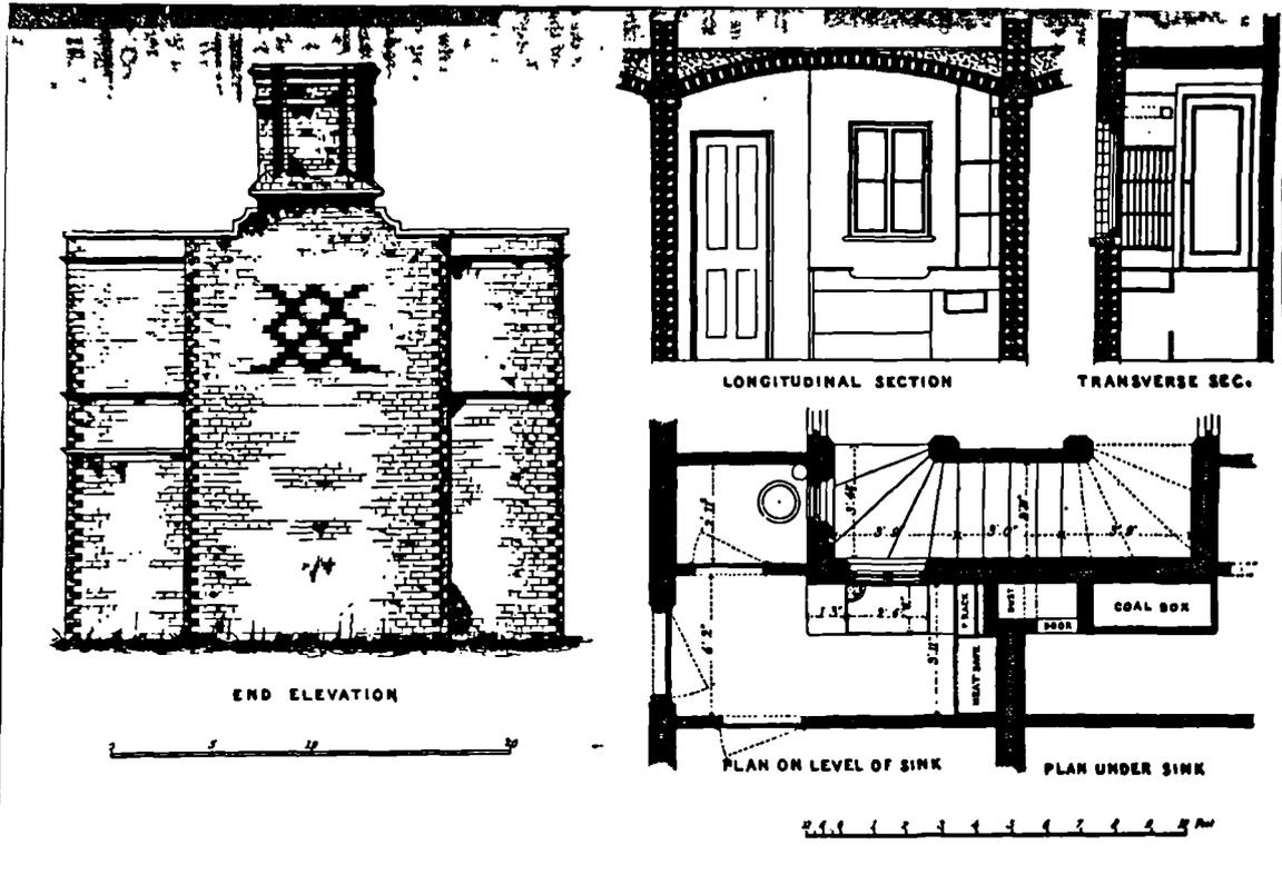
Figure 10.4. Prince Albert's Model Houses for Families at the Great Exhibition, 1851; end elevation, longitudinal and transverse sections, and detailed plan around common stair. [From James Steven Curl, The Life and Work of Henry Roberts, 1803-1876 (1983) p. 95]
