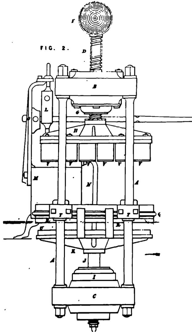
Figure 4.8. Hydraulic brick press by William Mencke, British Patent No. 5681, 1828. [Drawing enrolled with patent]
