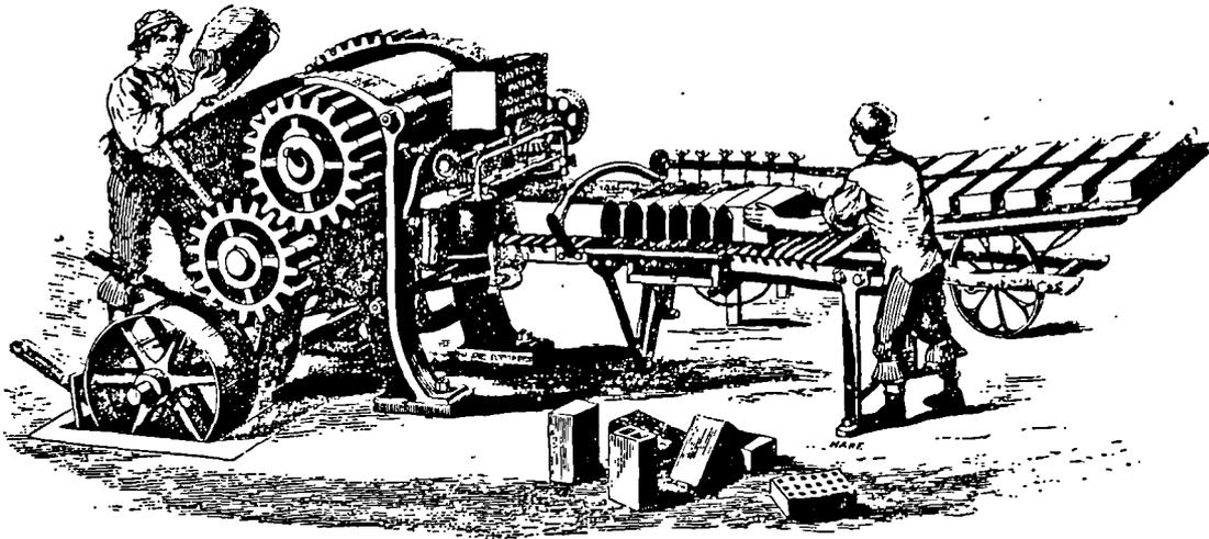
Figure 7.7. Henry Clayton's One-Process Brickmaking Machine.
