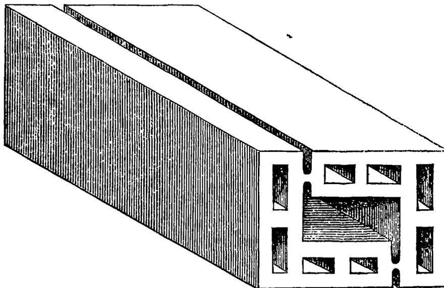
Figure 11.10. Perforated facing blocks introduced by John Taylor, c. 1863.
