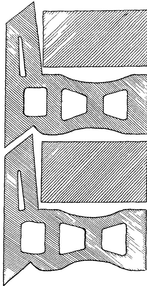
Figure 11.9. Interlocking facing bricks patented by W. Walton,
