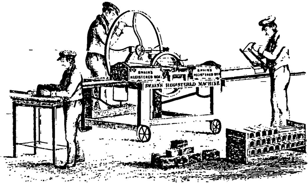
Figure 5.11. "Swain's Registered Pipe and Tile Machine", c. 1847.
