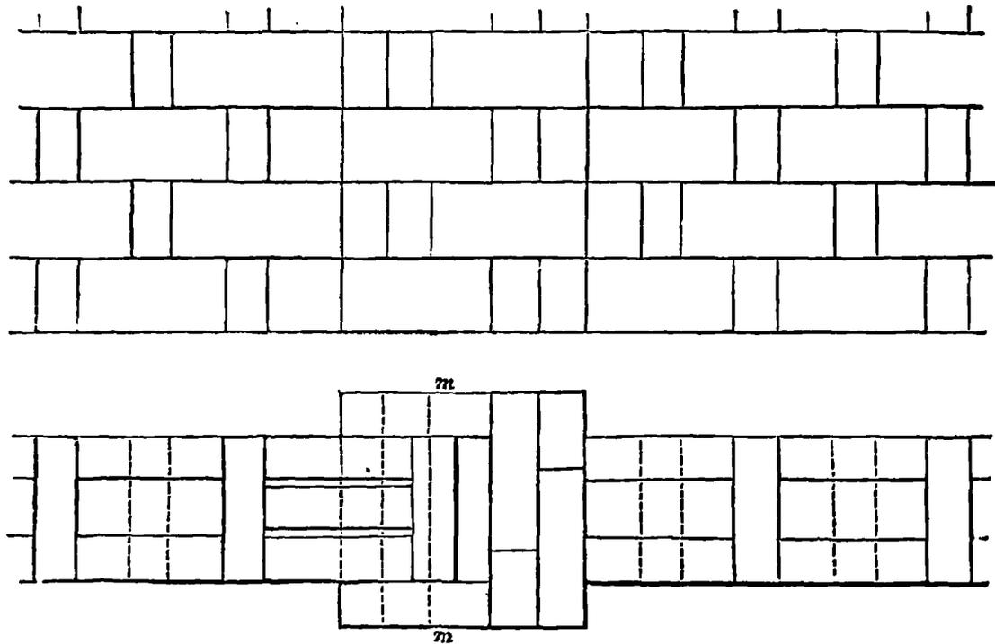
Figure 11.2. Plan and elevation of Silverlock's hollow walls.
