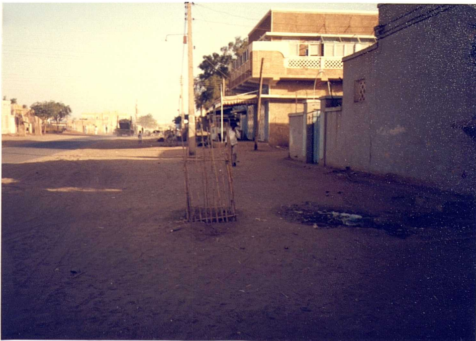
PLATE (7.11): Adjustable timber units added to the original balcony wall to make it as, approximately, high as 2ms. Would the architects consider the popular convention or would they insist on applying not matching elements to the perceived privacy.
