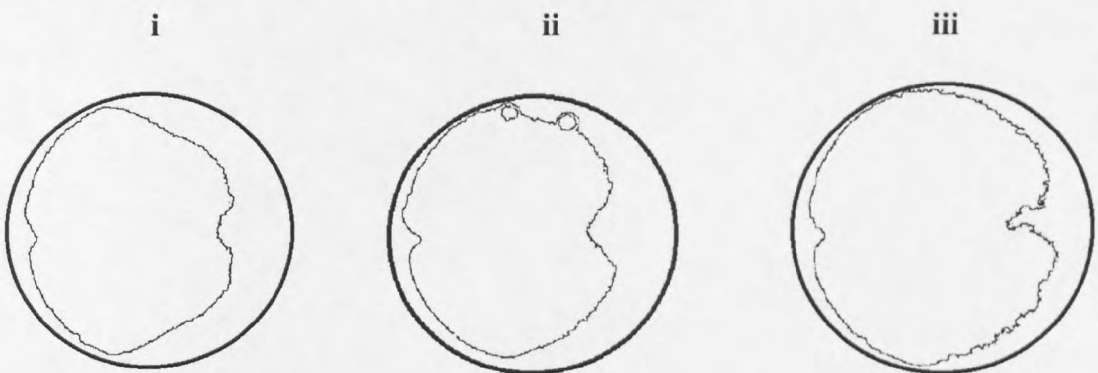
Figure 5.18 (b) Spark-ignition of n-pentane at tdc following compression to 875 K. Frames at (i) 2.2 ms, (ii) 2.4 ms and (iii) 2.6 ms after the spark initiation.
