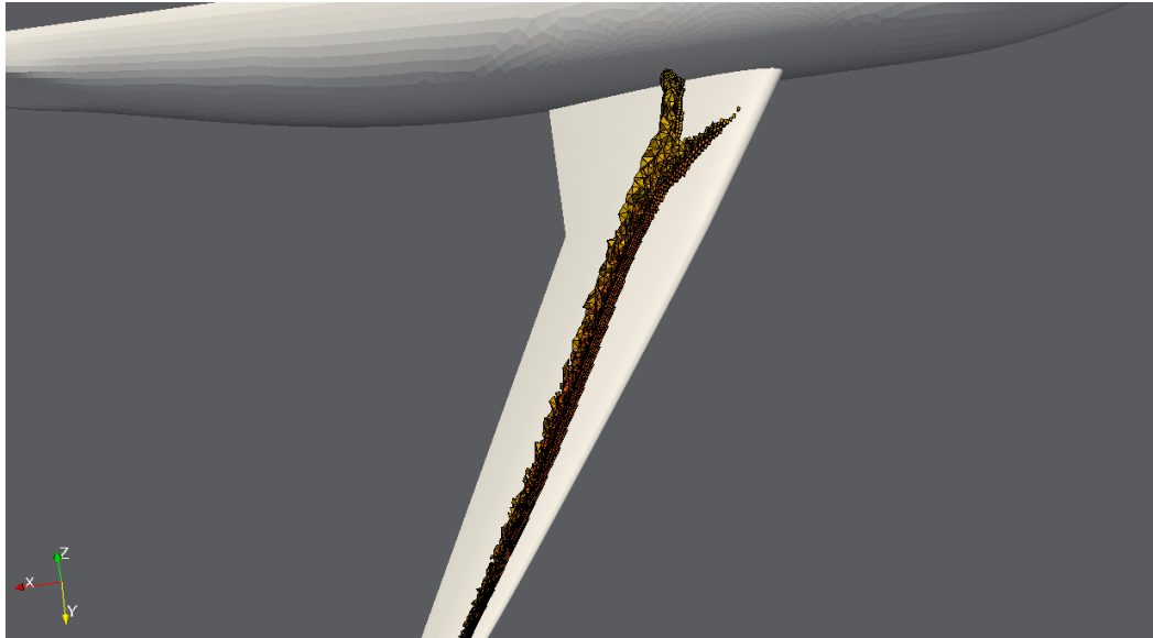
Figure 5.24: Extracted shock structure
