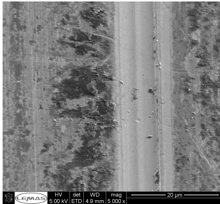
Figure 5.23: High magnification image showing surface deposits after testing in NaCl(aq) at 1Hz for a sliding distance of 216m.
