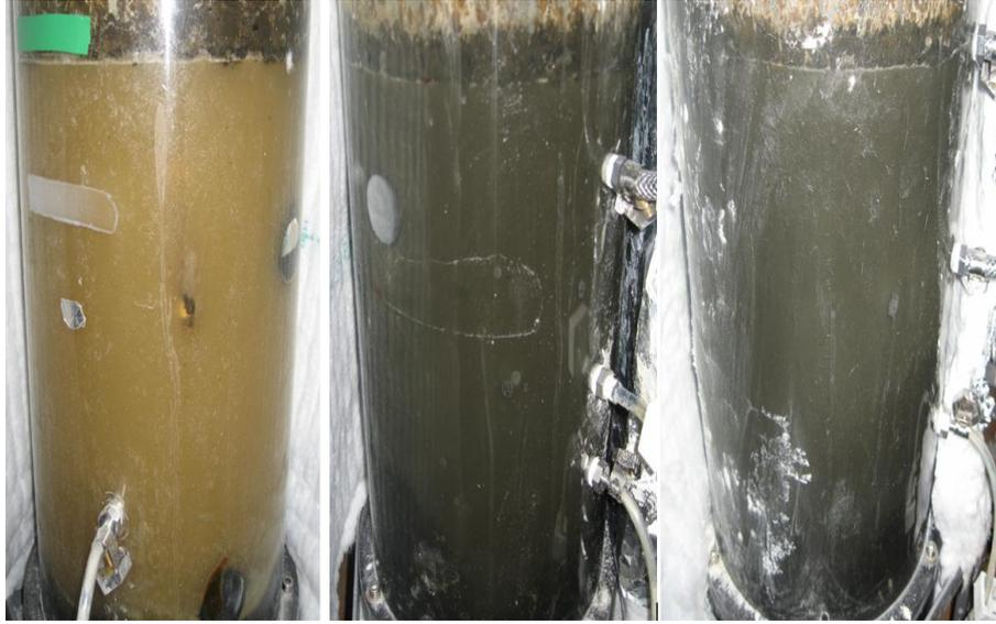
Figure 3.25: Snapshot of the digesters in the experiments showing the dilution in the unsparged digester (light colour on left picture), while the sludge in the other digesters (middle and right) is thicker (dark colour)
