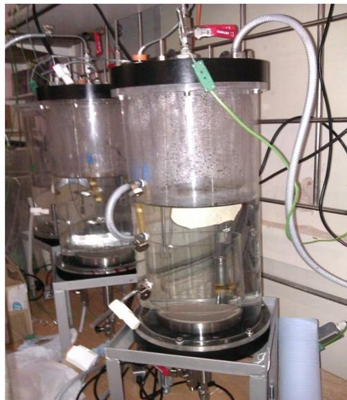
Figure 5.21 Actual airlift bioreactor modelled in this study and used in the current experiments
