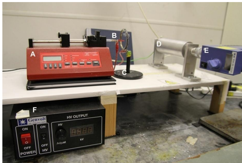
Figure 5: Electrospinning setup used for fabrication of aligned PCL microfibres. (A) Syringe pump. (B) Blunt needle connected to an electrode. (C) Focusing ring. (D) Electrically grounded cylindrical collector. (E) Electric motor. (F) Voltage generator.
