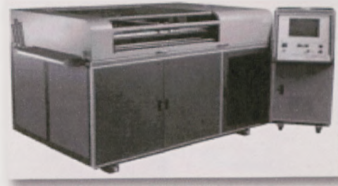
Figure 1.5 Layer Object Manufacturing system, Helisys Inc.
