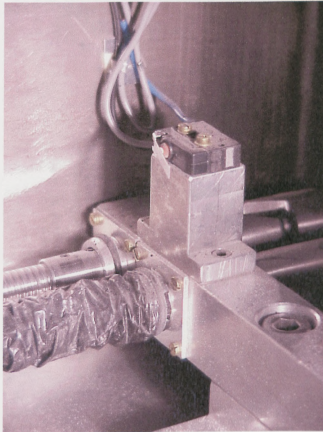
Figure 2.19 Security switches – turns the power off
