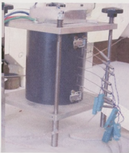
Figure 2.11 Thermal conductivity rig
