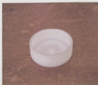
Figure 2.9 Machined nylon cup
