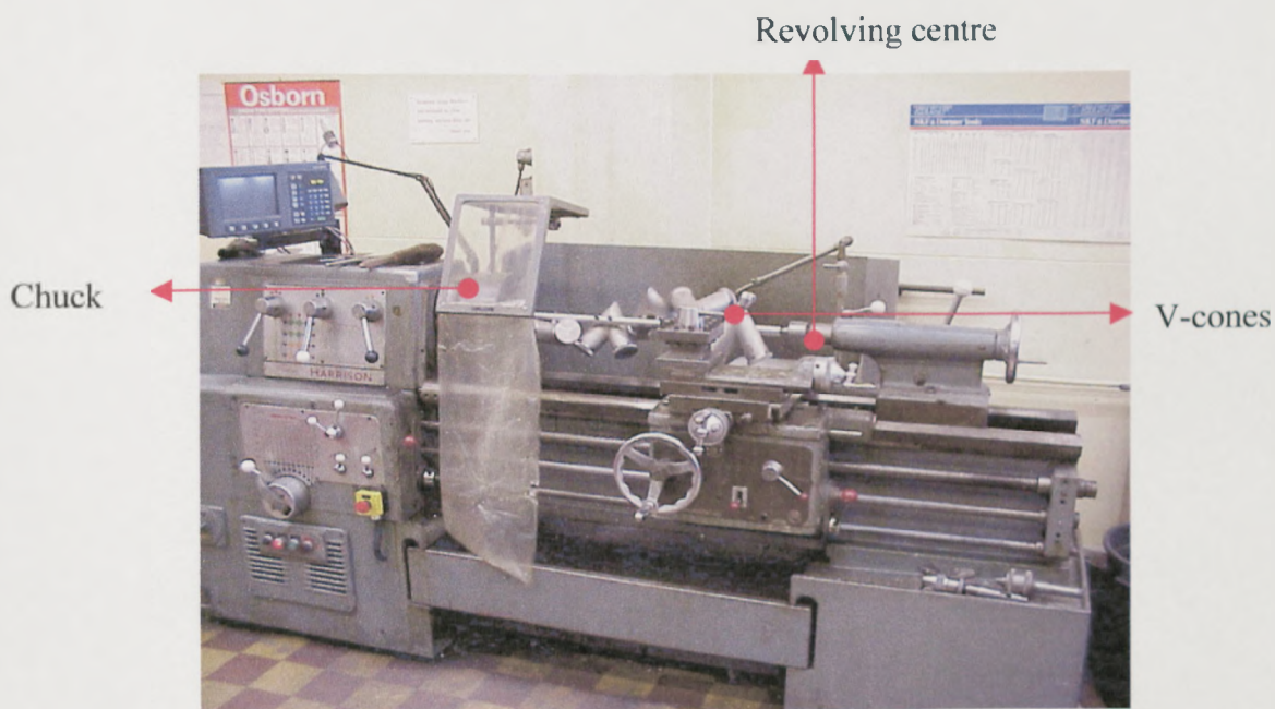
Figure 2.4 V-cones mixer assembly used for powder mixing
