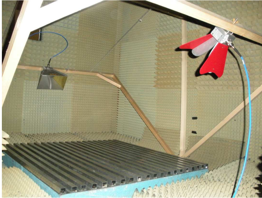
FIGURE 5.3: Measurement setup where both antennas are placed at 40 degrees.
