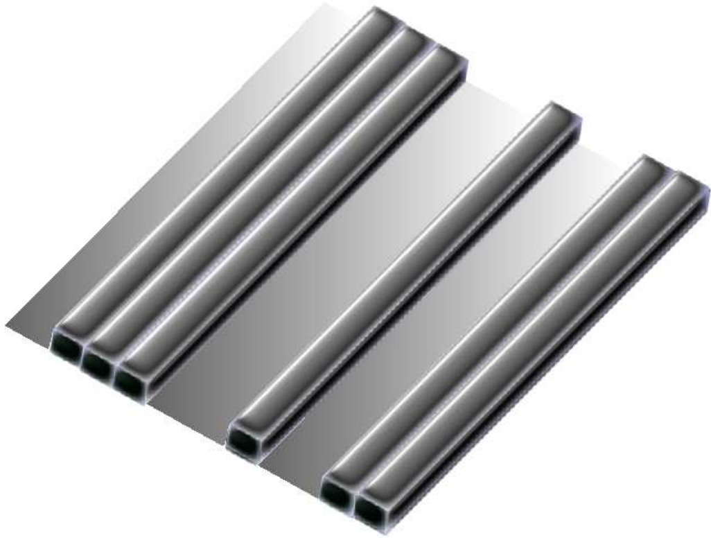
FIGURE 3.2: One period example of a maximum length diffuser according to the sequence s = [-1 +1 +1 +1 -1 -1 -1 +1 -1 -1 +1 +1] .
