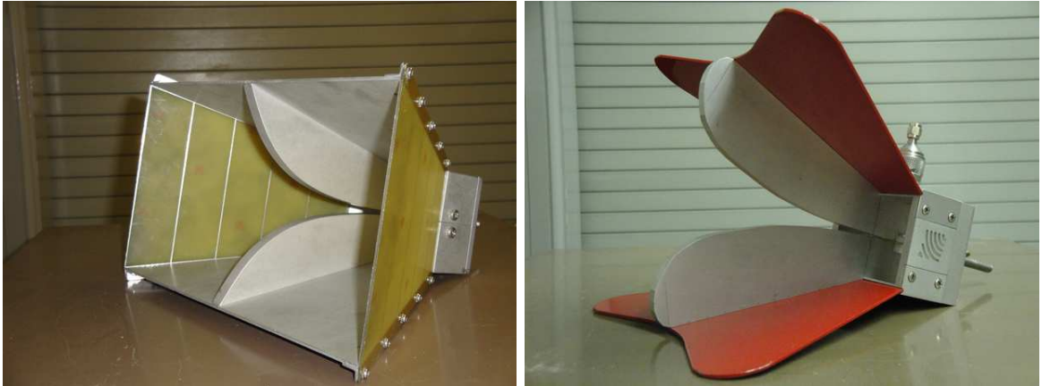
FIGURE 4.1: The double ridged waveguide horn antennas that were used in the anechoic chamber. The left figure shows the transmitter and the right one the receiver.
