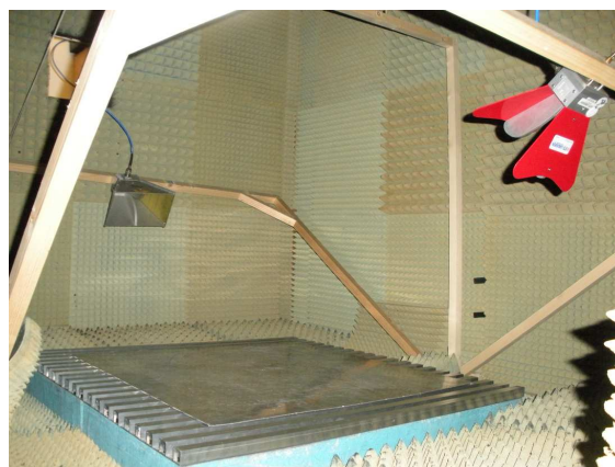
(c) Placing a plane reflector on the diffusers to measure the reflected signal.
