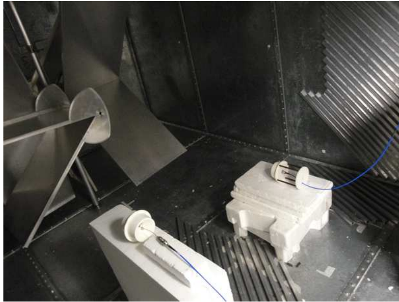
FIGURE 5.11: Image of the Reverberation Chamber Interior showing antenna and diffuser placement. The transmitter is placed at 0.5m and the receiver at 1.0m. The diffusers are placed at 45 degrees orientation. Their placement on the far wall and floor of the enclosure centered on the specular reflection points for the antenna is visible.
