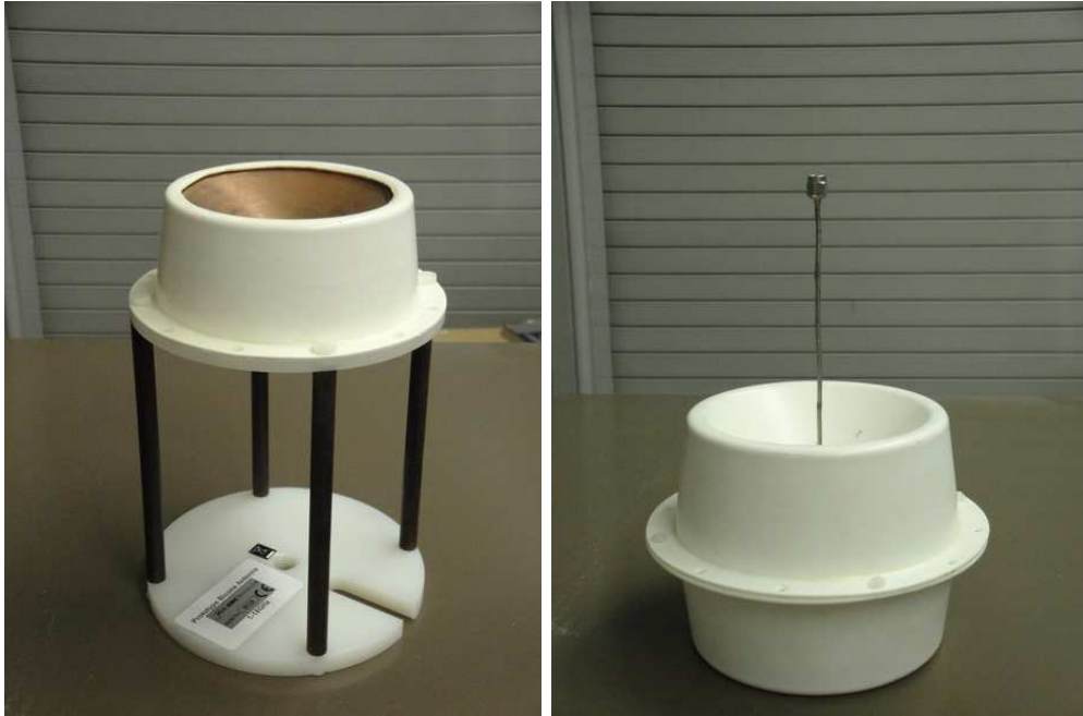
FIGURE 4.4: The omni-directional circular biconical antennas that were used in the reverberation chamber. The left figure shows the transmitter and the right one the receiver.
