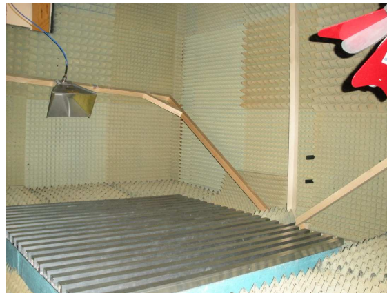
(b) Placing the diffusers on the floor to measure the reflected signal.
