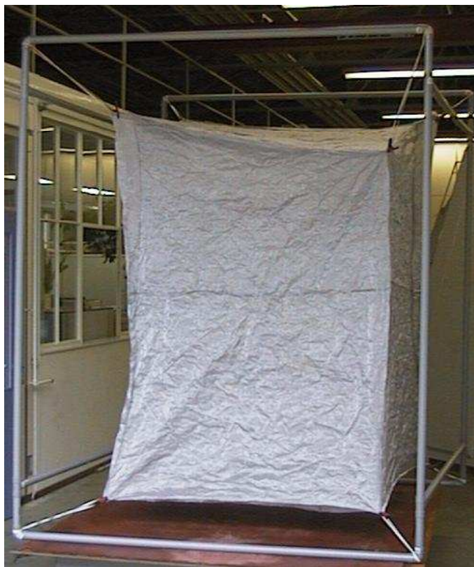
FIGURE 2.3: The VIRC: a flexible tent irregularly shaped. The field is stirred by moving the walls. The VIRC hanging in strings (Leferink et al., 2000).
