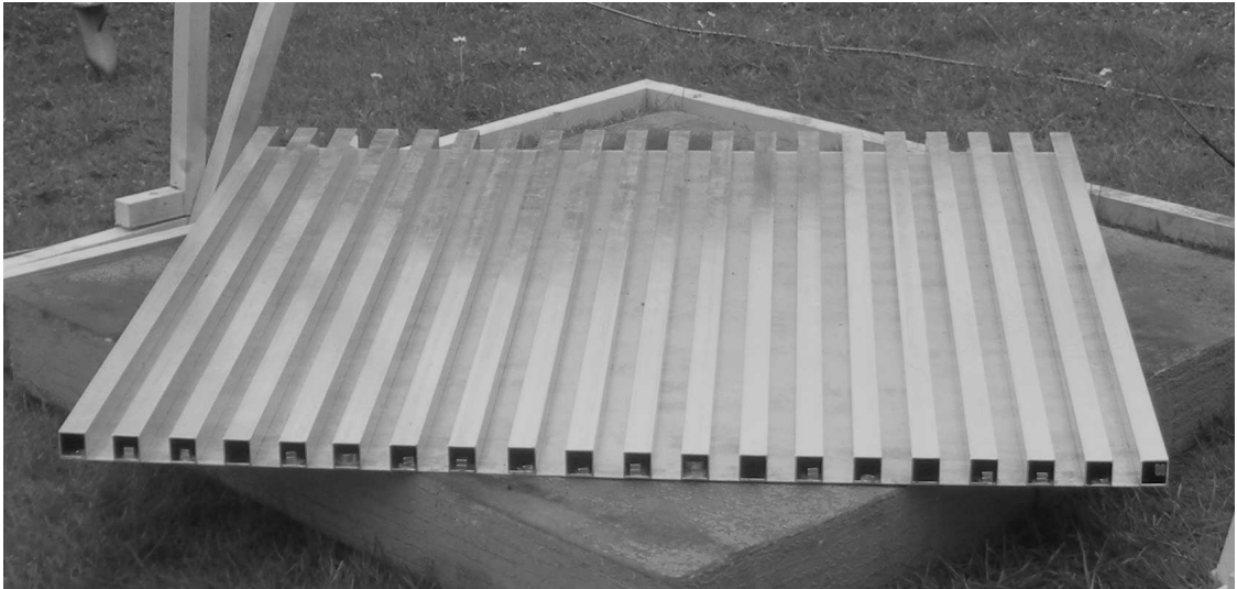
FIGURE 3.6: 1\text{m} \times 1\text{m} optimised orthogonal diffusers constructed according to the sequence s = [+1 -1 +1 -1] .
