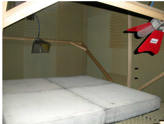
(a) Placing absorbers on the floor to measure the signal from the direct path.
