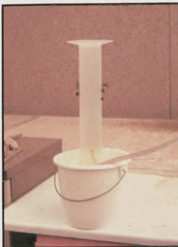
Plate 18 Gas collection unit for Phase 2 experiment in Leeds
