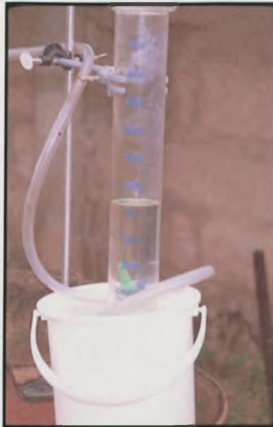
Plate 29 Gas collection unit for Phase 3 experiment in Kumasi
