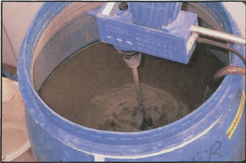
Plate 19 Stirring the influent to keep sludge particles in suspension and ensure a well mixed influent.
