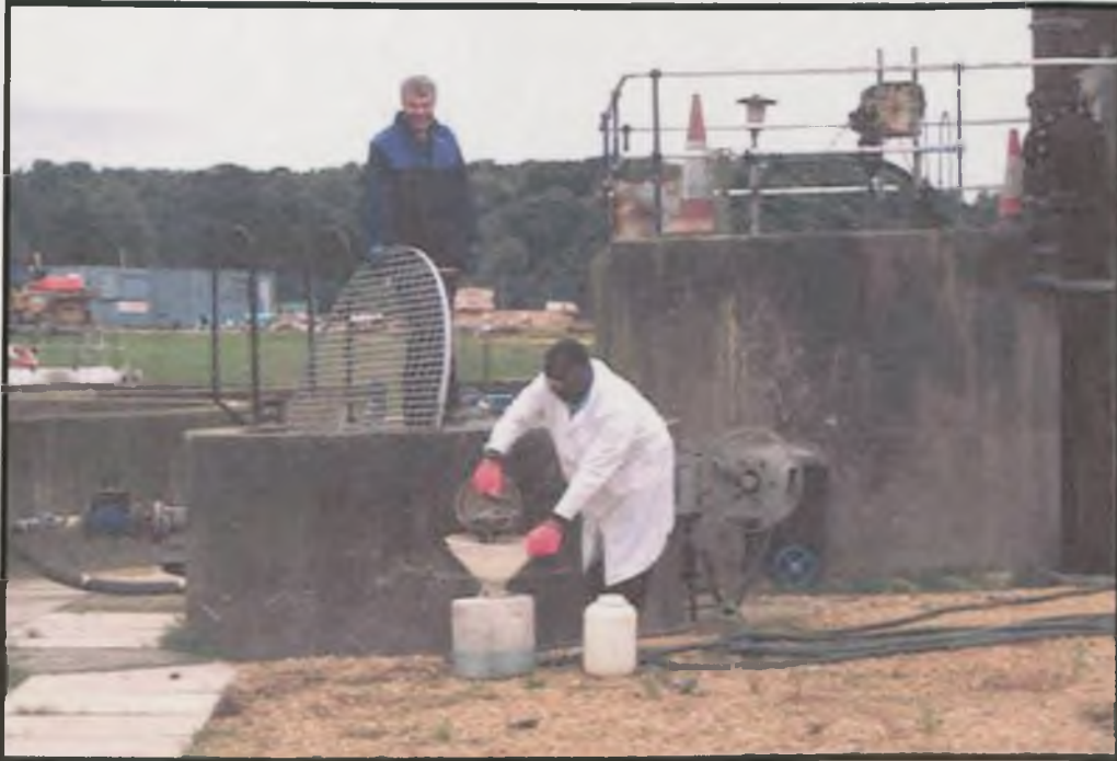
Plate 11 Taking sludge samples at Owl Wood Sewage Treatment Works
