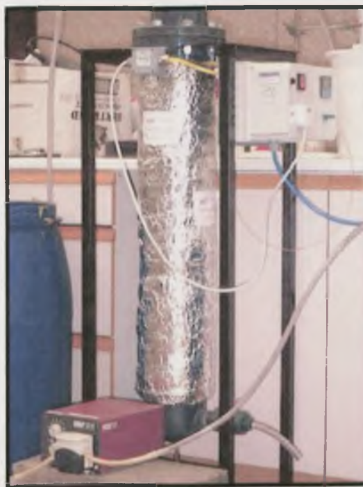
Plate 17 Heating coil wrapped around lower portion of reactor
