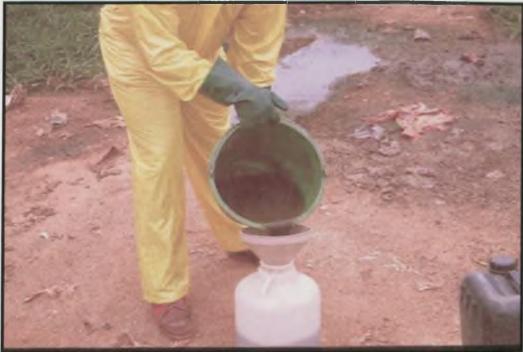
Plate 24 Filling 10-litre container with faecal sludge
