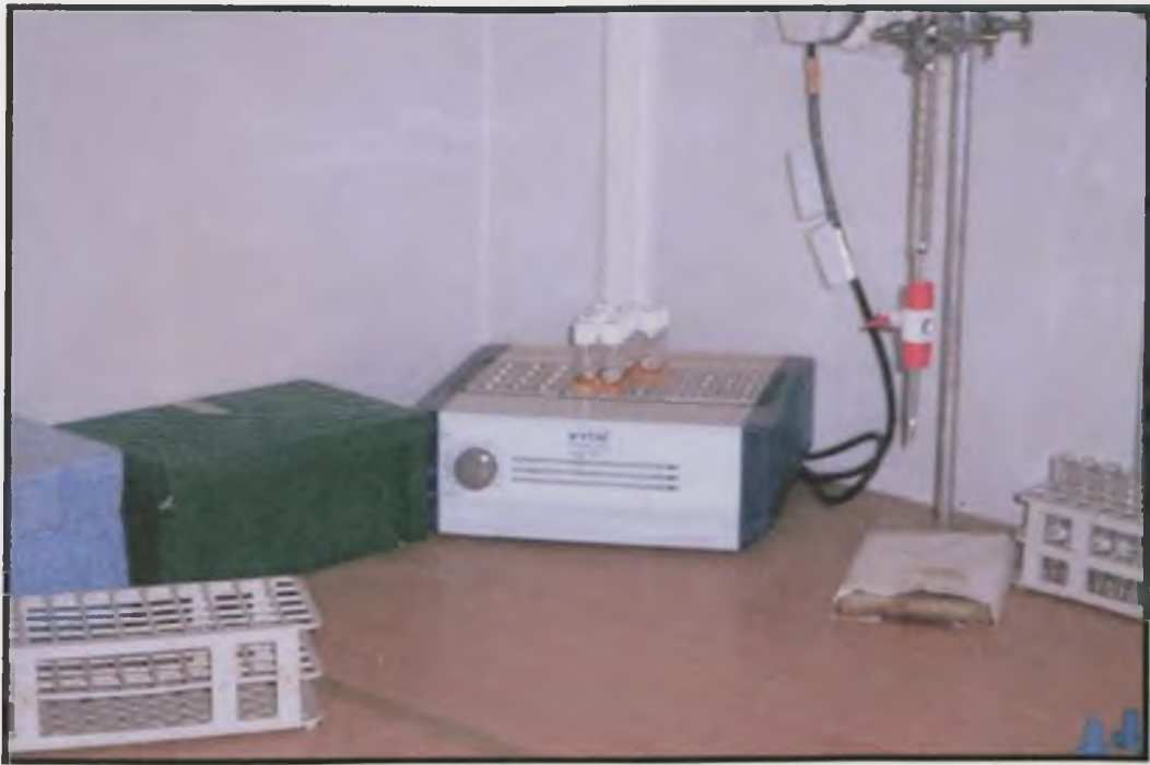
Plate 12 COD determination – digestion tubes in a heating block
