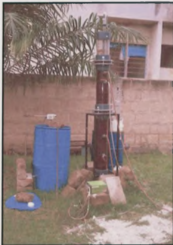
Plate 28 Experimental Set-up for the anaerobic digestion of faecal sludge using the UASB
