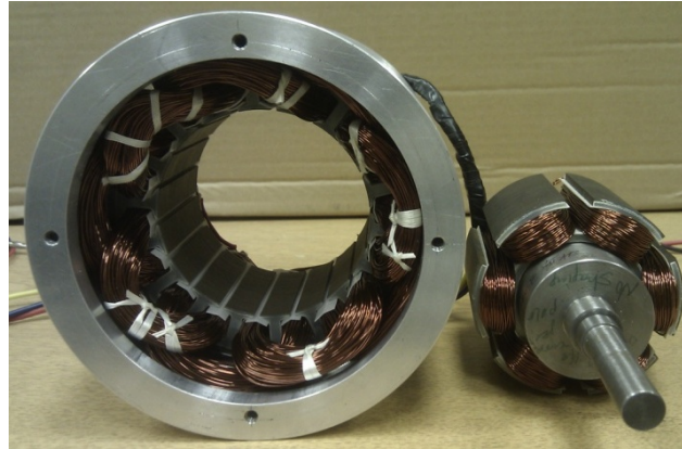
Fig. 6.21. Stator and rotor of EE prototype machine..
