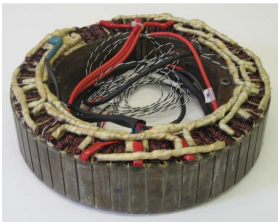
(a) Stator with windings
