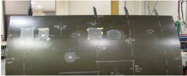
Figure 2.1: Panel with adhesively bonded composite patches [AMRC with Boeing research centre].
