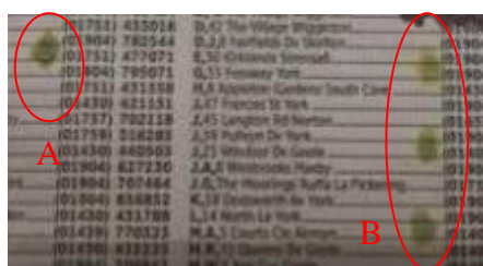
Figure 3.9 - Key: A = 5 \mu L spotted using a micropipette; B = triplicate spotting performed using TLC spotter.
