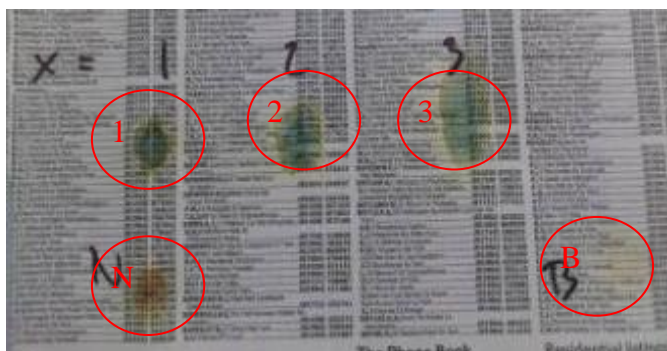
Figure 3.5 - Key: N = negative control (2 x 5 \mu\text{L} - Button Mushroom extract), B = blank (2 x 5 \mu\text{L} MeOH): 1 = 5 \mu\text{L} 37% HCl; 2 = 2 x 5 \mu\text{L} 37% HCl; x 3 = 3 x 5 \mu\text{L} 37% HCl on 10 \mu\text{L} (2 x 5 \mu\text{L} ) of methanolic Death Cap extract.
