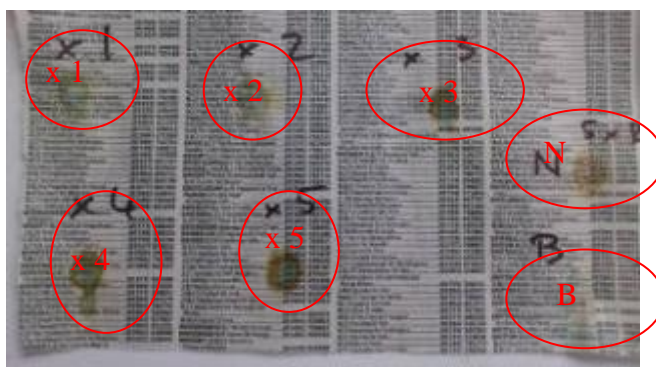
Figure 3.3 - Key: N = negative control (2 x 5 \mu\text{L} - Button Mushroom extract), B = blank (2 x 5 \mu\text{L} MeOH); x 1 = 5 \mu\text{L} ; x 2 = 2x 5 \mu\text{L} ; x 3 = 3x5 \mu\text{L} ; x 4 = 4x5 \mu\text{L} ; x 5 = 5x5 \mu\text{L} .
