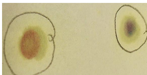
Figure 3.29 – The difference in colour between the two tested compounds after 10 minutes at 0.2 mg/mL. Left: 5-HIAA; right: 5-MT.
