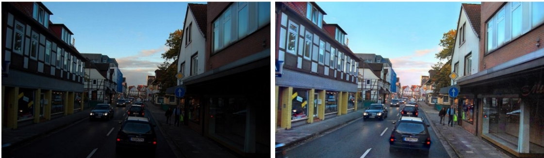
Figure 2.10: Representative low-light driving image (left) and enhanced result (right). Example from EnlightenGAN (Jiang et al., 2021).
