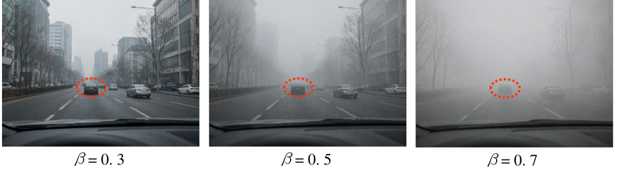
Figure 1.5: A driving scene under three fog densities, parameterised by the scattering coefficient \beta in Eq. (1.1). Illustration generated by the author.
