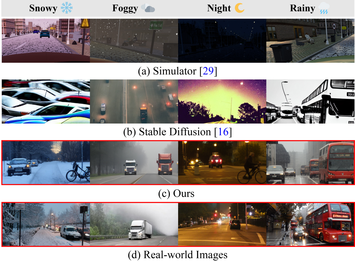
Figure 6.1: Representative failure modes of alternative sources for adverse weather training images. (a) A driving simulator (Kerim et al., 2022) provides geometric control but produces visually synthetic scenes with coarse textures and simulator-like colour statistics. (b) Vanilla Stable Diffusion (Rombach et al., 2021) generates visually appealing images, but often violates dashcam geometry through artistic composition and incorrect camera perspective. (c) WeatherDG generates photorealistic adverse weather driving images with dashcam-compatible viewpoint and scene layout, closely resembling (d) real adverse weather driving images.
