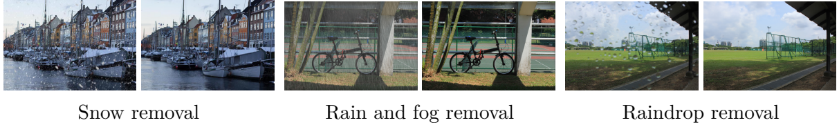
Figure 2.8: Representative single-type weather restoration; each pair shows the degraded input (left) and restored output (right). Examples reproduced from the official WeatherDiffusion repository accompanying Özdenizci and Legenstein (2023).
