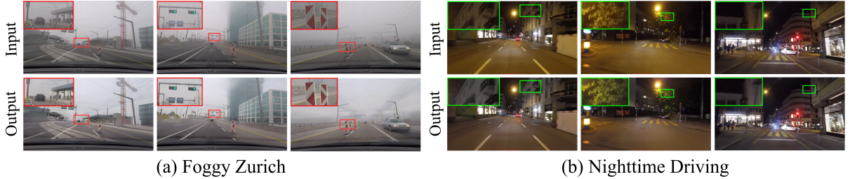
Figure 4.10: Qualitative generalisation results on Foggy Zurich and Nighttime Driving, both held out from training. AllWeatherNet improves clarity of vehicles, signs, and buildings in fog, and corrects colour casts from artificial lighting at night.
