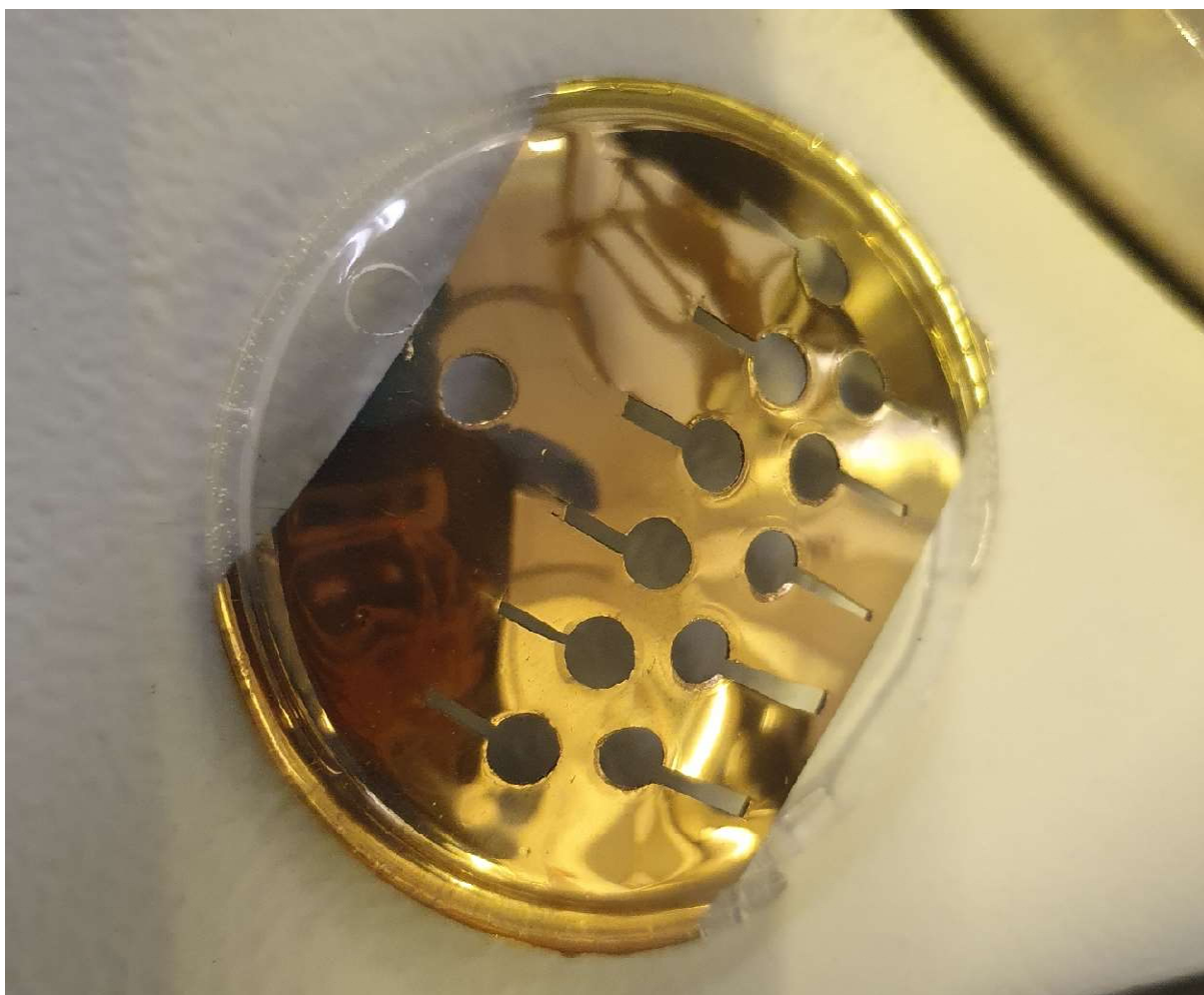
Figure S8: Conformal silicone mask used to pattern gold back contacts; this image was taken post deposition.
