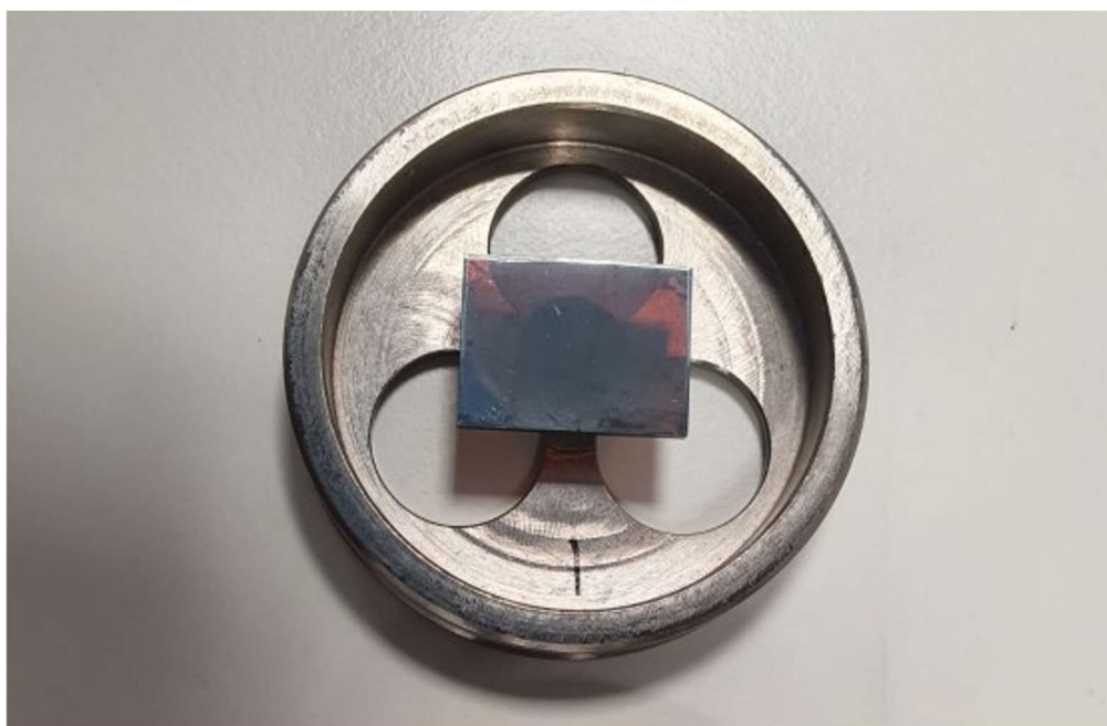
Figure 3.13: A perovskite sample mounted in a bulk sample holder, prepared for XRD measurement. The non-elastic putty is visible through the perovskite film. Here, the sample is positioned at an exact height, and perfectly horizontal, within the holder using a clean microscope slide and the rim of the sample holder.
