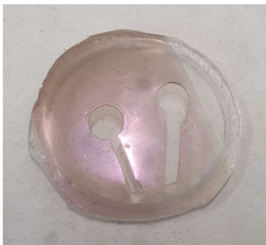
Figure S13: Silicone evaporation mask used to define device pixels on a curved CFRP substrate, note this image recorded after the ITO deposition.
