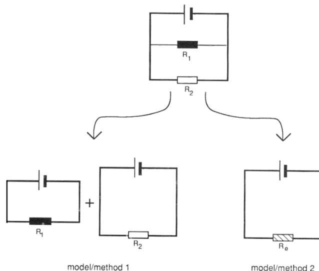
**Figure 5.5: Two models of parallel circuits leading to two methods of tackling parallel circuit problems (Millar and Beh, 1993, p. 354)**
