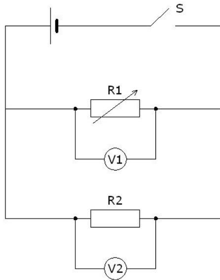
**Figure 5.7: Circuit diagram showing voltmeters connected across parallel resistors**
