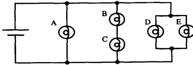
**Figure 2.4: Predicting the relative brightness of the bulbs (from McDermott and Shaffer, 1992)**
