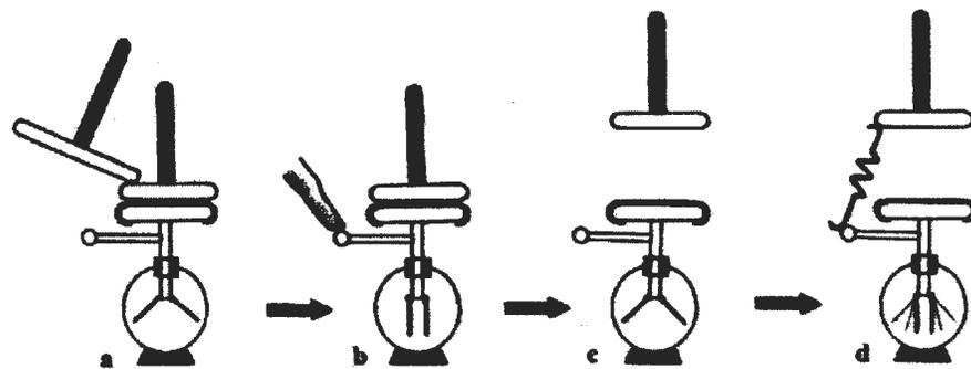
**Figure 12.** In (a) and (b) two metallic discs are charged. The system is a capacitor with variable capacitance. In (d) a current discharges the capacitor.
