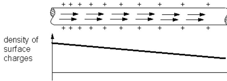
**Figure 2.16: Linear density distribution of surface charges on a rectilinear conductor (from Haertel, 2008a, p. 5)**
