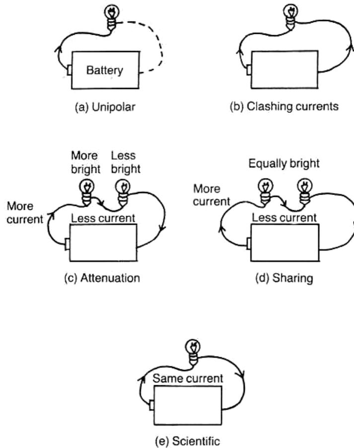
**Figure 2.2: Children’s models for current in simple circuits (from Shipstone, 1985b, p. 36)**
