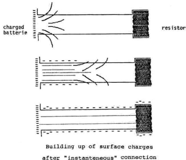
**Figure 2.15: Building up of surface charges after connecting a complete circuit (from Duit, 1991)**
