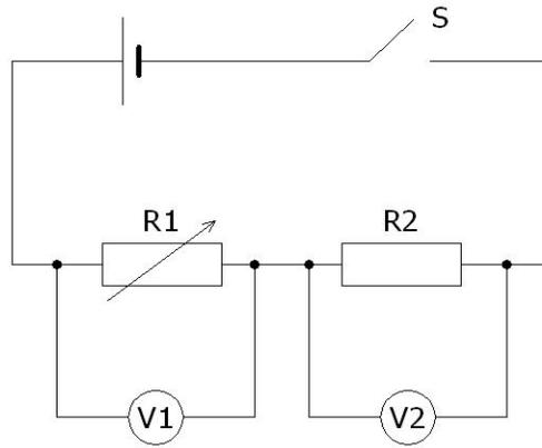
**Figure 5.6: Circuit diagram showing voltmeters connected across series resistors**
