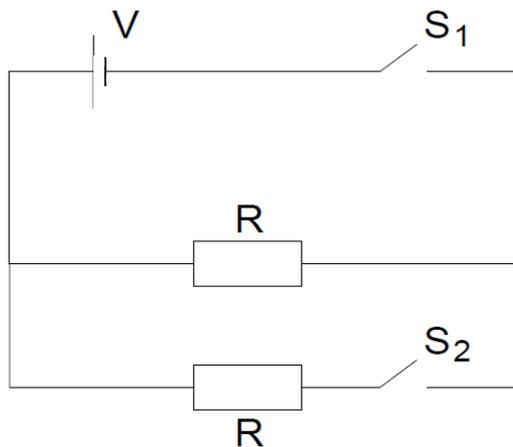
**Figure 6.5:** The circuit diagram for an added resistance in parallel
