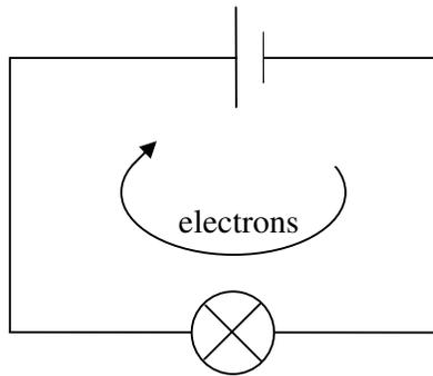
**Figure 6.1: Electron flow in an electric circuit**
