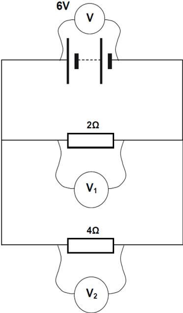
(a) What is the reading, in volts, on voltmeter  $V_1$ ?
