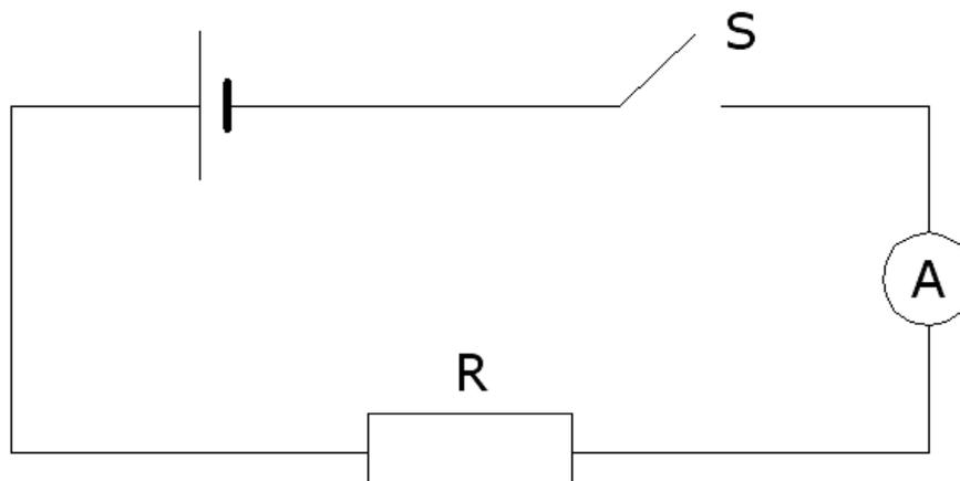
**Figure 1: A simple circuit**
