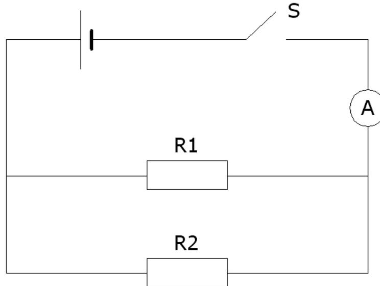
**Figure 3: A parallel circuit**
