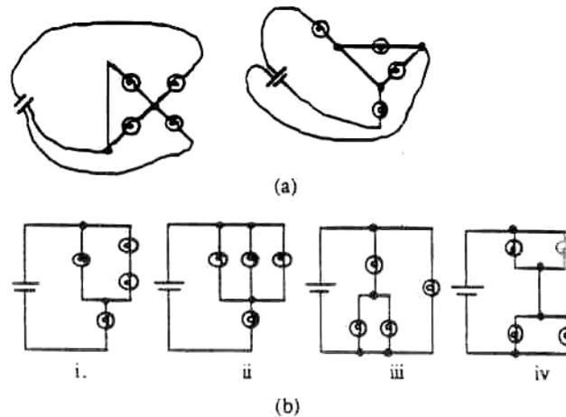
**Figure 2.5: Resistance in complex circuits (from McDermott & Shaffer, 1992)**
