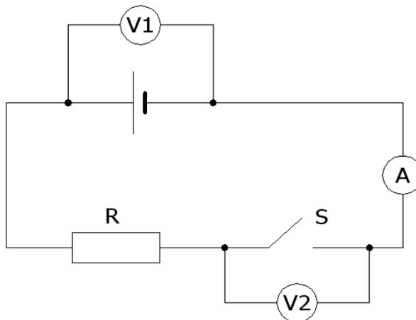
**Figure 6: Voltmeters across the battery and switch**
