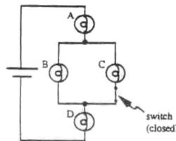
**Figure 2.7: Predicting the brightness of identical bulbs when the switch is closed (from McDermott and Shaffer, 1992, p. 998)**
