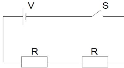
**Figure 6.4:** The circuit diagram shown to students adding a resistance in series
