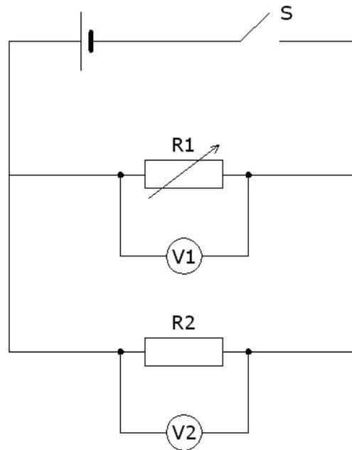
**Figure 5: Voltmeter readings in a parallel circuit**
