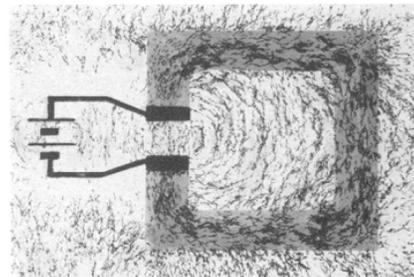
**Figure 2.14: Fields inside and surrounding current carrying conductors (from Jefimenko, 1962, p. 20)**
