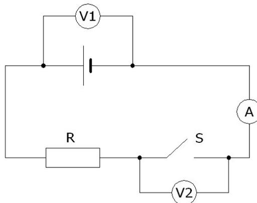
**Figure 5.8: Circuit diagram showing voltmeters connected across the battery and the switch**
