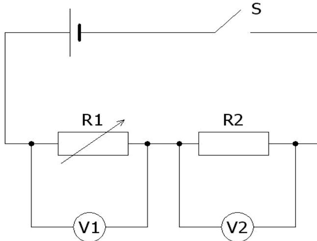
**Figure 4: Voltmeter readings in a series circuit**
