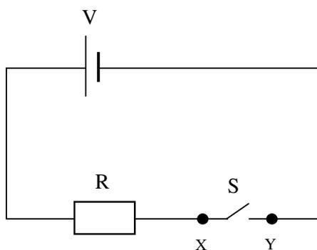
**Figure 5: A simple circuit with S opened**
