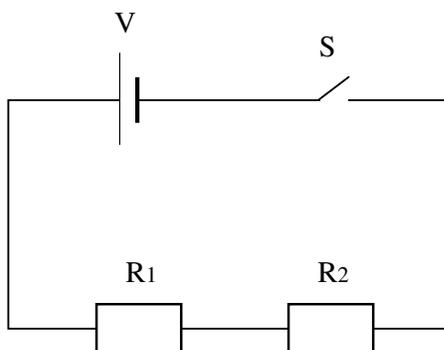
**Figure 2:** A series circuit
