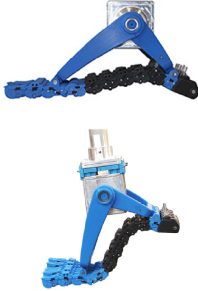
Figure 7: The SoftFoot designed by Piazza et al. Taken from [32].
