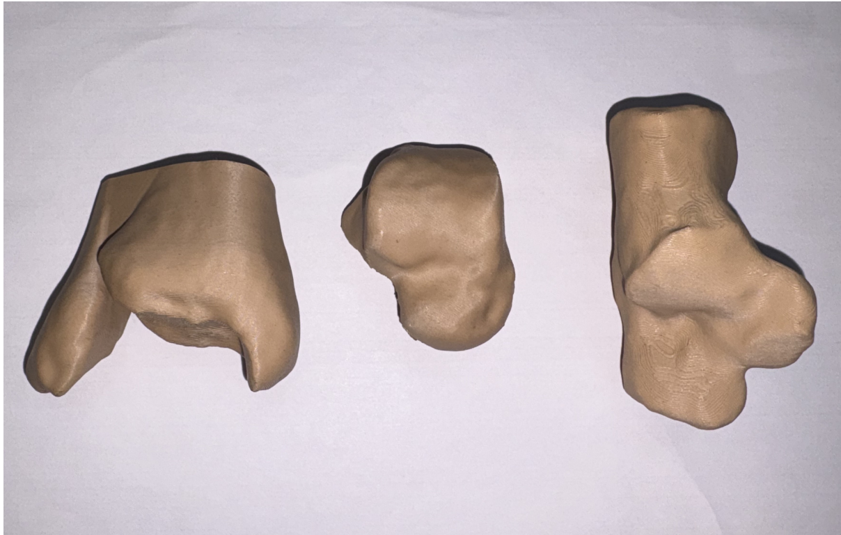
Figure 21: The smoothed bone structured as 3D printed from the CAD files. Shown here from left to right are the now fused shank (the tibia and fibula), talus, and calcaneus bones.
