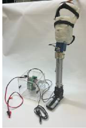
Figure 15: The bent knee rig implemented by both McMullan and Leake. Taken from [43].
