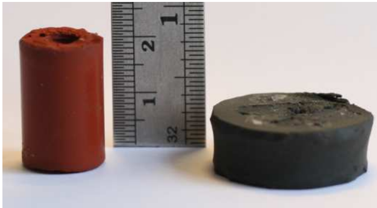
Figure 5.20: Test specimens (surface damage caused during removal from test rig)
