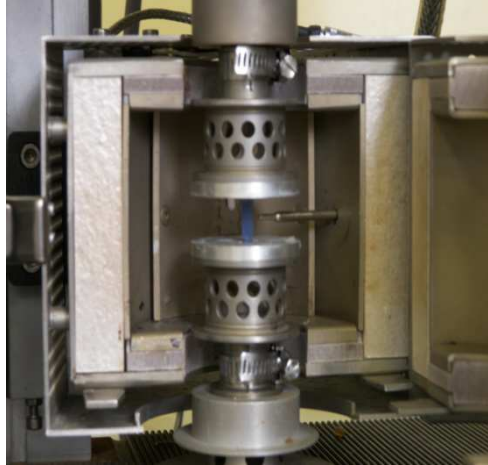
Figure 3.5: Viscoanalyser machine (DMTA) to measuring material properties
