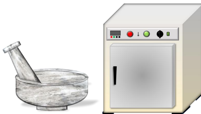
Figure 3.8: Equipment for melt amorphisation, mortar and pestle to mix the sample and a heating oven, where the sample is melted.
