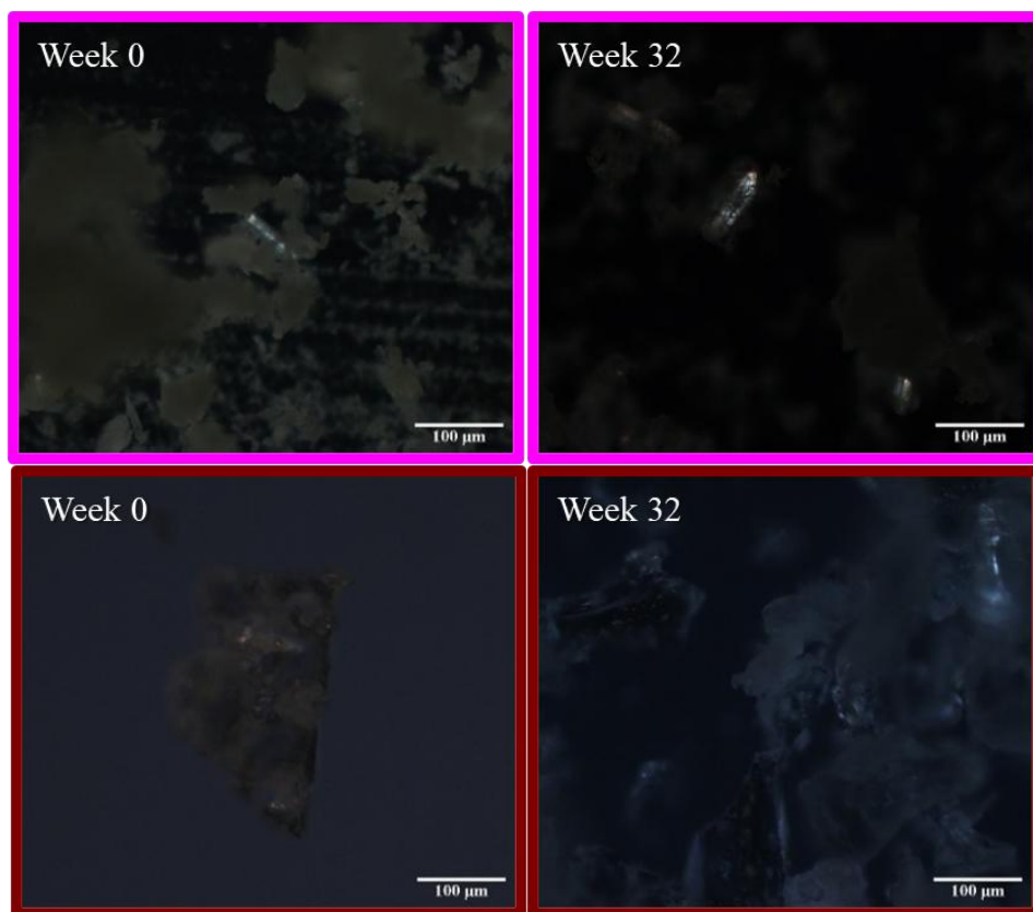
Figure C.1: PLM images of SC VAL and Am VAL (bordered in magenta and maroon respectively) at weeks 0 and 32 at 25% RH. Crystallinity was evaluated by analysing 10 images per sample, at a given time.
