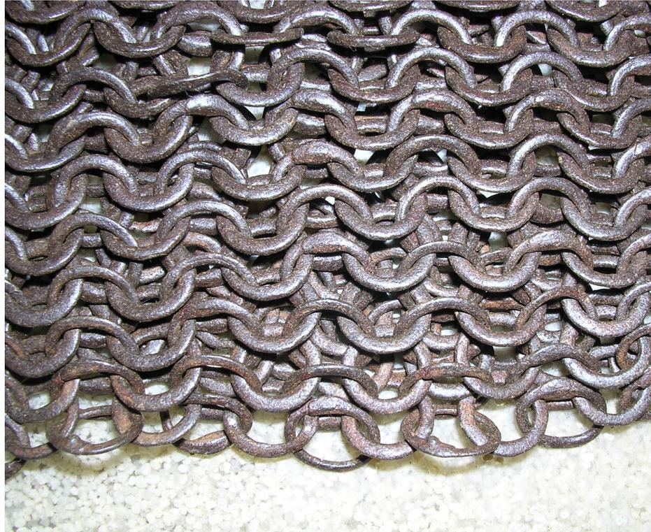
Figure 1 Detail of the inside of an example of mail horse armour of the fourteenth century, showing the inner ends of the wedge-shaped rivets. Royal Armouries no. VI.566.
