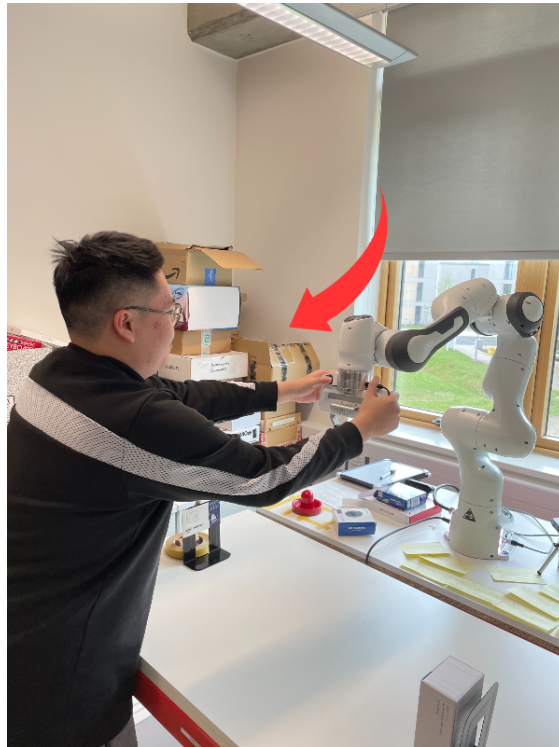
Figure 4.16: Kinesthetic teaching on the 7-DoF Franka robot: with the manipulator in zero-gravity compliance mode, an operator manually guides the end-effector along the desired path (red arrow).
