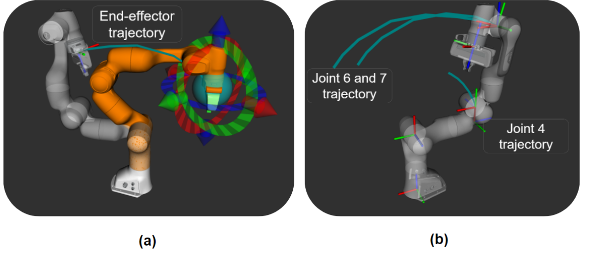
Figure 4.13: (a) illustrates the operation sequence of a Franka robot arm, beginning with the initial stage (highlighted in orange) and progressing towards a state near to a singularity. (b) displays the motion trajectories of Joints 4, 6, and 7, which are influenced by the singularity.
