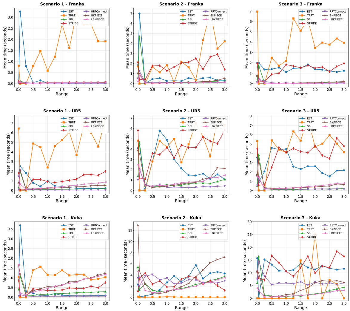
Figure 3.5: Mean planning time, in seconds, as a function of the range parameter for seven motion planners (EST, TRRT, SBL, STRIDE, RRTConnect, BKPIECE, and LBKPIECE) on the three robotic arms.
