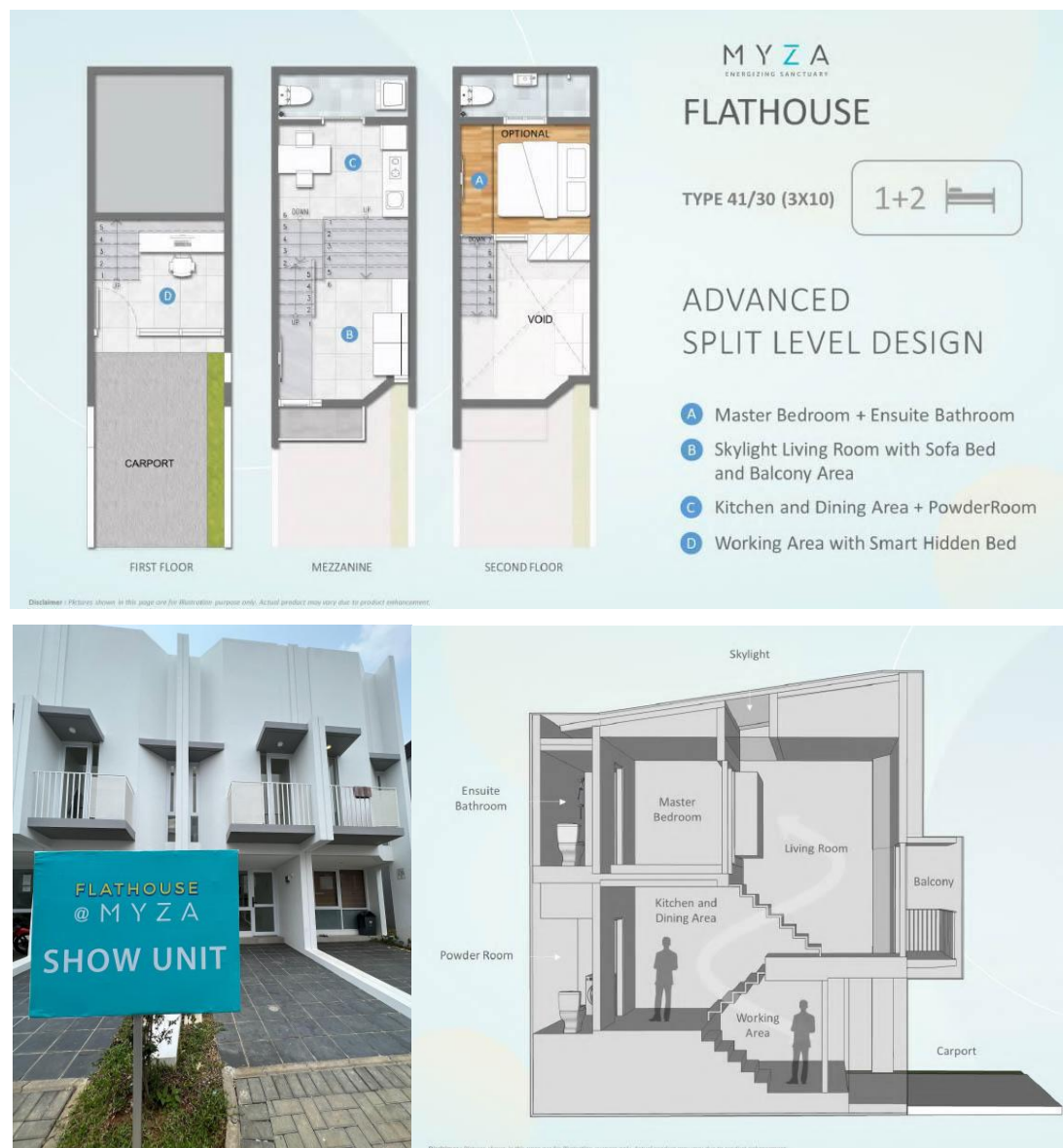
Figure 4.11 Details of Flathouse in BSD City Sources: BSD City brochure and author's photograph, 2023
