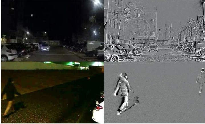
Figure 1.19: The outputs of an RGB camera, and event camera in low light scenarios, with negative events shown in black and positive events shown in white.
