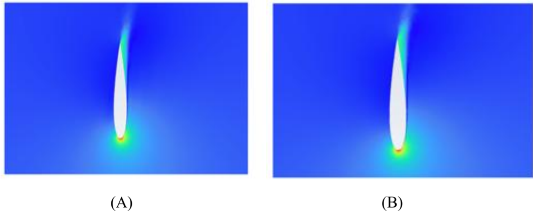
Fig. 5.25: Velocity distribution around (A) NACA0015 and (B) optimized airfoils when VAWT-130 at 90^\circ azimuthal angle where maximum improvements in the momentum occurs.
