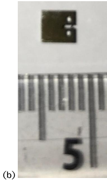
Figure 118: (a) Deformed HPT sample with FCG sample removed; (b) Machined FCG sample
