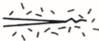
Figure 66: Brittle crack tip in FCG sample (Jenkins, 2018)
