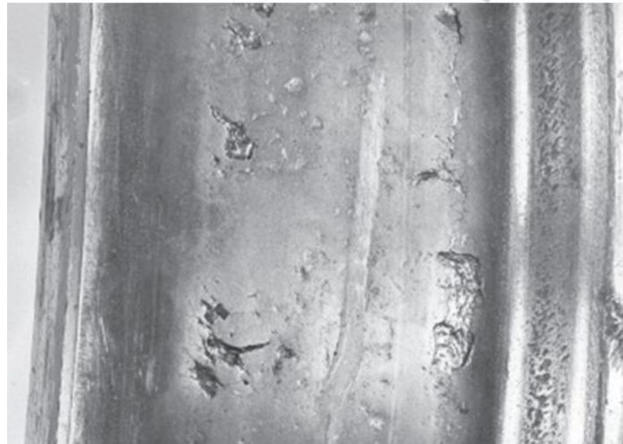
Figure 51: Fatigue wear leading to spalling from a wheel (Ekberg and Sotkovszki, 2001)
