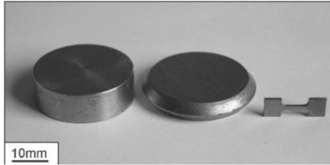
Figure 43: Dog bone specimen from processed HPT intended for tensile testing (Larijani, Kammerhofer and Ekh, 2015)
