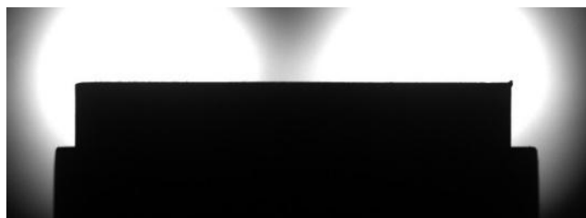
Figure 5.1 – An example image from the High-Speed rig front camera showing uneven illumination of blade.
