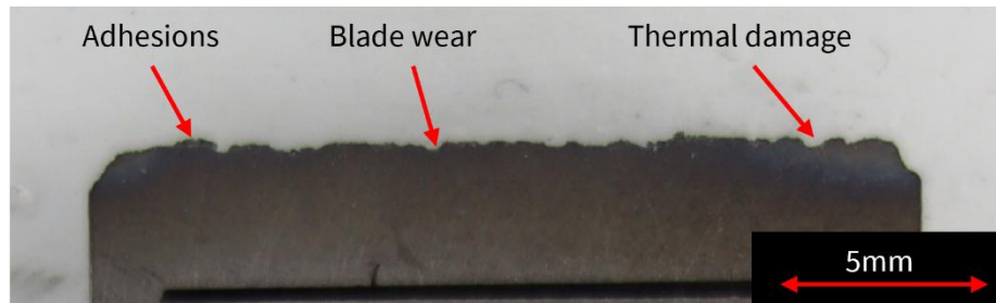
Figure 6.12 – Image of a tested blade from a 0.02 \mu m/pass, 52HR15y M601 test showing multimodal wear
