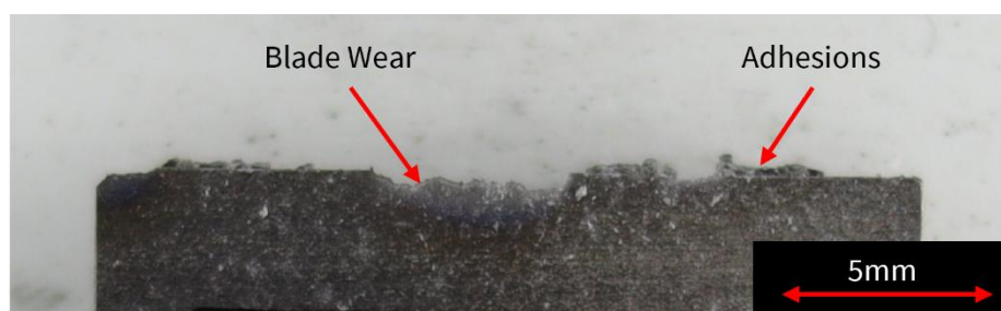
Figure 7.11 – Image of mixed modal wear on a blade tested against M320 62HR15y, 0.02 \mu m/pass with 200°C backplate
