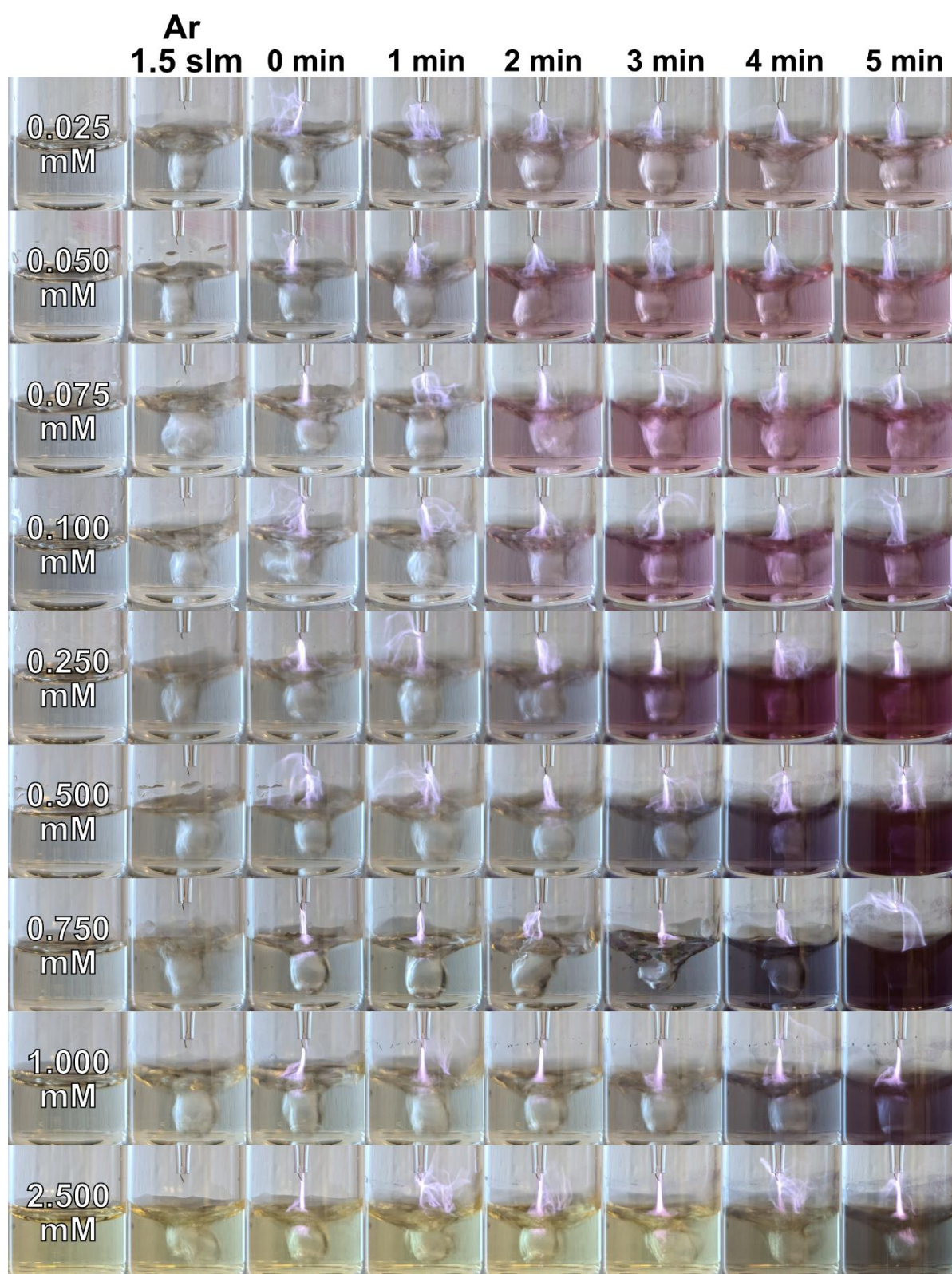
Figure 4.4. Process of the nanoparticle synthesis from aqueous precursor solution to colloidal nanogold over 5 min of treatment time.
