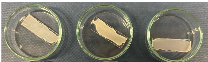
Figure 6.1. Samples of polyaminoborane that had been spin coated onto glass plates. Polyaminoborane was dissolved in THF (20 % w/w) to form the spin coating solution. The spin coating ramp programme that formed the most even thin film (right) was: 1000 rpm for 10 s with ramp up to 4000 rpm for 90 s.
