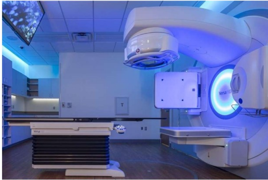
Figure 3 Radiotherapy machine (linear accelerator or 'linac')
