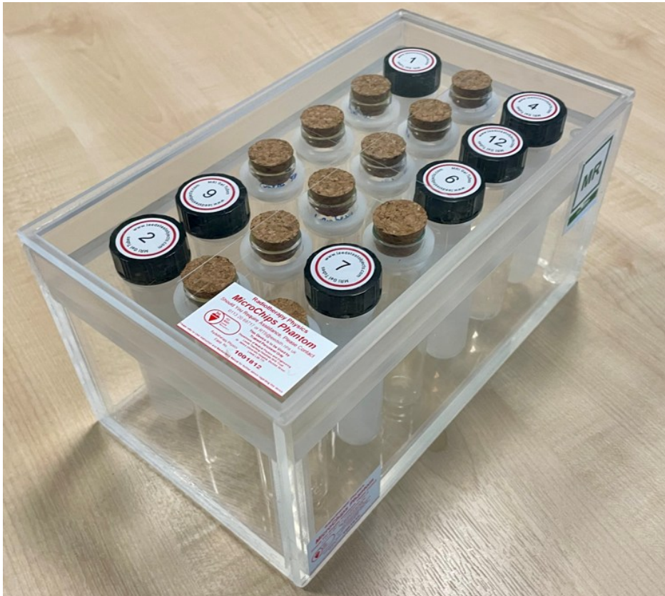
Figure 20 The MICROCHIPS acrylic phantom; test tube holder manufactured for this study.
