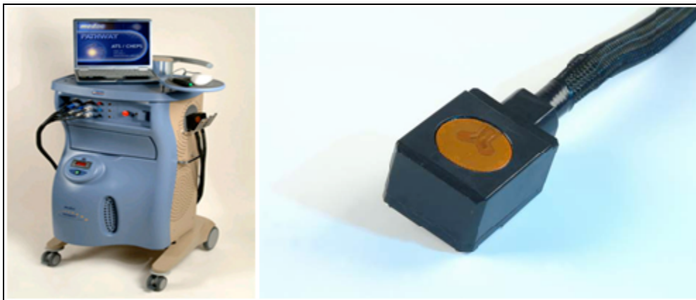
Figure 2.1: Medoc Pathway unit (left) and CHEPS thermode used for thermal stimulation (right).
