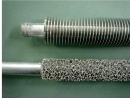
Figure 4.26: A helically finned (top) and metal foam covered tube [132].
