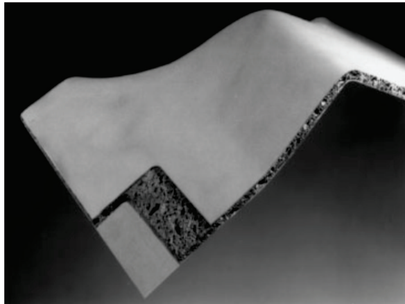
Figure 3.5: Aluminium foam sandwich (AFS) produced by Karman, Osnabruck (Germany) [80].
