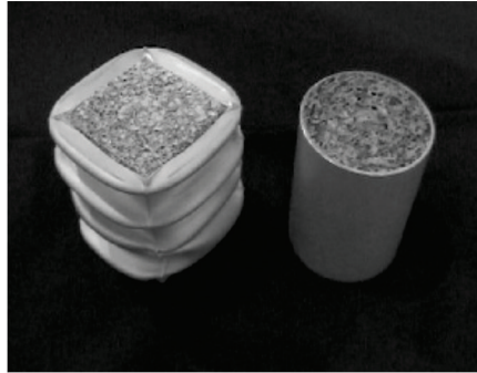
Figure 3.2: Prototypes of crash absorbers based on extruded aluminium hollow sections filled with Cymat aluminium foam [74].
