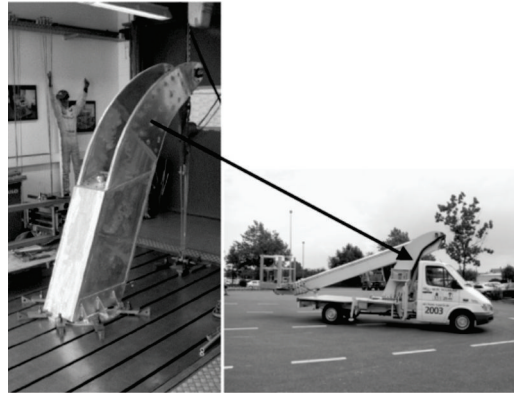
Figure 3.6: Base of a lifting arm for a truck made from AFS sandwich panels. [67].
