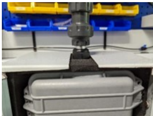
Figure 26: Soundproofing foam placed to cover the opening on top of the enclosure
