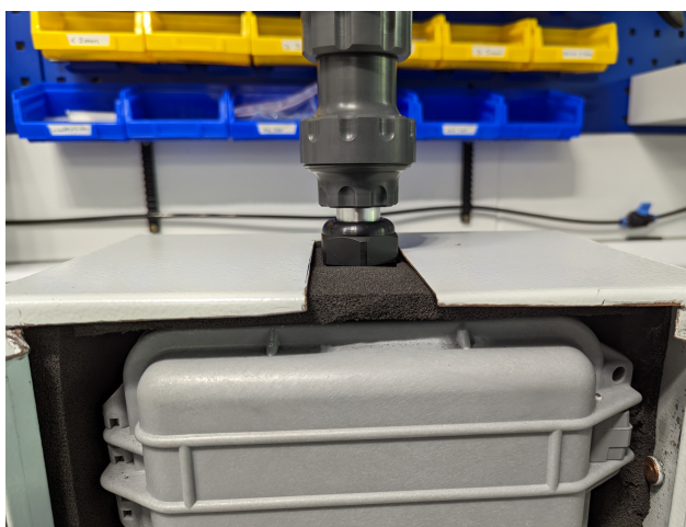
(b) The opening in the top of the enclosure, showing where an additional layer of foam has been placed to reduce noise escaping
