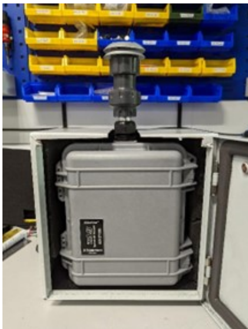
Figure 25: Sampler placed inside enclosure
