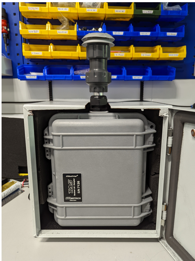
(a) The Minivol TAS, placed inside the soundproofing enclosure
