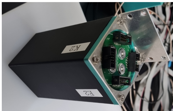
Fig. 7.13 GAGG encapsulated in the plastic housing with the feed-through PCB shown.
