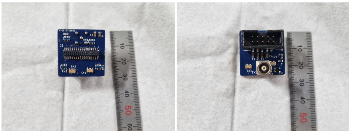
Fig. 7.30 Circuit diagram of simple readout board alongside pictures of the assembled PCB for the circuit shown in Figure 7.5.
