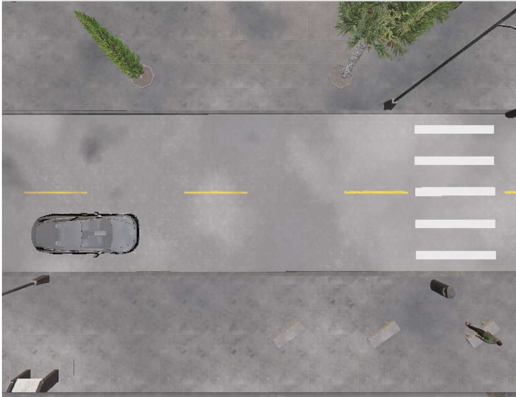
Figure 5.1: Illustration of the zebra crossing interaction scenario used to evaluate the impact of different pedestrian models on AV behaviour. The pedestrian begins at a standstill, positioned 4 m from the centreline of the vehicle lane and 2 m from the kerb, while the AV approaches at the constant speed under different Time-to-Arrival (TTA) settings. The pedestrian began at a standstill, positioned 4 m from the centreline of the vehicle lane and 2 m from the kerb, and waited at the kerb before initiating a crossing
