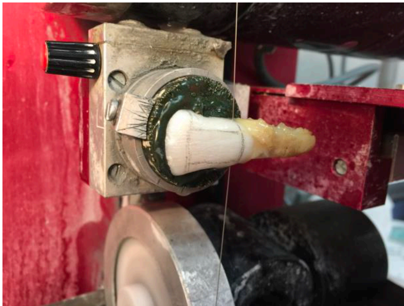
Figure 3. Diamond wire saw apparatus used for teeth sectioning.
