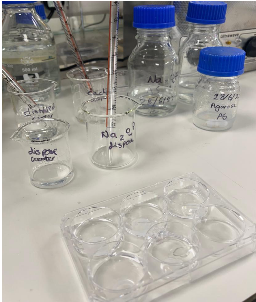
Figure 13. The agarose gel disks were placed into six well plates and immersed with aqueous solution of \text{CaCl}_2 for one hours.
