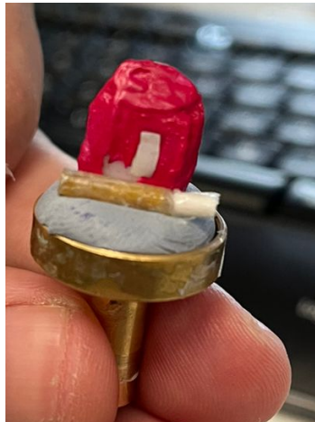
Figure 9. Represents the phantom used in calibration to the images in the Micro-CT.
