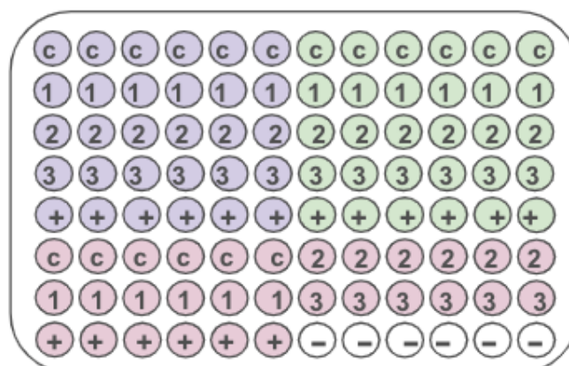
Figure 2.4: Layout of 96 well plates for phage efficacy assays. Each colour block represents a different P. aeruginosa strain: light purple indicates strain 203.1, light green indicates strain 413, and light pink indicates strain 342. Within each colour block, wells are designated as follows: c = phage cocktail treatment (192 \mu\text{L} SCFM, 4 \mu\text{L} bacterial culture, 4 \mu\text{L} cocktail at MOI 0.1); 1, 2, 3 = individual phage treatments (192 \mu\text{L} SCFM, 4 \mu\text{L} bacterial culture, 4 \mu\text{L} individual phage at MOI 0.1); + = bacteria-only positive control (196 \mu\text{L} SCFM, 4 \mu\text{L} bacterial culture); - = media-only negative control (200 \mu\text{L} SCFM). Each condition is performed in triplicate across rows. All bacterial cultures were diluted to MOI 0.1 prior to plating.
