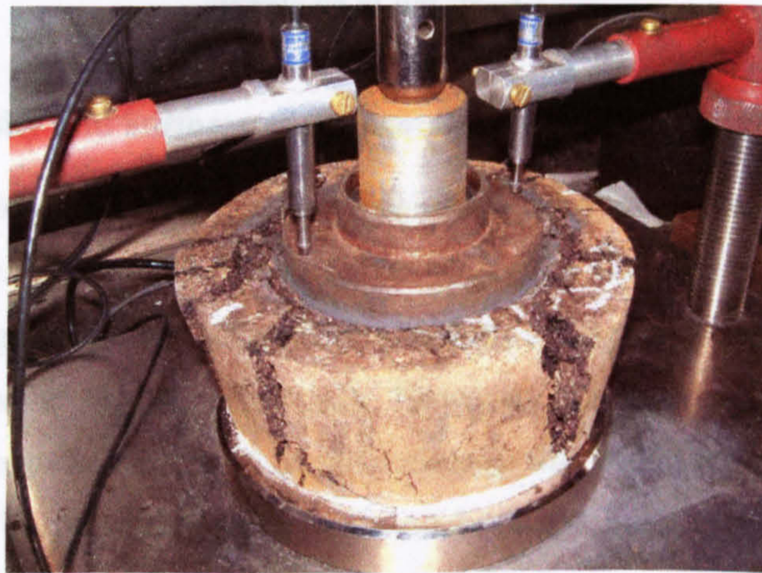
Fig. 9.23 Failure of the WPC sample, with plastic cells at mid depth.
