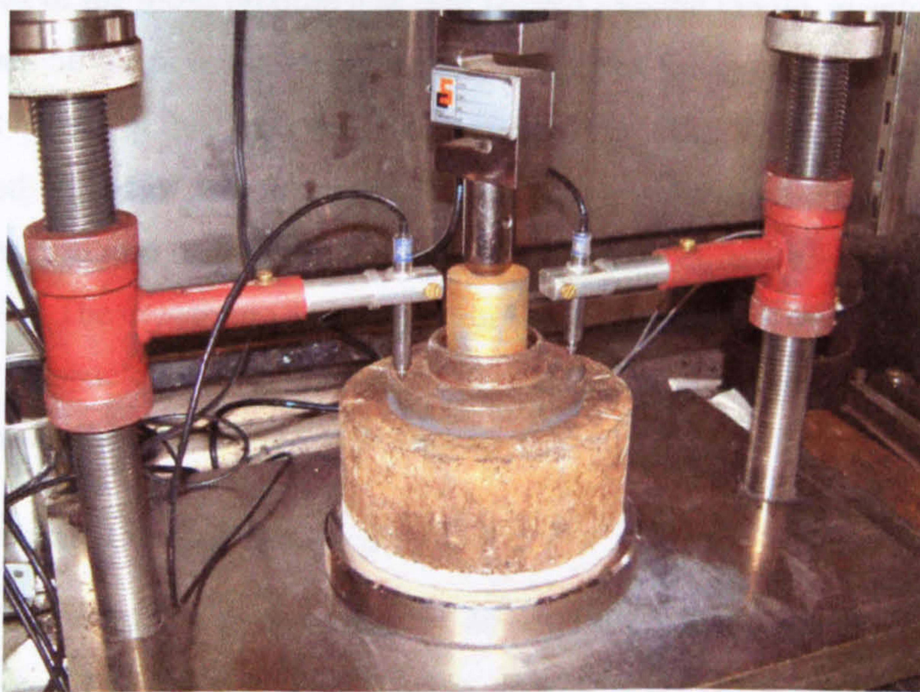
Fig. 9.20 Dynamic Loading of the capped CBEMs.
