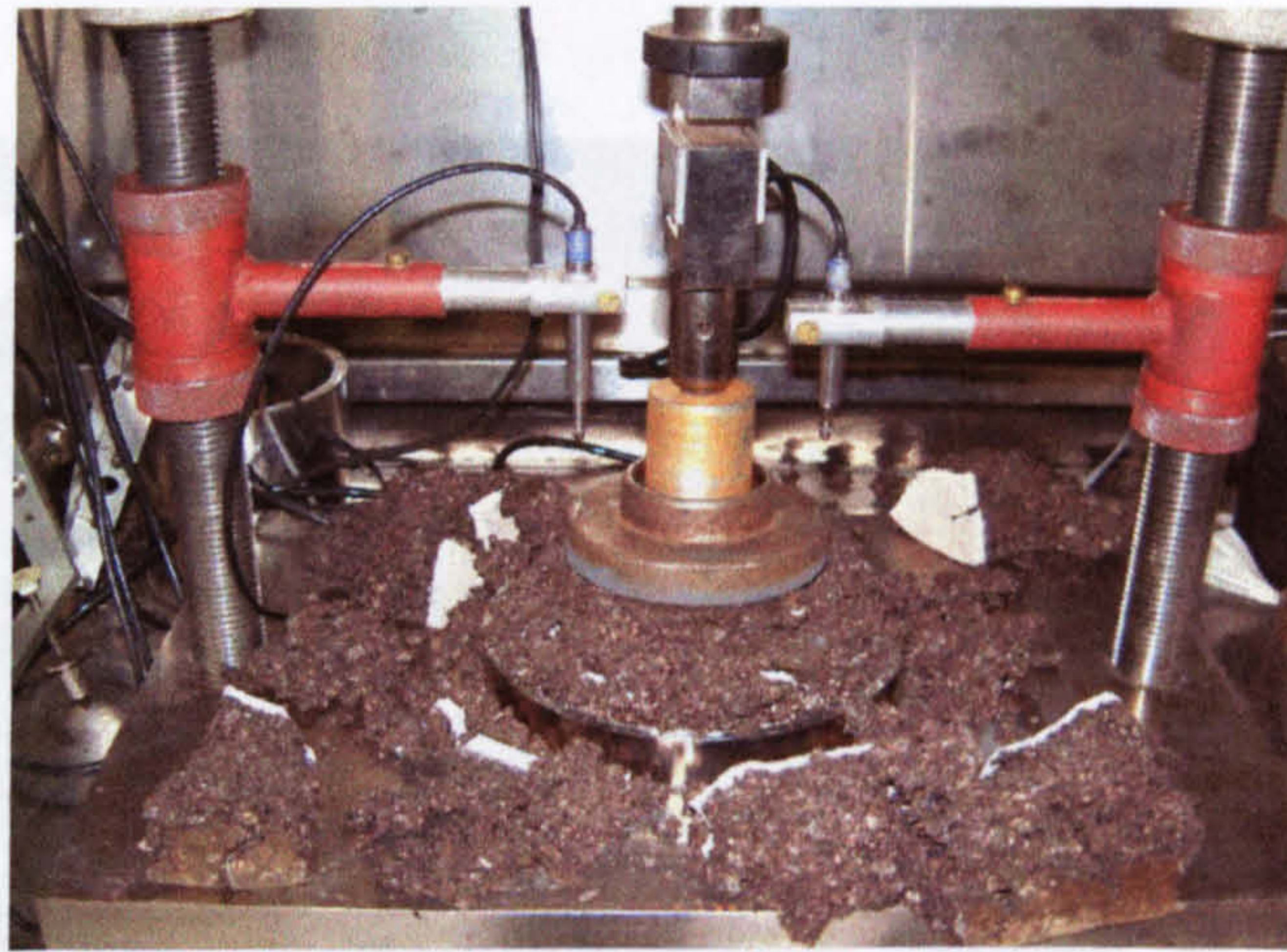
Fig. 9.22 Total failure of the NPC sample.
