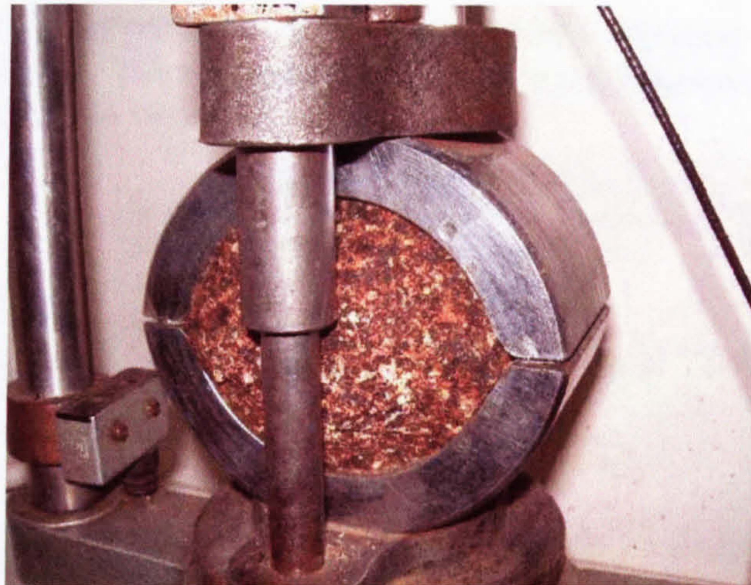
Fig. 7.9 A CBEM sample at maximum flow, showing plastic mode of failure.
