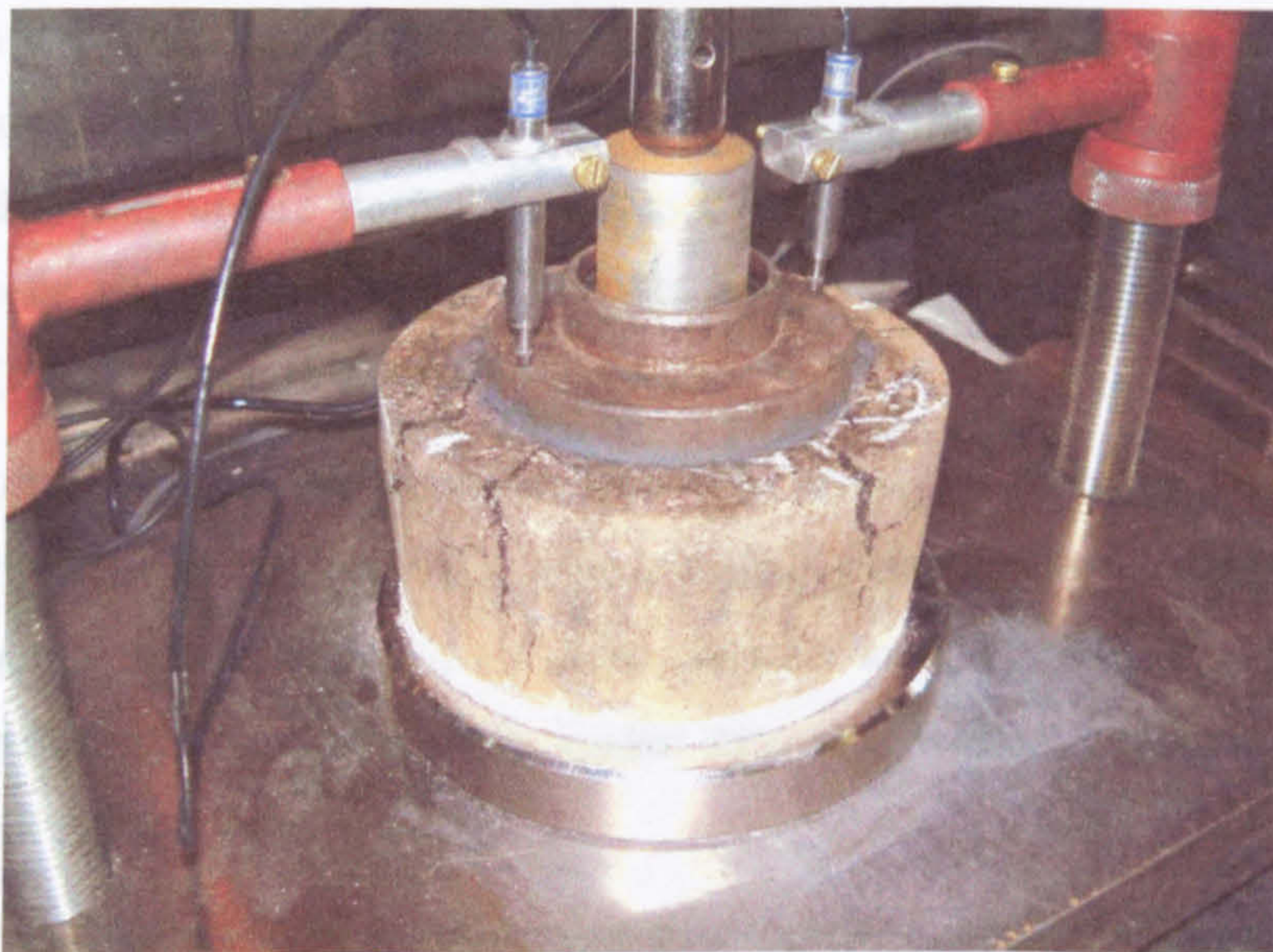
Fig. 9.28 Propagation of cracks in the NPC sample during the final investigation.
