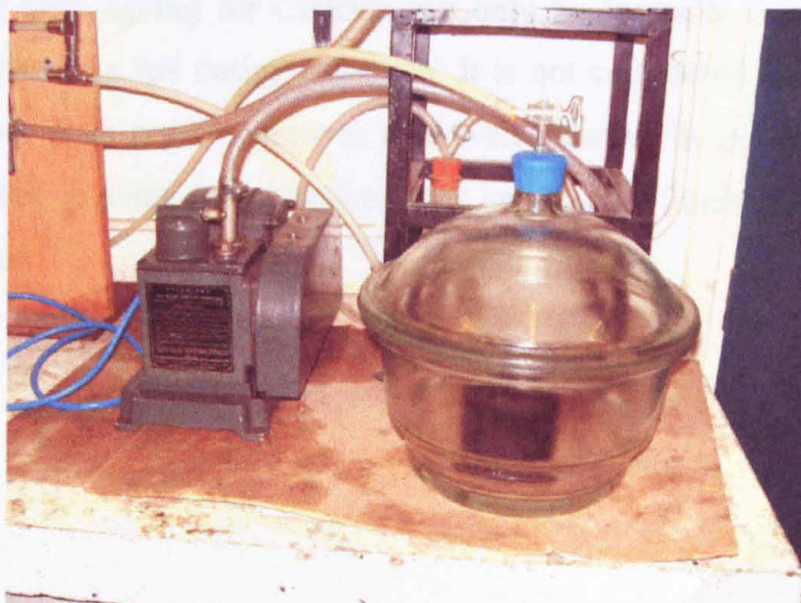
Fig. 5.16 Vacuum saturation apparatus.
