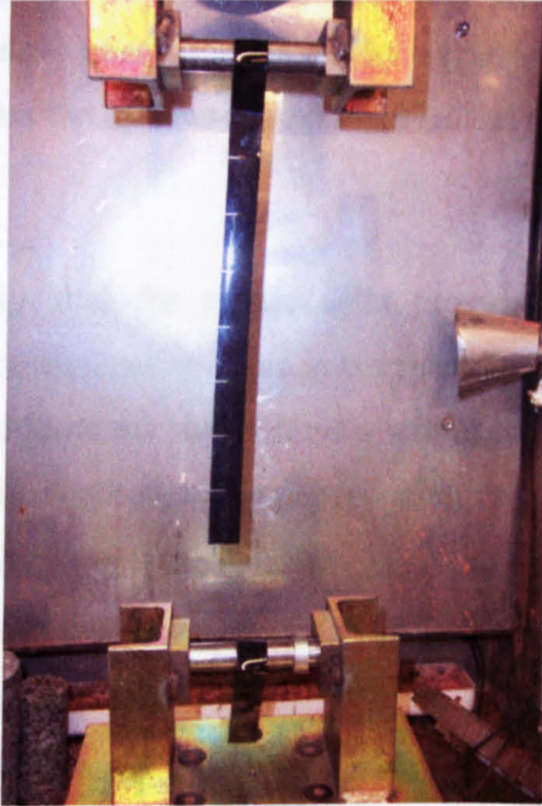
Fig. 9.35 Failure of a plastic strip during direct tension test.
