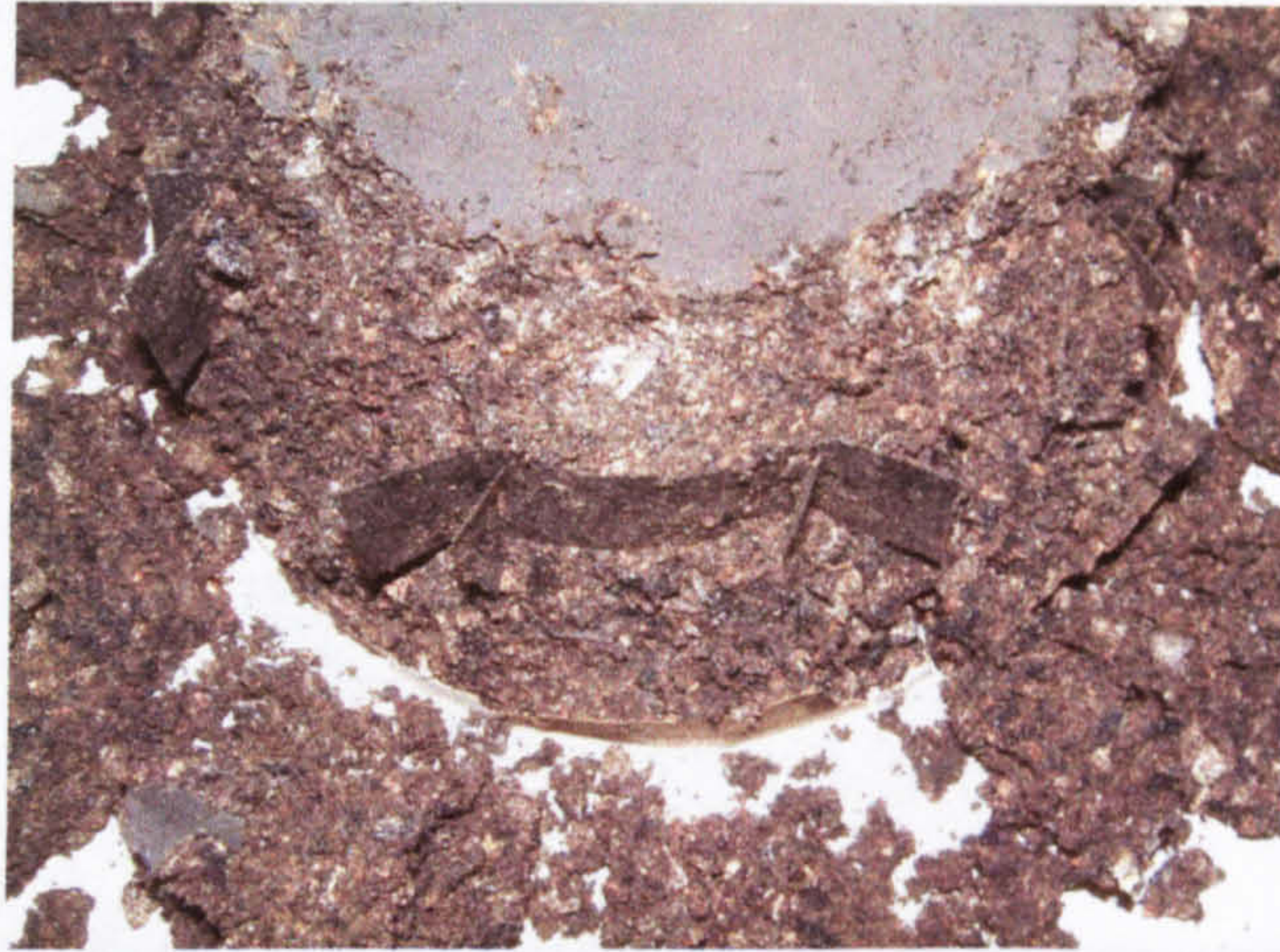
Fig. 9.25 View of the plastic cells within the failed sample as in Fig. 9.23.
