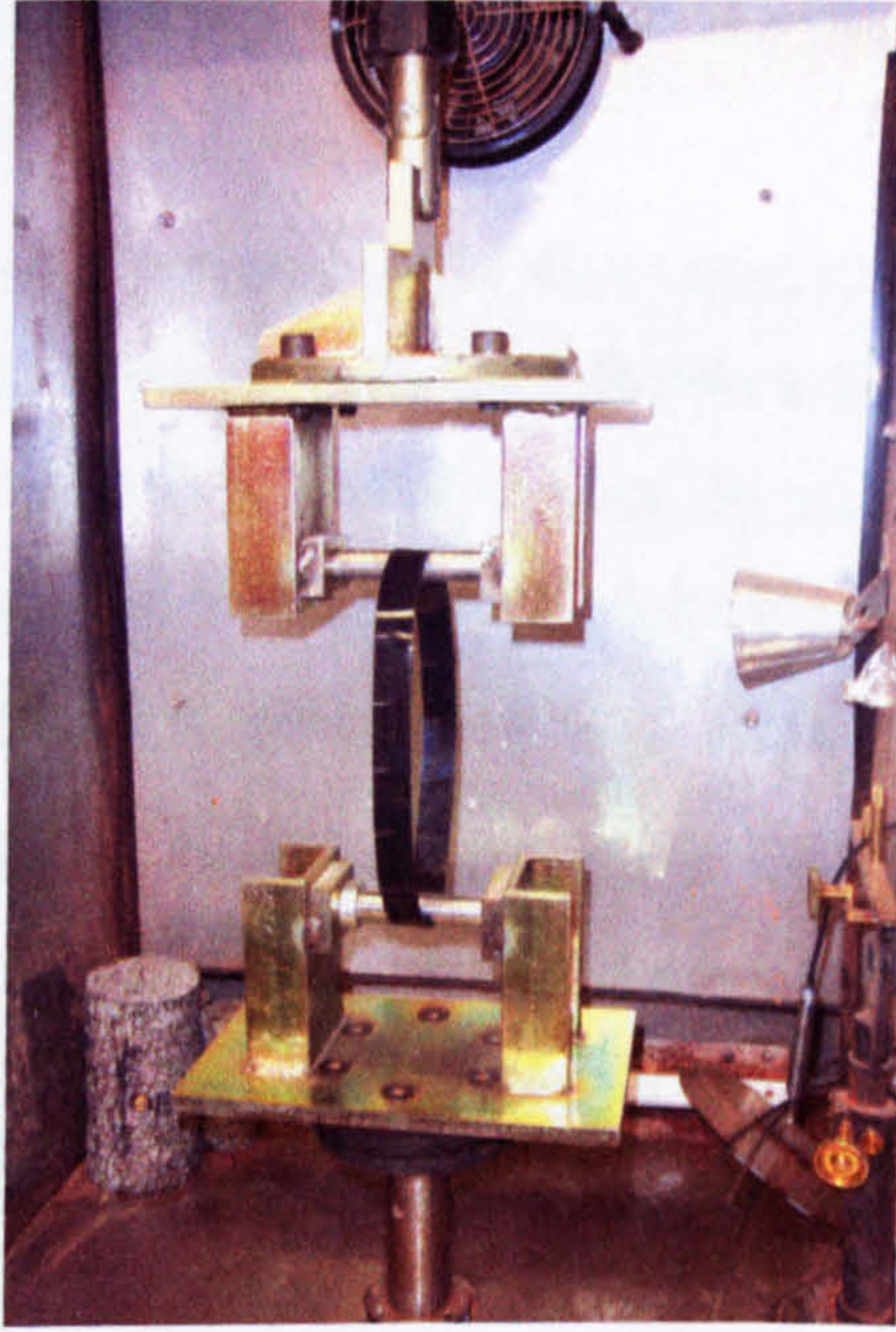
Fig 9.32 Arrangement of direct tension test (full loop).
