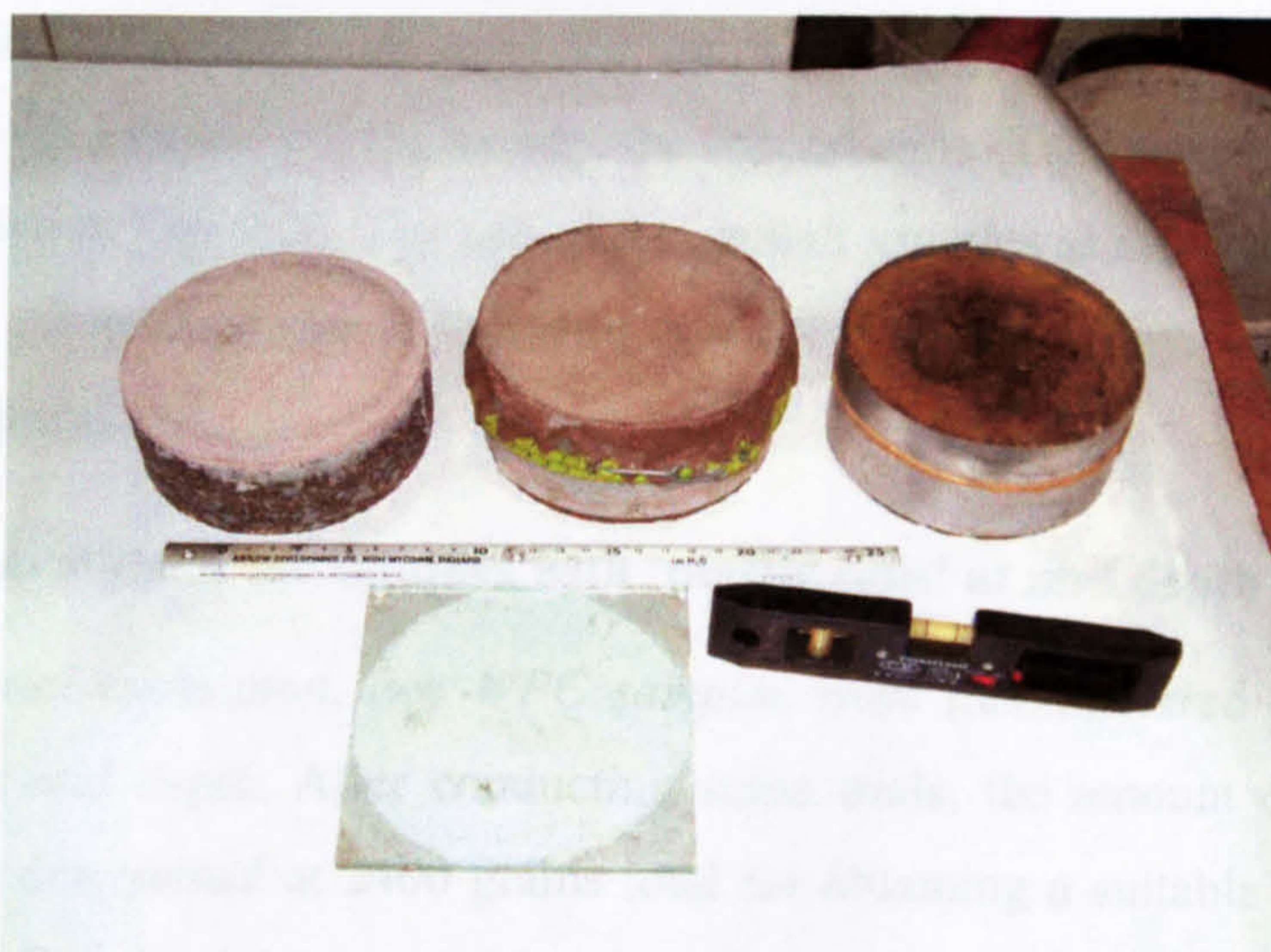
Fig. 9.19 Capping of samples to obtain upper and lower parallel flat surfaces.
