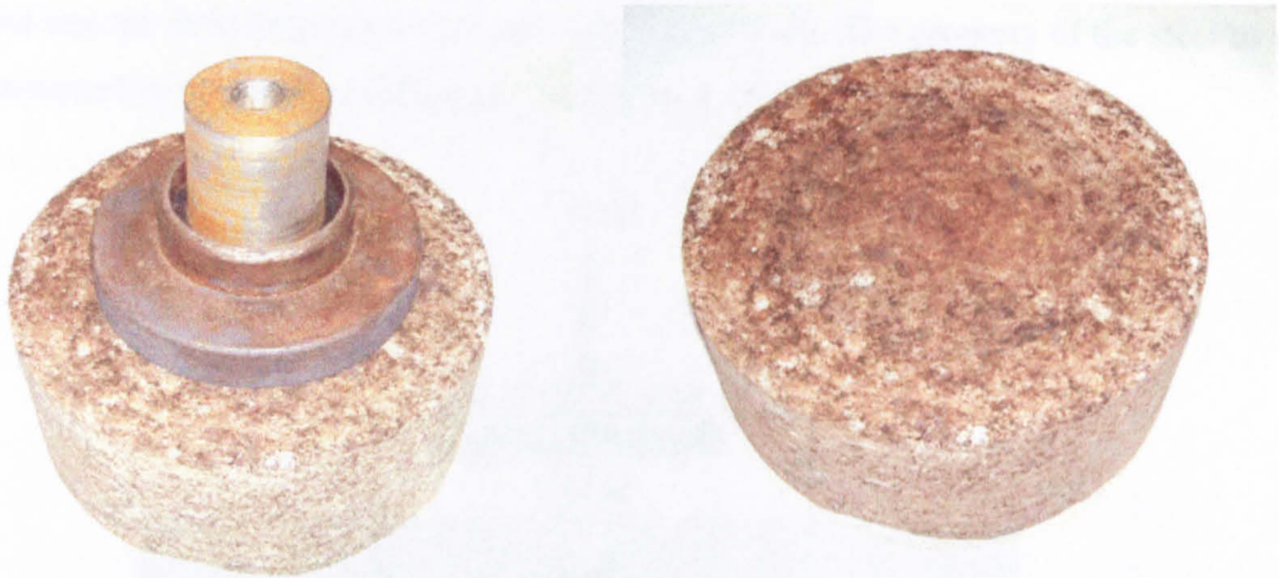
Fig. 9.29 WPC sample at the end of dynamic creep test showing very minor damage.
