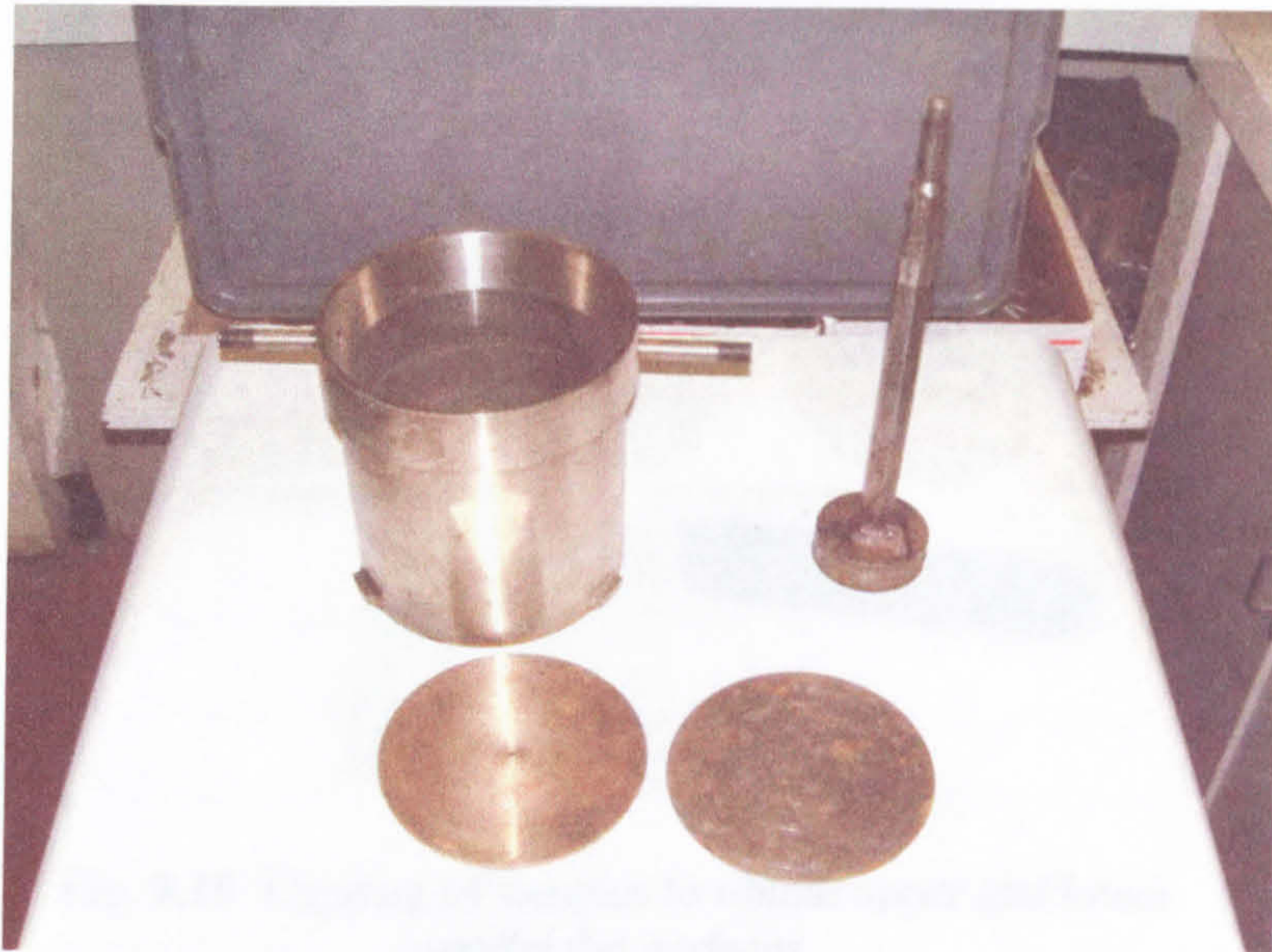
Fig. 9.18 Mould (150mm diameter) and Tamping Rod.
