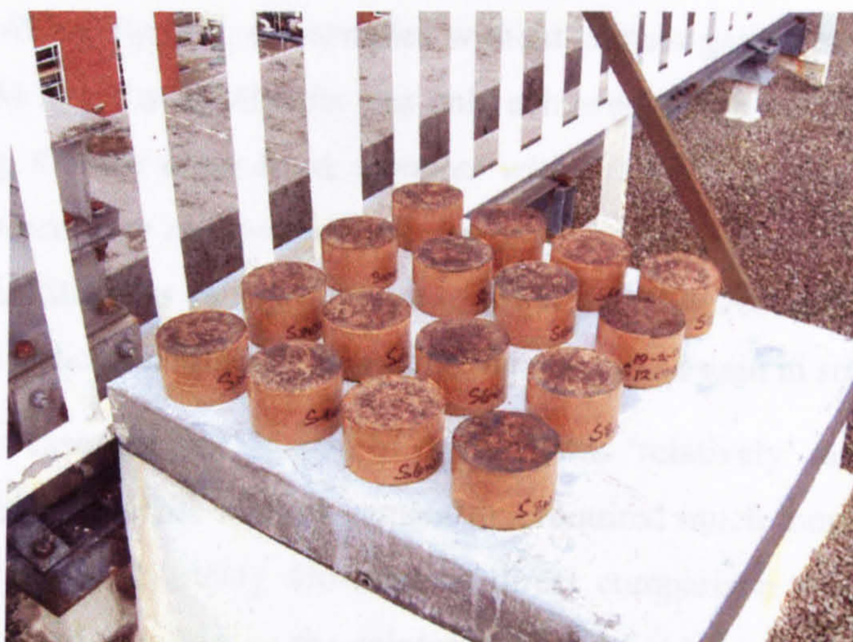
Fig. 9.6 Outdoor curing of CBEM samples.
