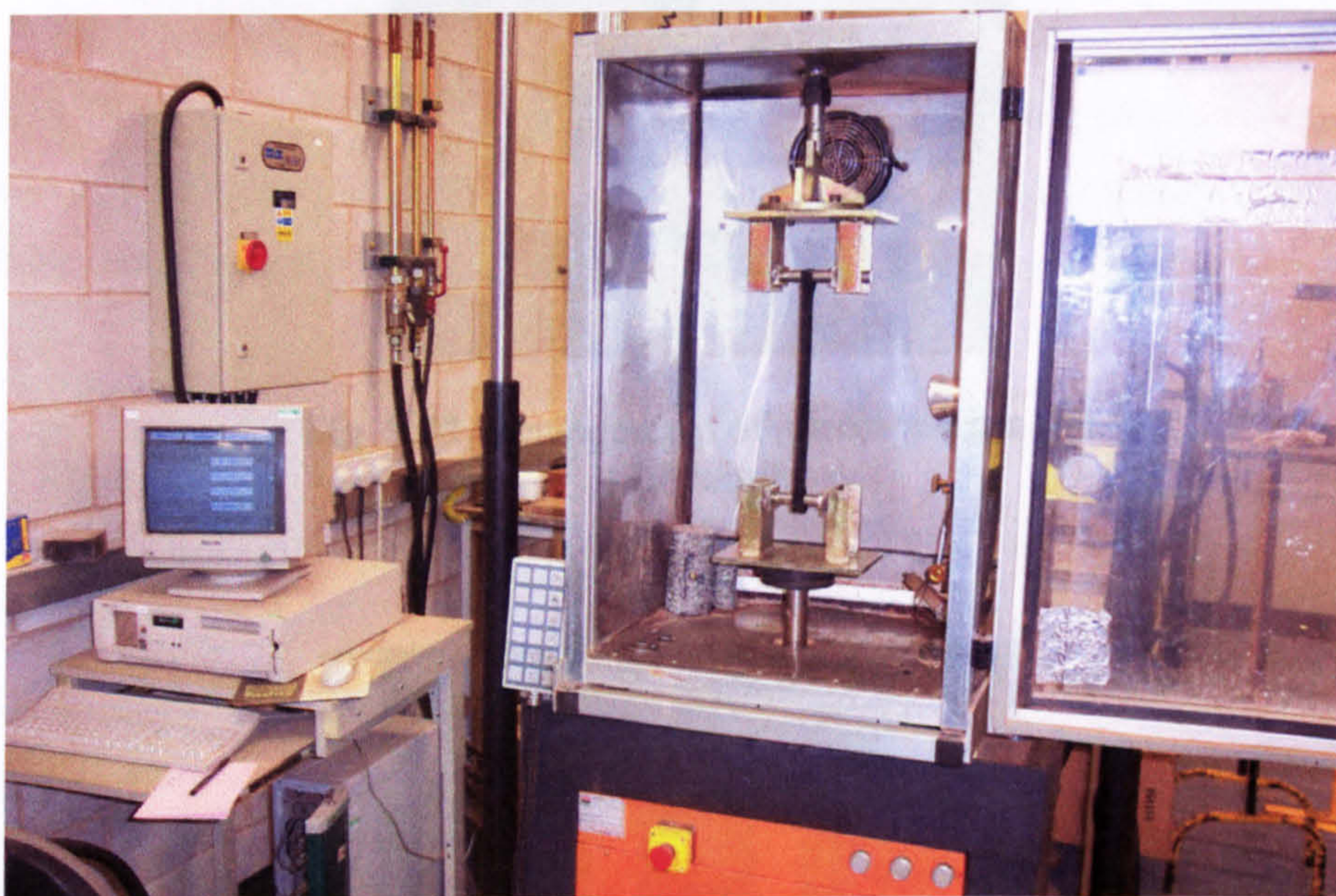
Fig. 9.31 Instron Hydraulic machine (100 kN capacity).
