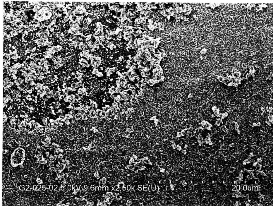
Figure 3-12: SEM image of FeS after 24 hours exposed time at 50% H 2 S, 50% CO 2 , 60°C, pH 5 [5]
