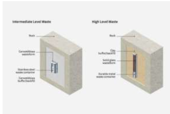
Figure 1-4: An example of a proposed multi-barrier system for a GDF.
