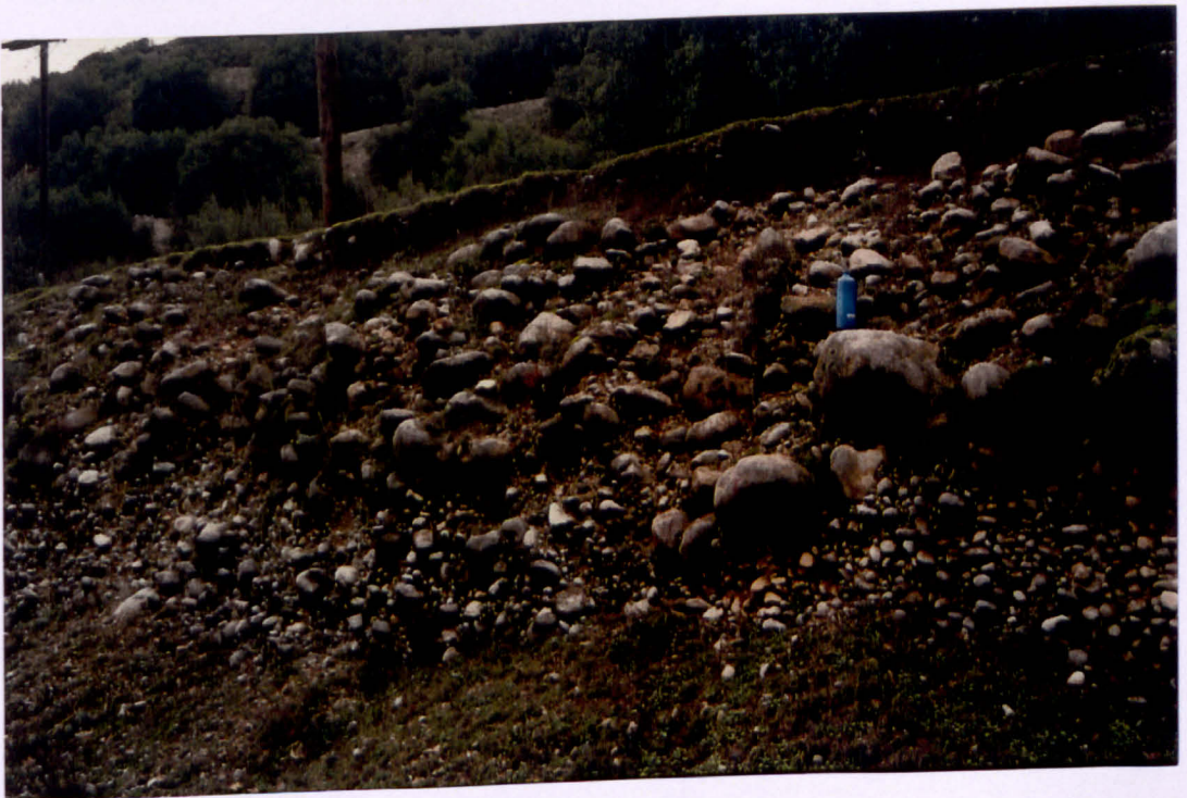
FIGURE 6.8 Photograph of the coarse grained alluvial unit at the eastern end of cross section 1 at the Aristi-Papingo Bridge Reach. The gravel matrix is not cemented and appears quite weathered. A distinctive red soils rests on top of the alluvial deposit ( cf. Woodward et al. , 1994). A water bottle is shown for scale.
